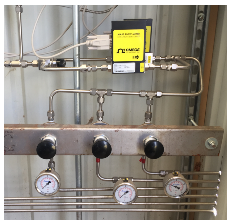
(b) Pressure regulators and Omega flowmeter used for Sierra meter verification
