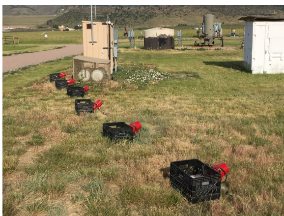
(a) Six Sierra flow meters connected in series at the CSU Methane Testing and Evaluation Center.
