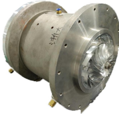
Figure 2-9: Prototype expander-compressor with an integrated electric motor. From [37].
