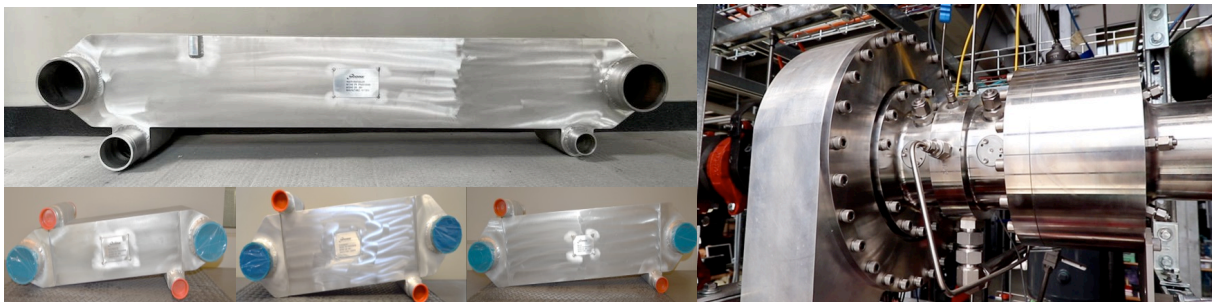
Figure 1-4: Custom fabricated heat exchangers and turbomachinery utilized in the ORVC system. Highly effective heat exchange and efficient turbomachinery help to give the technology uniquely high performance.
