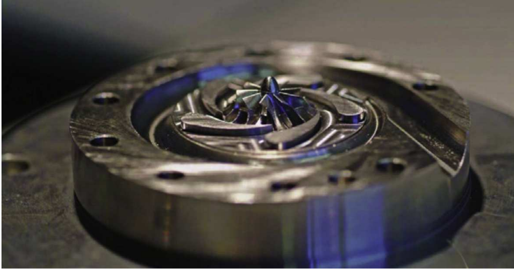
Figure 2-2: Example of a radial turbine that has been proven to be effective in ORVC applications. From [40].
