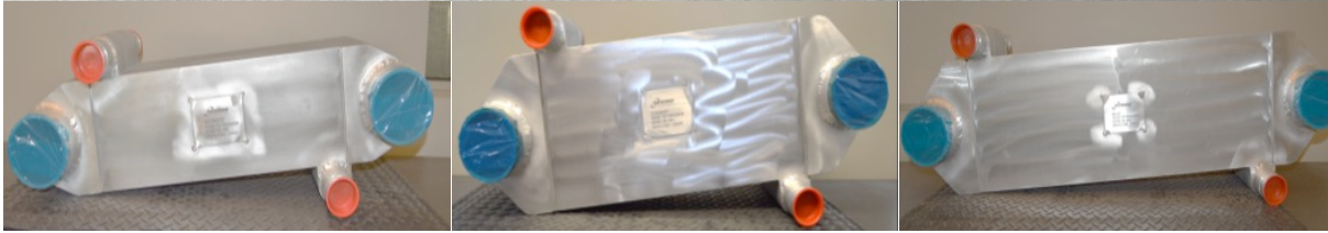
Figure 3-18: Power cycle recuperator, cross-cycle economizer, and suction line heat exchanger cores (left to right).
