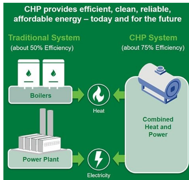
Figure 1-2: CHP offers significantly improved efficiency over traditional energy systems. Pairing thermally driven chillers with CHP systems can improve CHP utilization and efficiency. Sourced from [16].
