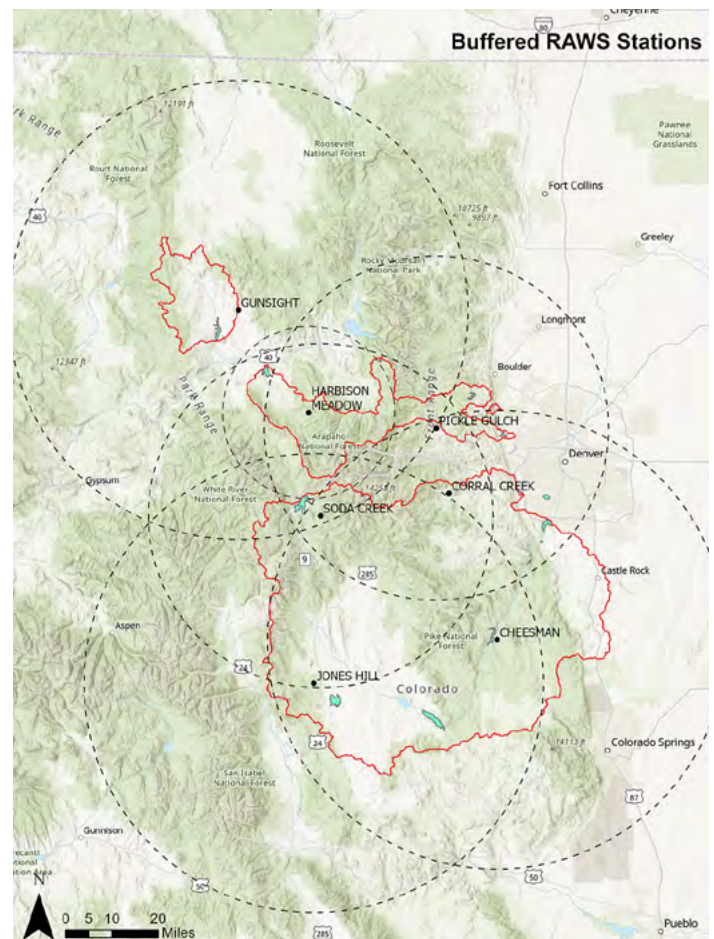
Figure 5: RAWS locations used for fire modeling with Denver Water source area in red. Dotted circles represent the spatial extent at which each station influenced fire behavior modeling.
