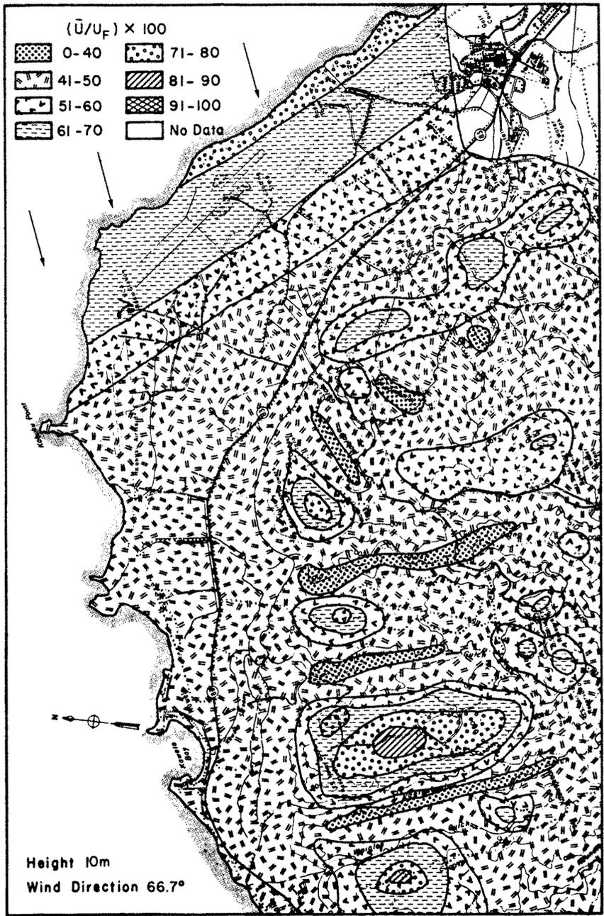
**FIGURE 3.13.** Contour Plot of Relative Velocities over the Kahuku Point Model at Equivalent 10 m Height for Wind Direction of 66.7° from North.
