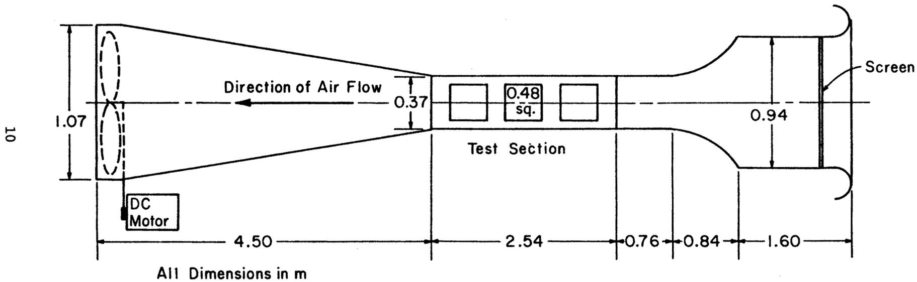
**FIGURE 2.2.** Transpiration Wind Tunnel Facility at Colorado State University.
