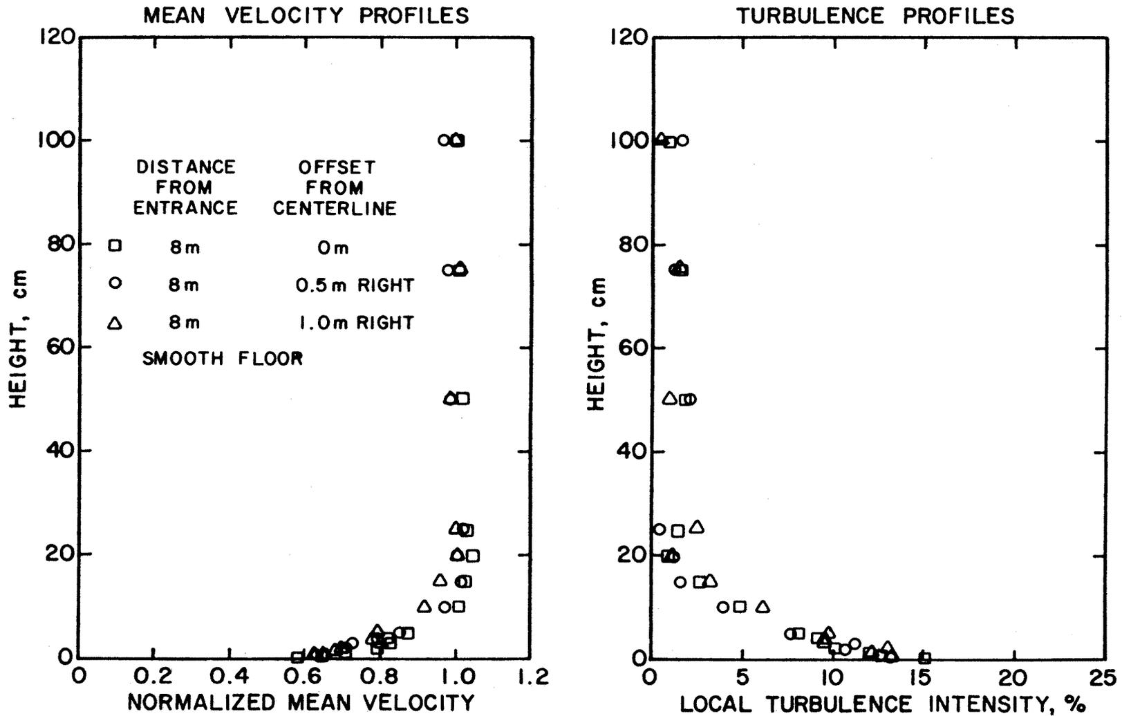
**FIGURE 3.3.** Velocity and Turbulence Intensity Profiles Measured at Spanwise Locations at 8 m Location over the Smooth Floor of EWT. Velocity Profiles were Normalized with Velocity Measured at 50 cm Height.
