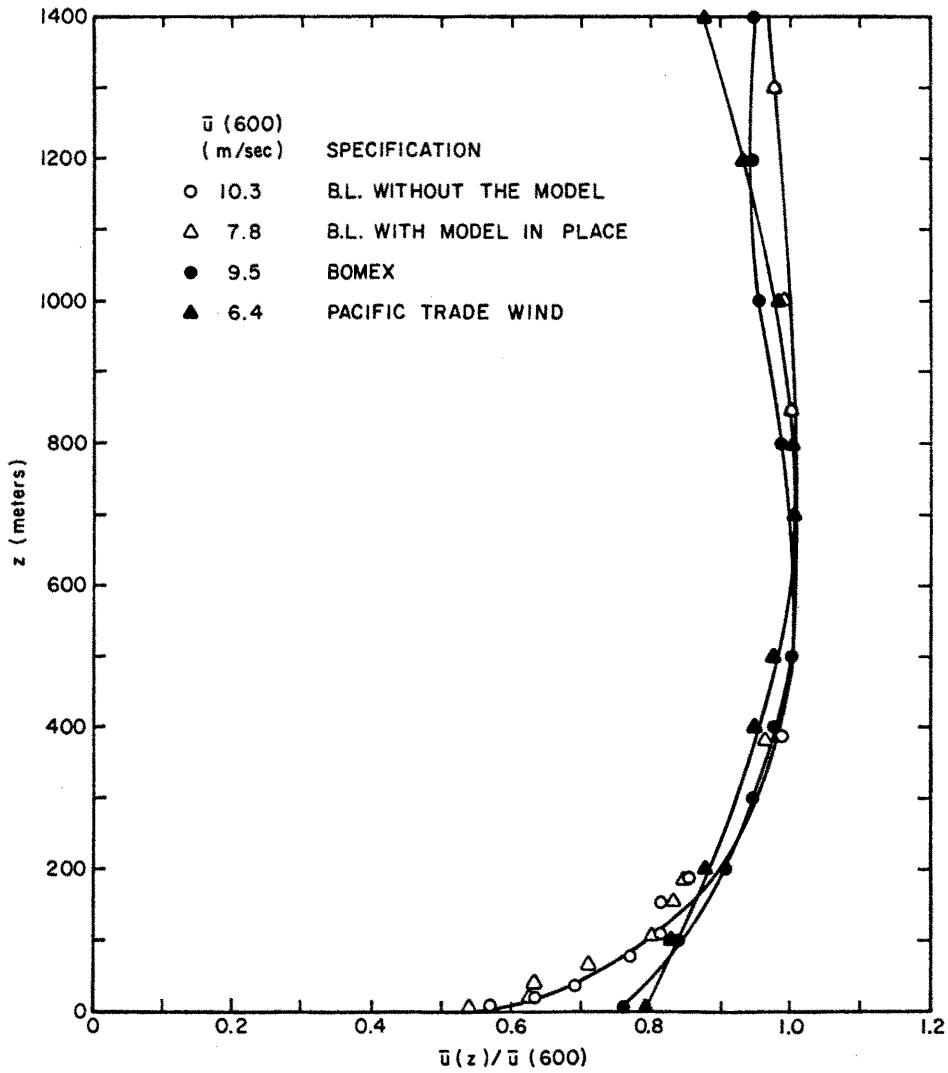
FIGURE 3.6. Comparison of Simulated Trade Wind Boundary Layer in EWT with Marine Trade Wind Boundary Layer Reported by Augstein (1979).
