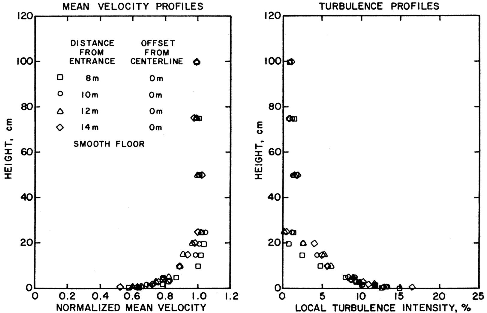
FIGURE 3.1. Velocity and Turbulence Intensity Profiles Measured Along the Centerline at 8, 10, 12 and 14 m from the Wind Tunnel Entrance over the Smooth Floor of EWT. Velocity Profiles were Normalized with Velocity Measured at 50 cm Height.
