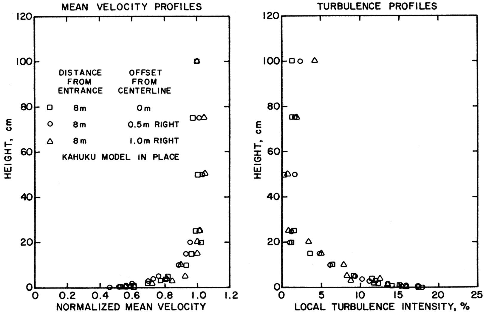
FIGURE 3.4. Velocity and Turbulence Intensity Profiles Measured Upstream of the Kahuku Model at 8 m Location. Velocity Profiles were Normalized with Velocity Measured at 50 cm Height.
