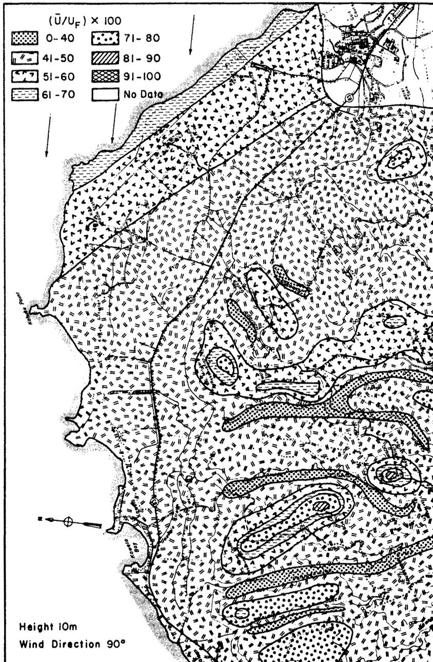
**FIGURE 3.15.** Contour Plot of Relative Velocities over the Kahuku Point Model at Equivalent 10 m Height for Wind Direction of 90° from North.
