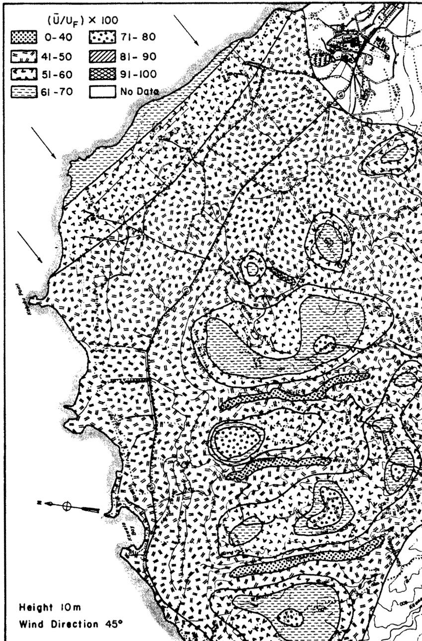
FIGURE 3.11. Contour Plot of Relative Velocities over the Kahuku Point Model at Equivalent 10 m Height for Wind Direction of 45° from North.
