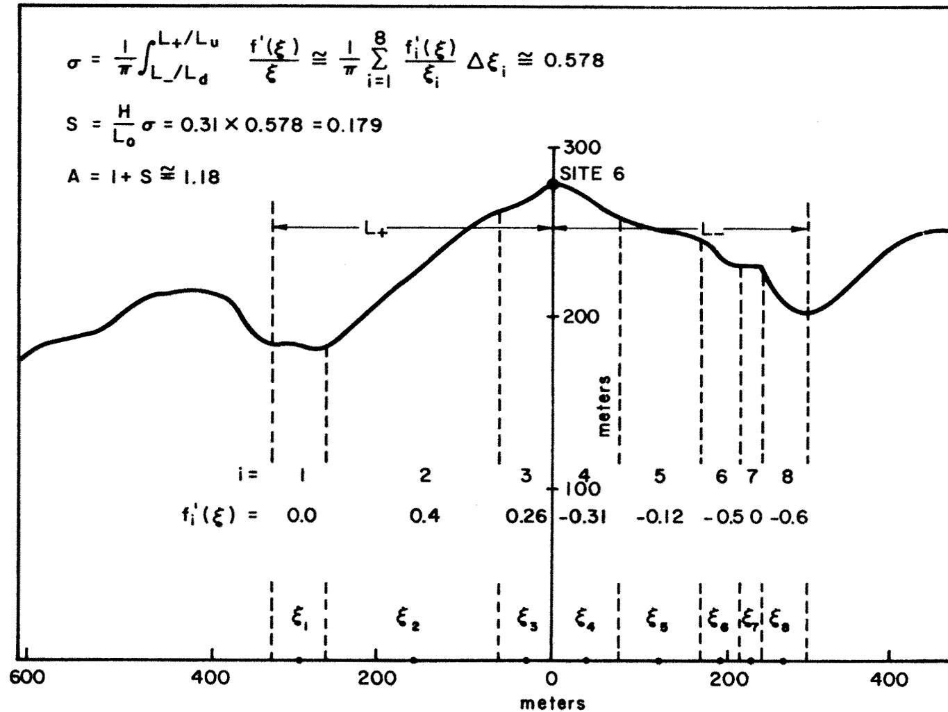
FIGURE 5.6. Demonstration for Definition of  $L_+$  and  $L_-$ , and Approximation Scheme for Evaluating Equation (5.19) in Hunt's Analytical Technique.
