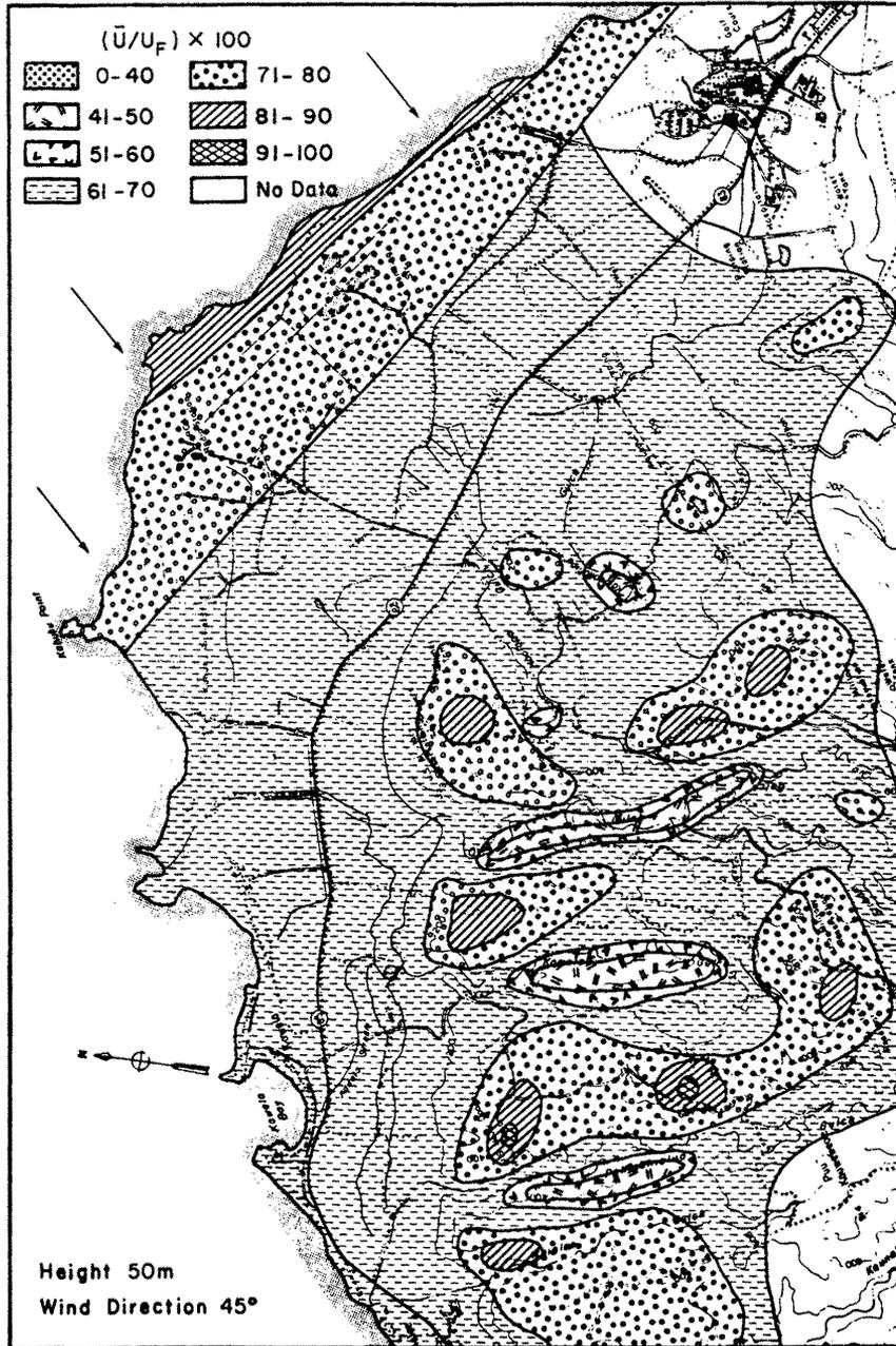
**FIGURE 3.12.** Contour Plot of Relative Velocities over the Kahuku Point Model at Equivalent 50 m Height for Wind Direction of 45° from North.
