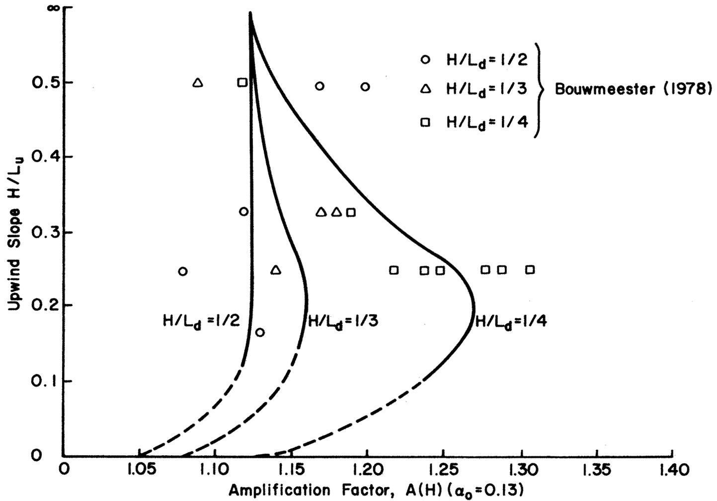
FIGURE 5.2. Dependency of Crest-amplification Factor on Upwind Slope for  $\alpha_0 = 0.13$ .
