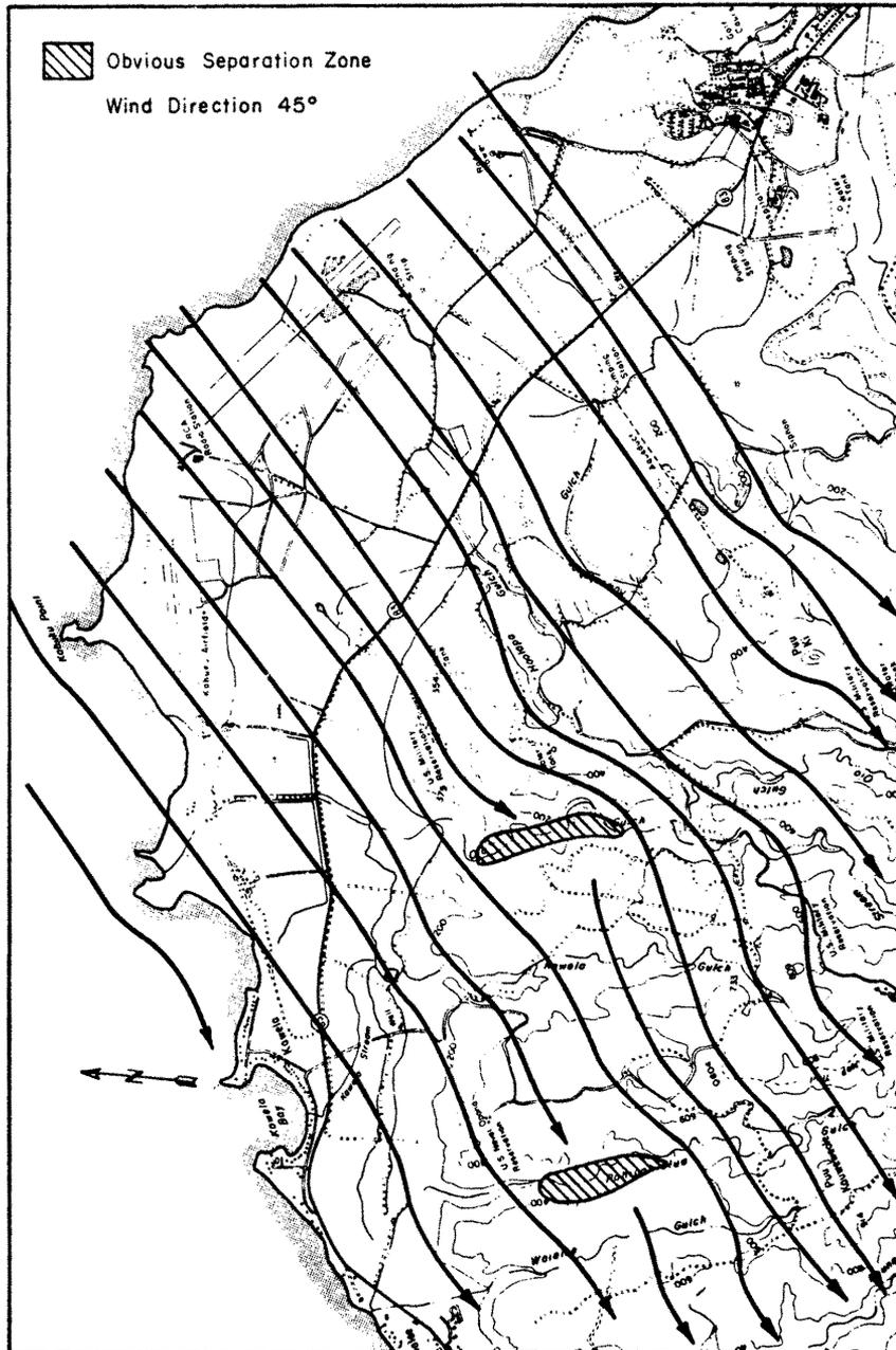
**FIGURE 3.8.** Flow Pattern Over the Kahuku Point Model for Approaching Wind Direction of 45° from North.
