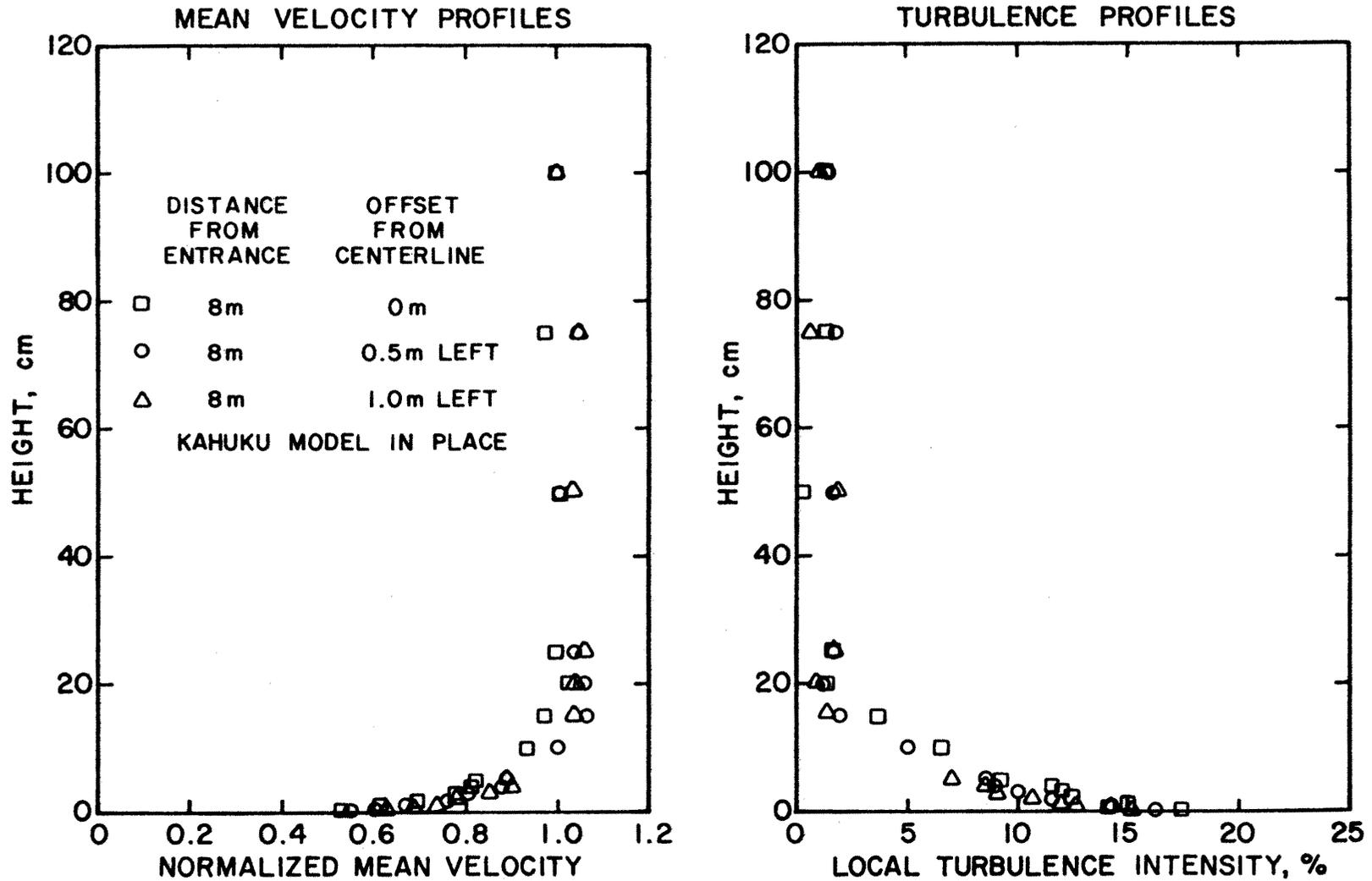
**FIGURE 3.5.** Velocity and Turbulence Intensity Profiles Measured Upstream of the Kahuku Model at 8 m Location. Velocity Profiles were Normalized with Velocity Measured at 50 cm Height.
