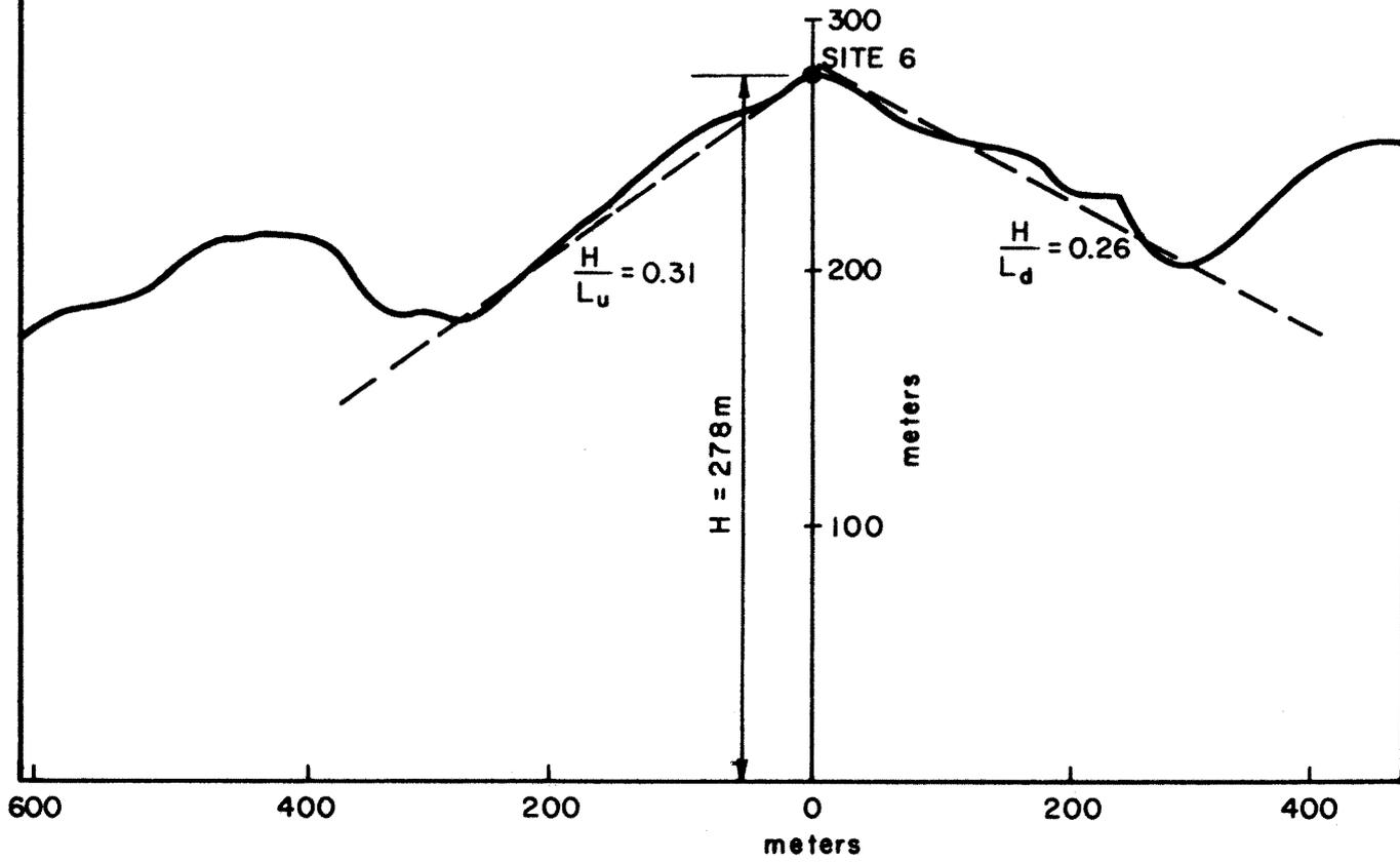
FIGURE 5.3. Vertical contour for Site 6 and Its Surrounding Area and Characteristic Parameters Used in Bouwmeester's Speed-up Prediction Technique.
