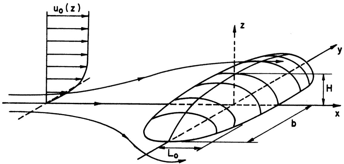
FIGURE 5.5. Coordinates and Notations for Potential Flow Over an Ellipsoidal Hill
