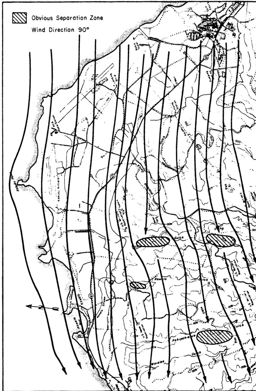
FIGURE 3.10. Flow Pattern over the Kahuku Point Model for Approaching Wind Direction of 90° from North.
