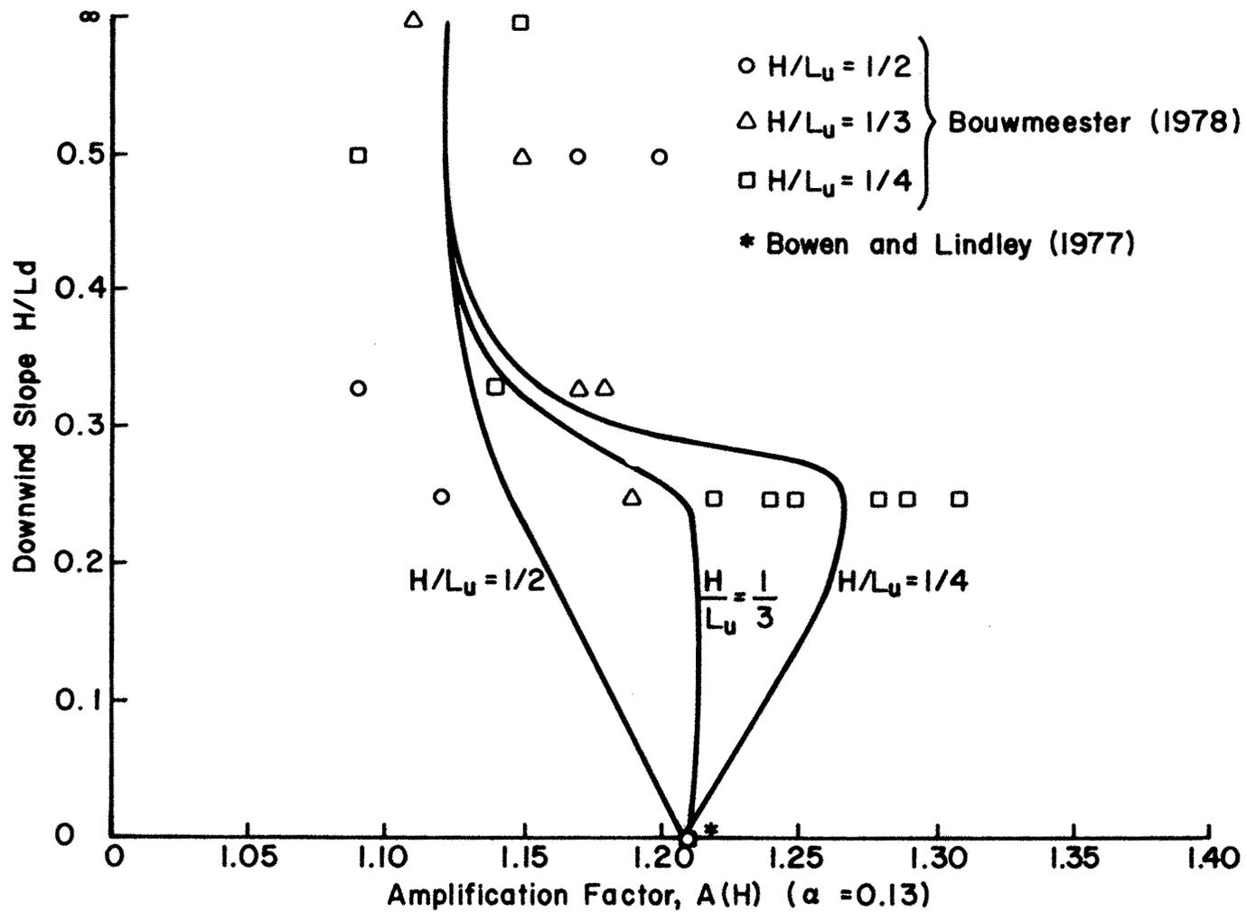
FIGURE 5.1. Dependency of Crest-amplification Factor on Downwind Slope for  $\alpha_0 = 0.13$ .
