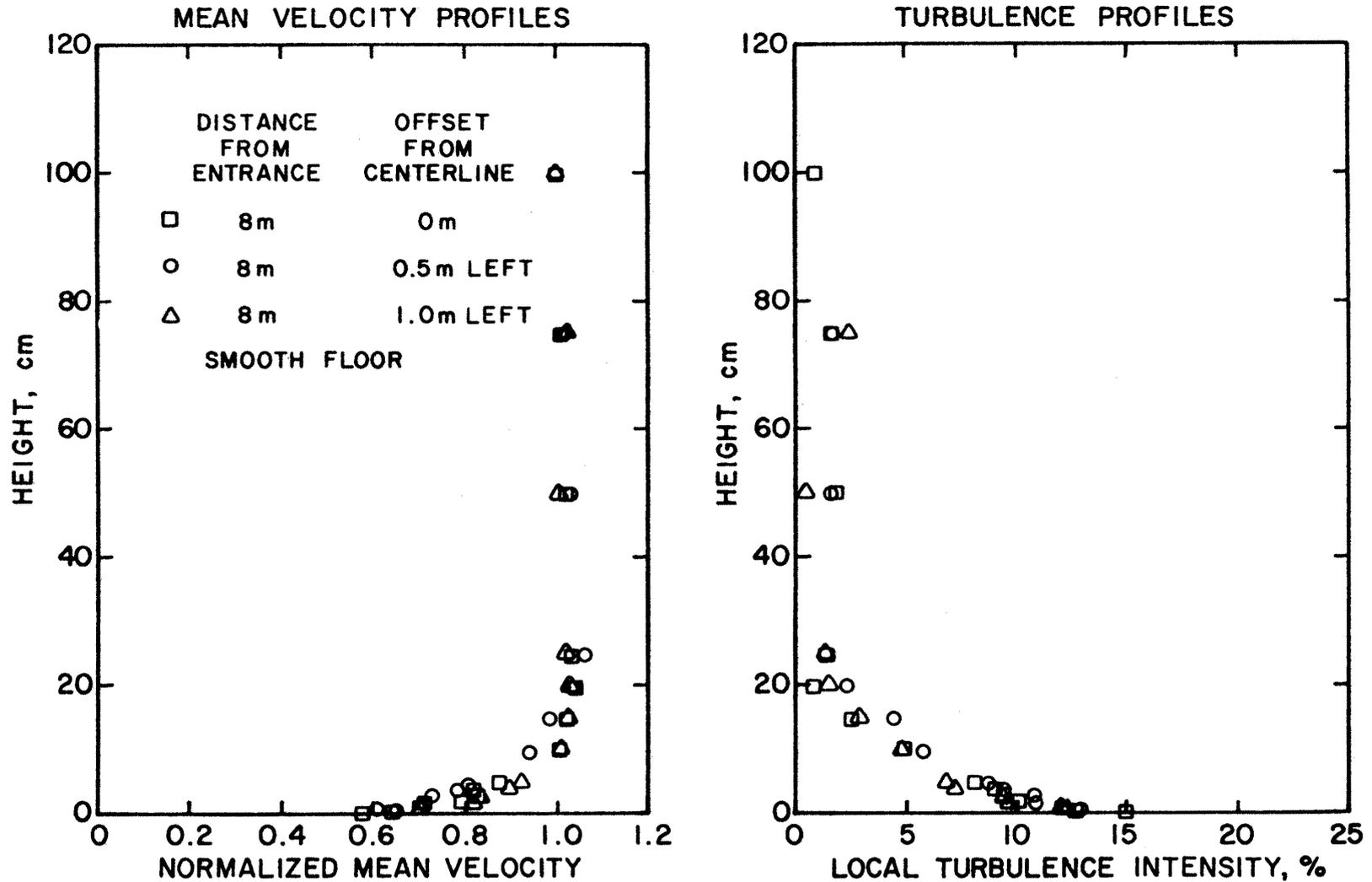
**FIGURE 3.2.** Velocity and Turbulence Intensity Profiles Measured at Spanwise Locations at 8 m Location over the Smooth Floor of EWT. Velocity Profiles were Normalized with Velocity Measured at 50 cm Height.
