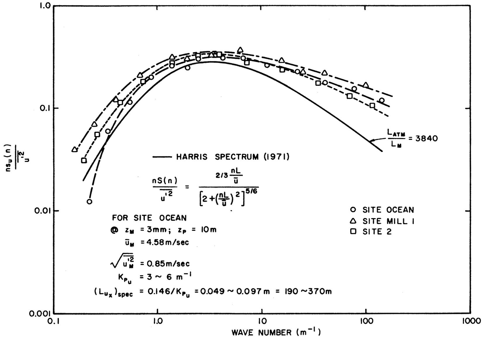
FIGURE 3.7. Comparison of Longitudinal Power Spectra Measured at Three Sites Over the Kahuku Model with Harris Spectrum at 10 m Height.
