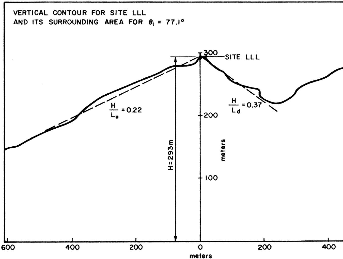
**FIGURE 5.4.** Vertical Contour for Site LLL and Its Surrounding Area and Characteristic Parameters Used in Bouwmeester's Speed-up Prediction Technique.
