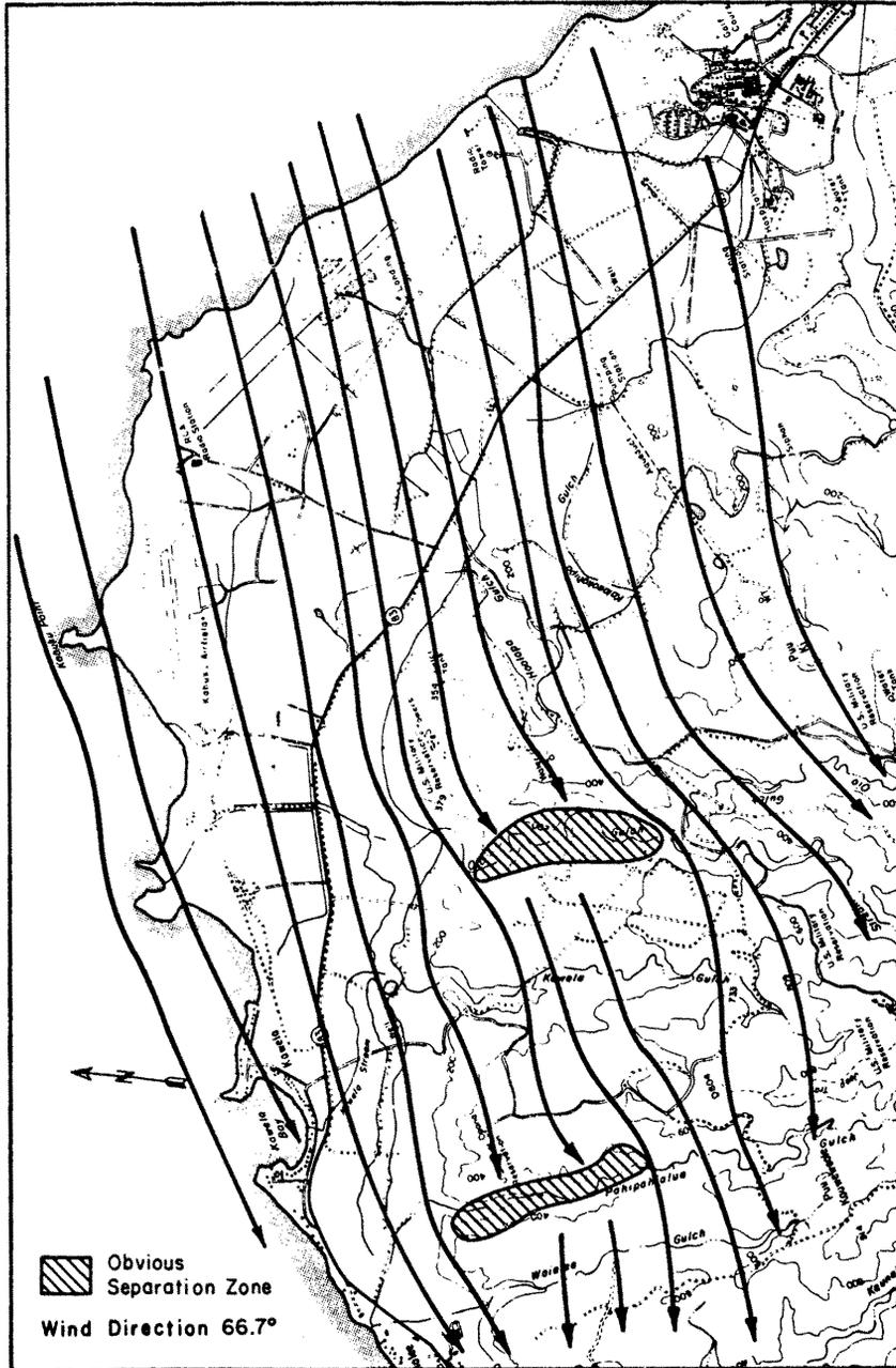
FIGURE 3.9. Flow Pattern over the Kahuku Point Model for Approaching Wind Direction of 66.7° from North.
