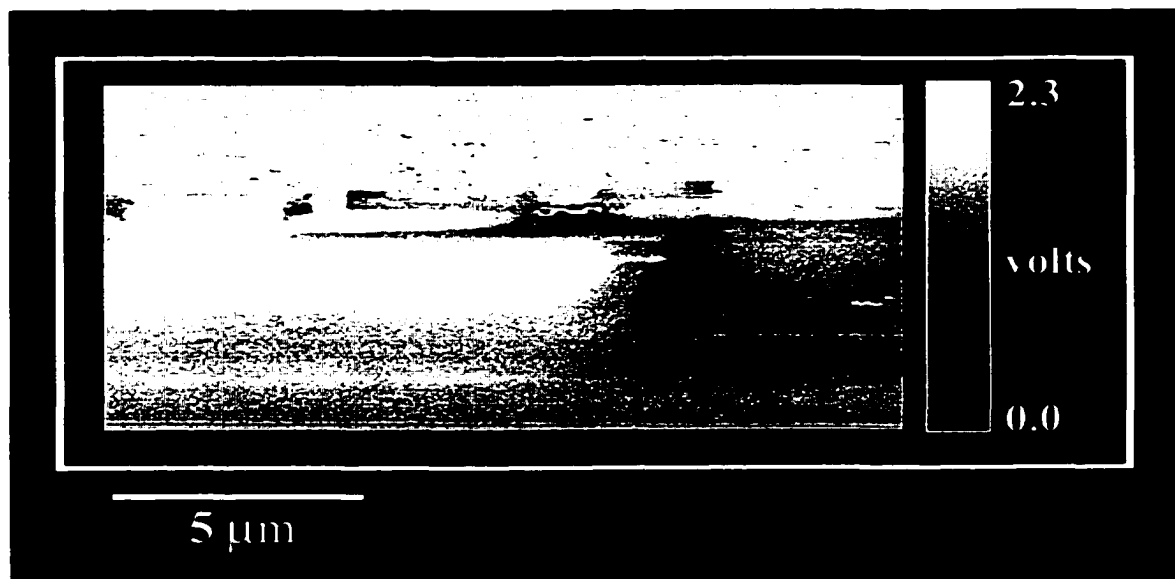
Figure 5.10: Scanning capacitance (dC/dV) cross-section image of a Hewlett Packard bipolar transistor.
