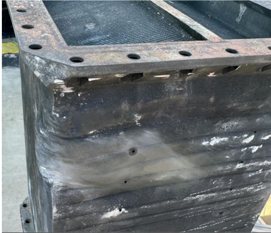
Figure 19: Bulging of the Initial Oxiperator
