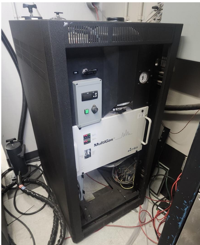
Figure 14: MKS Instruments, Inc Model No. 2030 FTIR Gas Analyzer
