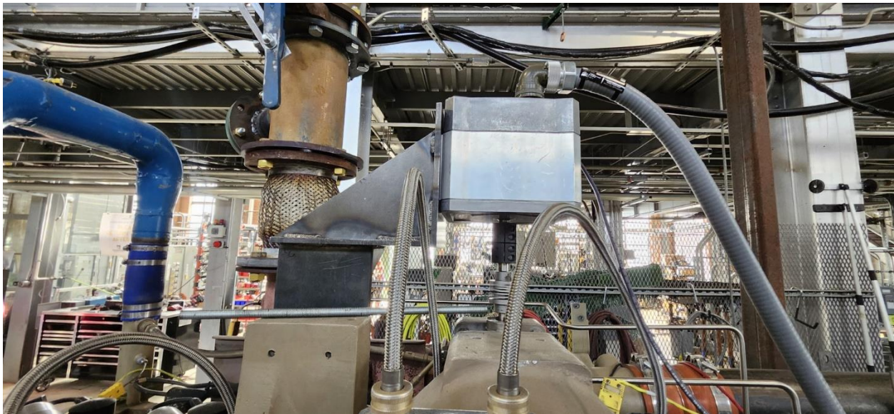
Figure 8: ActuCOM R8 speed governor mounted on the top of the engine using new steel bracket.
