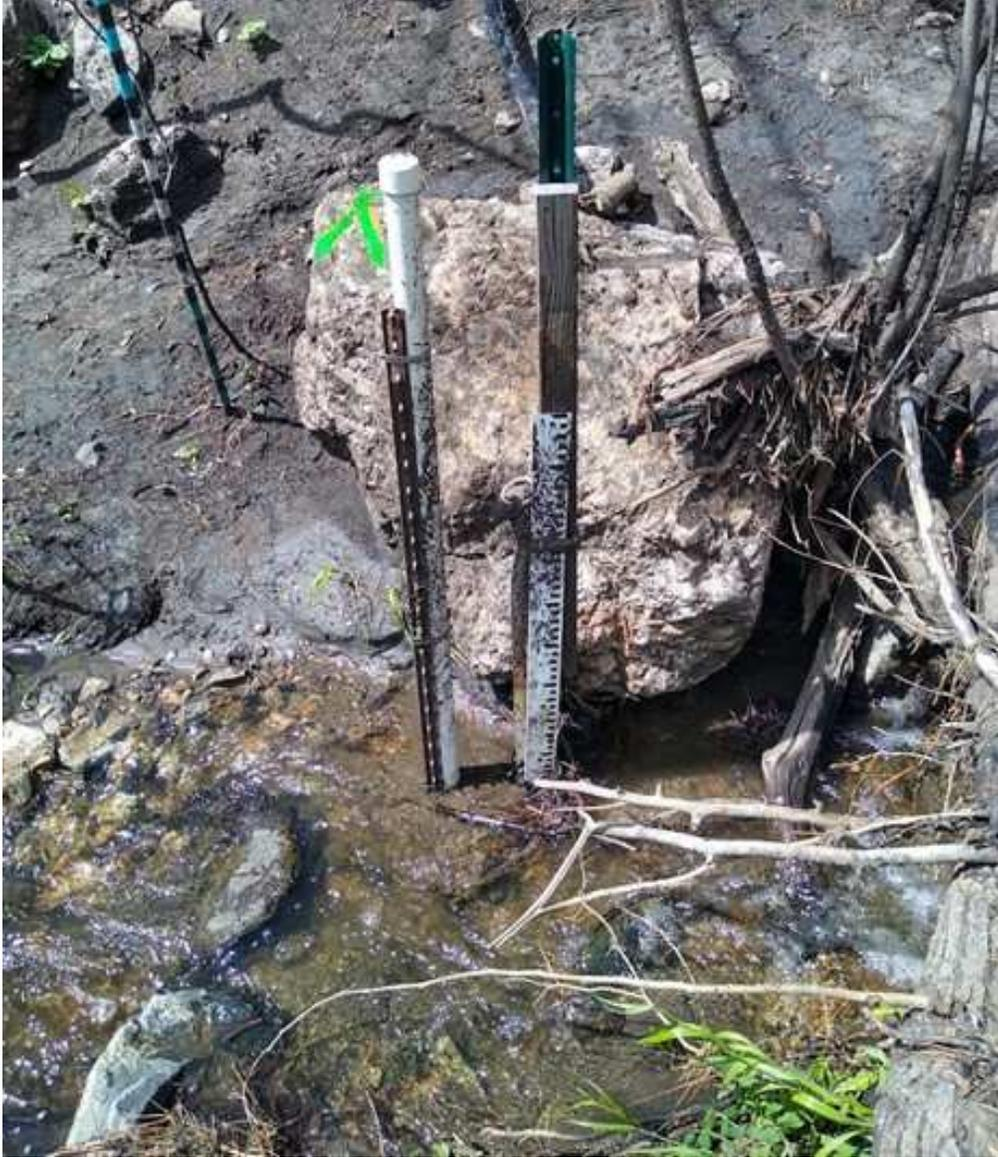
**Figure 14.** Geomorphic change observed at SBI. After a large rainstorm on June 25, 2021, the stream sensor was covered with ~10cm of fine sediment. The debris marking the upper levels of the staff plate imply that a large amount of sediment was moved downstream. Photo courtesy of Stephanie Kampf.
