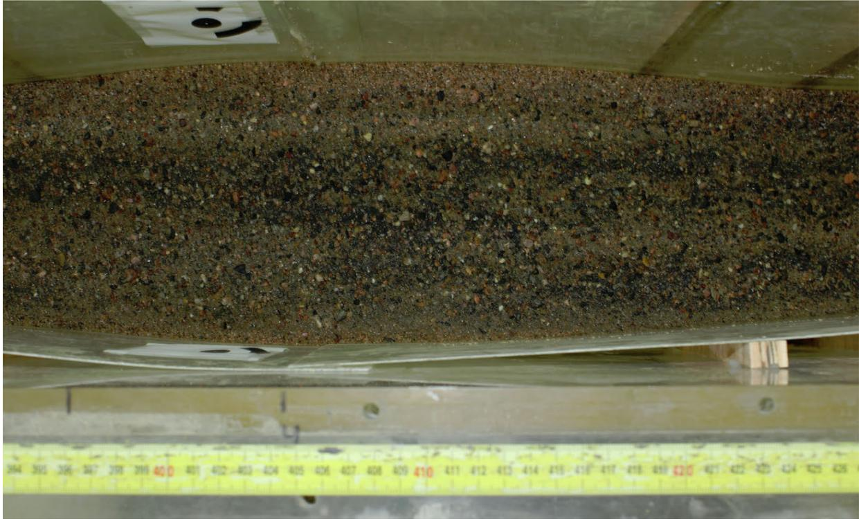
**Figure 50:** Return to an armored condition after 711 minutes (Run 5).
