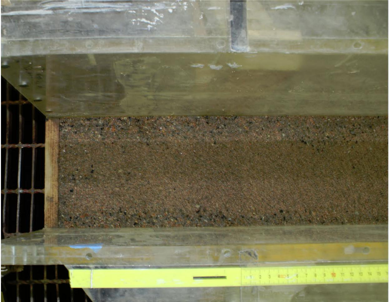
**Figure 49:** Sediment Pulse after reaching the flume outlet at 86 minutes.
