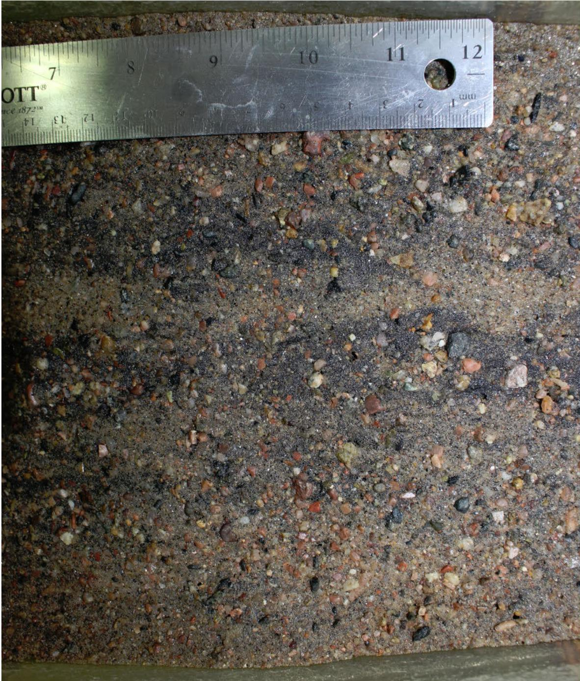
**Figure 45:** Surface material at riffle location after Run 2 (24.13 hours).
