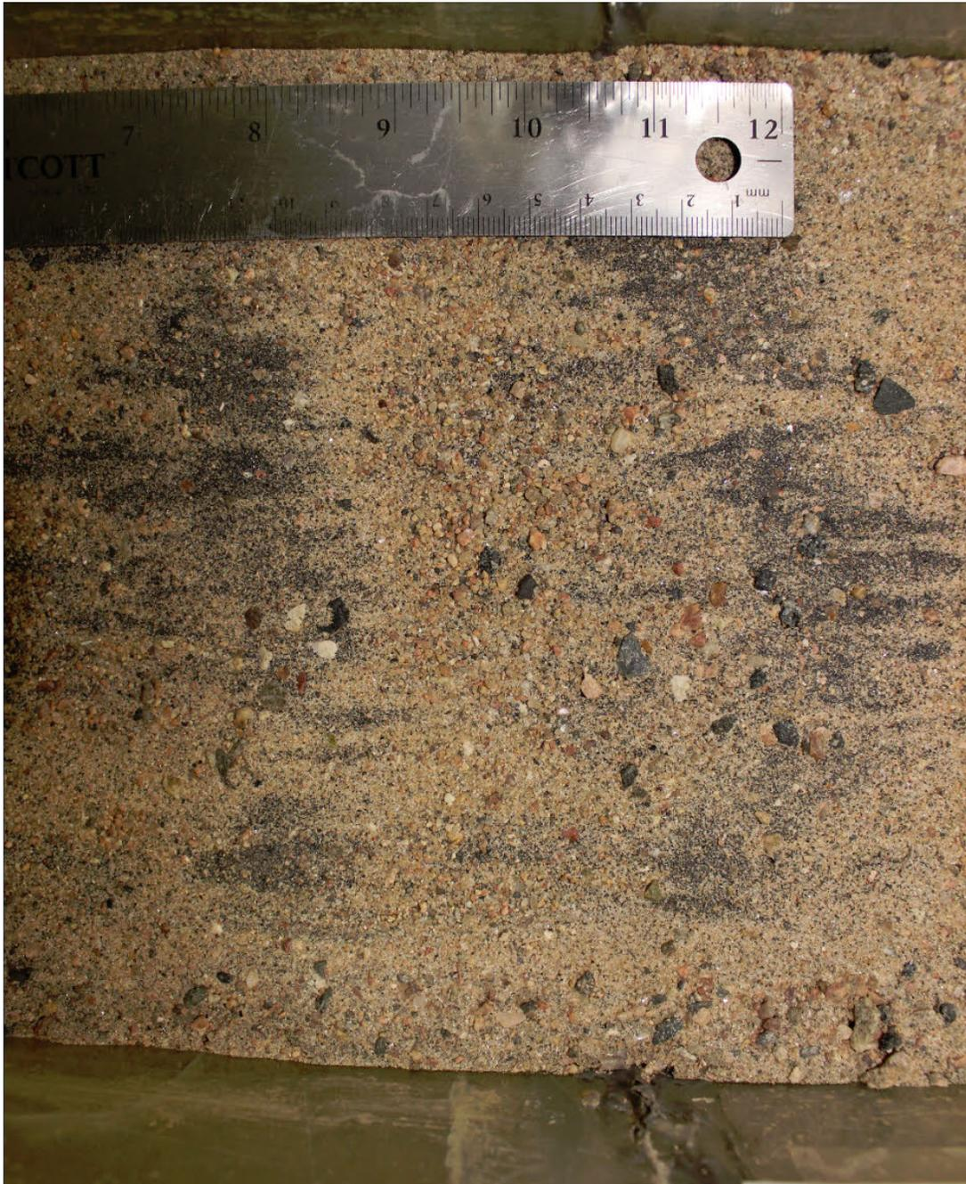
**Figure 44:** Surface material at riffle location after Run 1 (13 hours).
