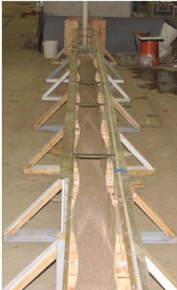
**Figure 12:** Image of the flume with sinusoidal walls installed, inducing width variability.
