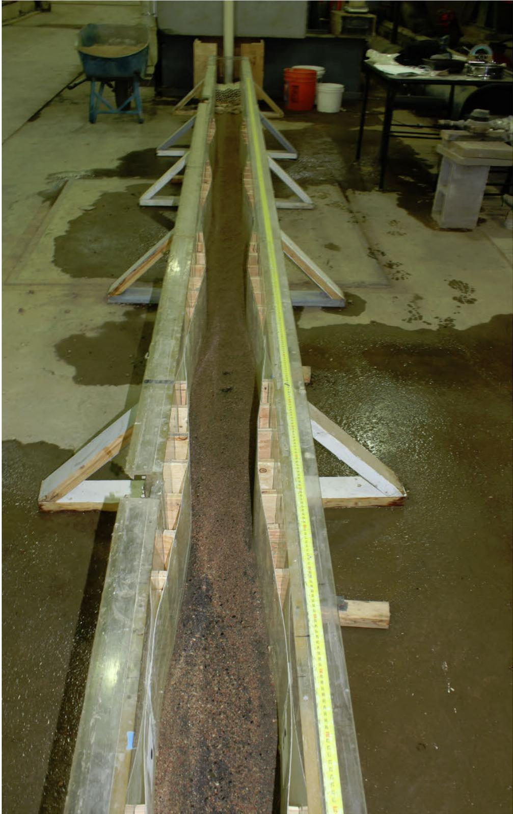
**Figure 47:** Location of sediment pulse after 27 minute (Run 5).
