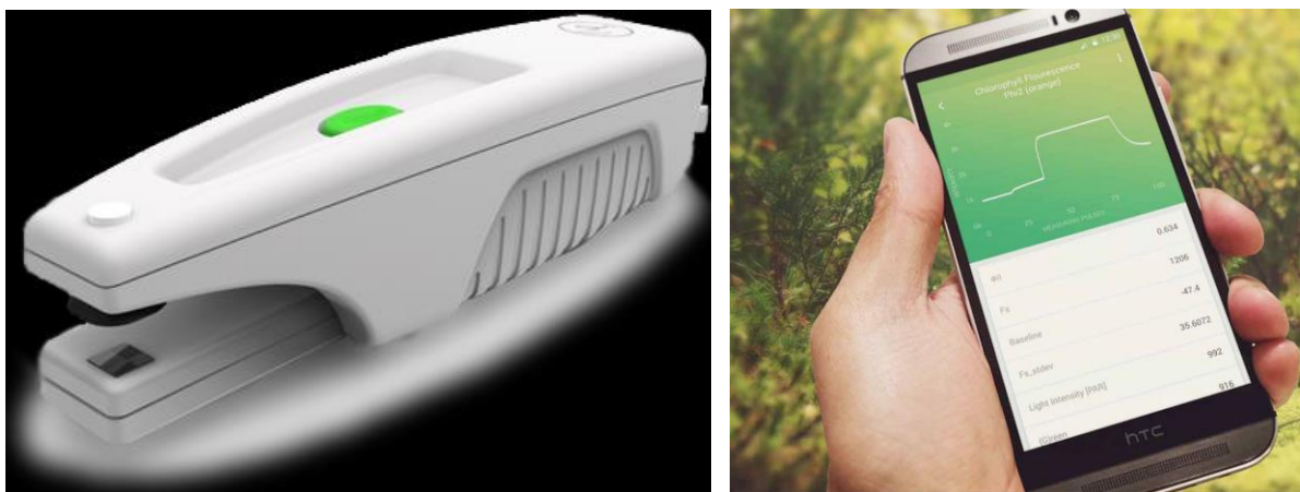
Figure 5.3. Photographs of PhotosynQ (left) and mobile phone application to view results in the field (Images from http://photosynq.org/ ).
