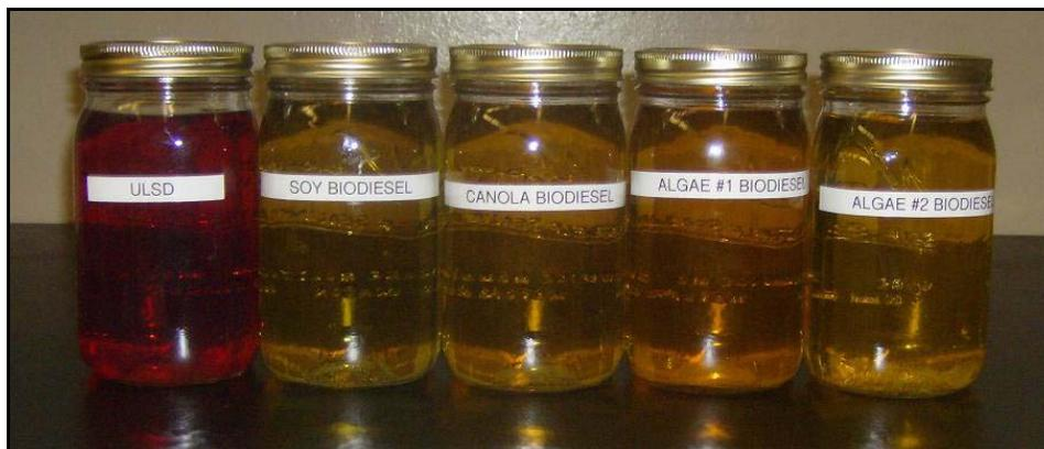
Figure 4.1 - Samples of red diesel and B100 biodiesels used in tests.
