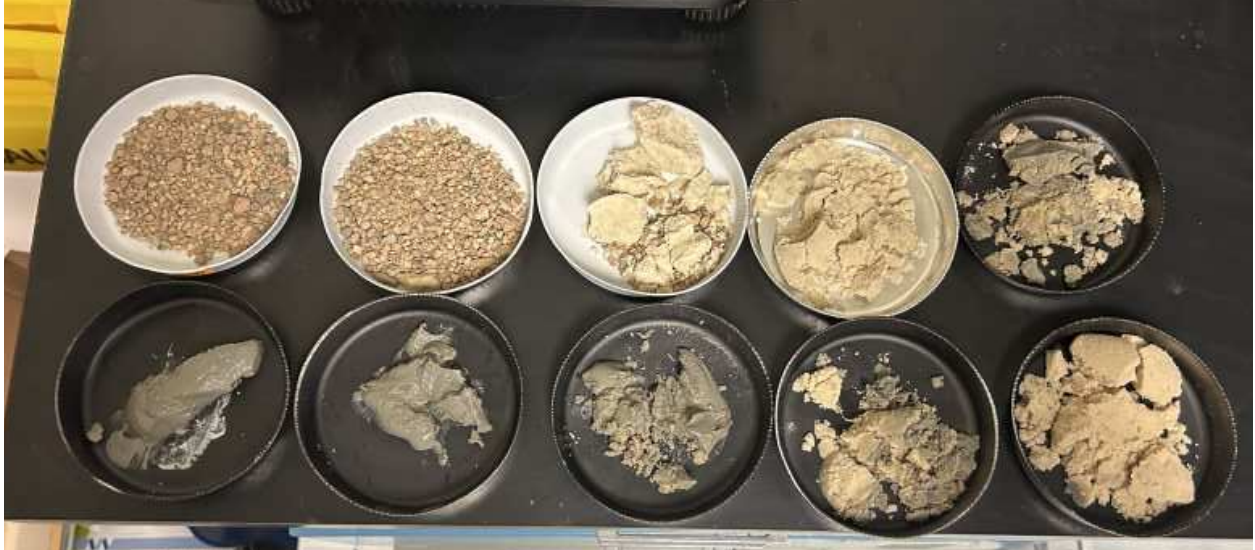
Figure B.5 - Sample collection series from various depths of deconstructed tailings column.
