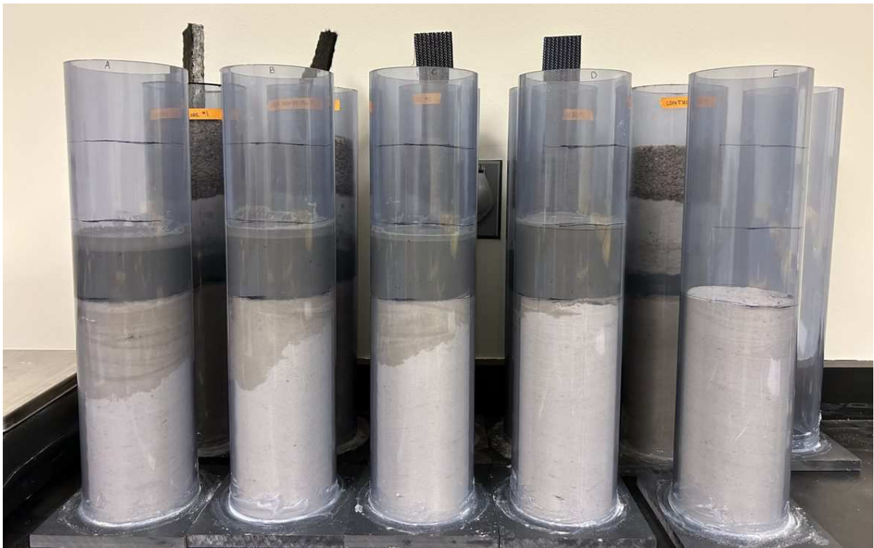
Figure B.4 - Setting up the tailings column experiments and visually observing immediate drain down into the lower fines layer.
