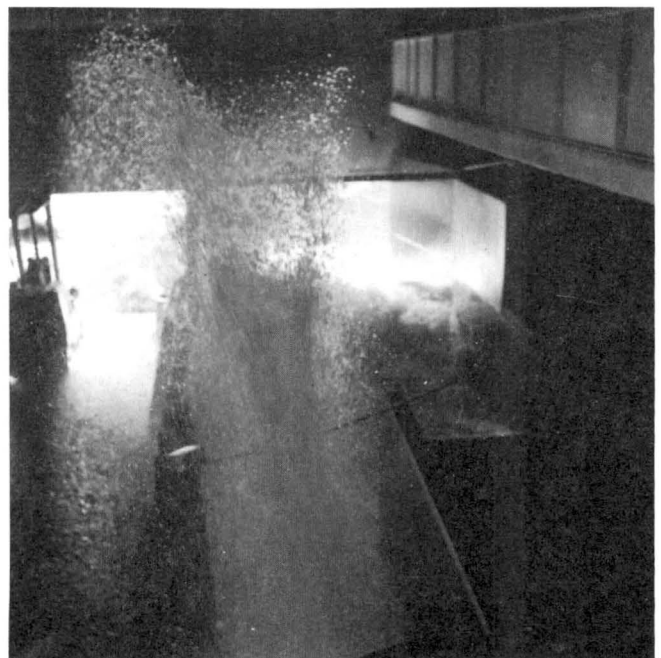
Figure 85. Jet beyond the gate structure. Gate is open 11.2 ft, head is 440 ft and gap width is 0.8 in.
