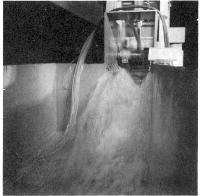
Figure 90. The effectiveness of the side-wall deflectors is seen for the condition of figure 89.
