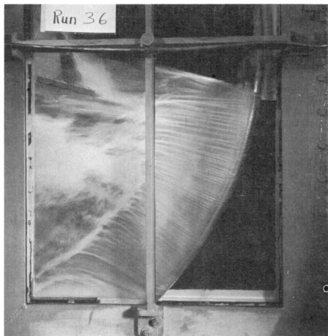
Figure 58. Retracted condition for gate at 0 ft, gap width of 0.863 in. and H_a of 430 ft with top jet arrestor.
