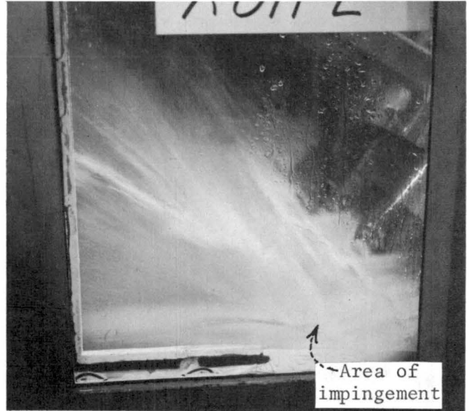
Figure 39. Normal operation with triangular side-seal recess for 2.15-ft gate opening and 270-ft head.
