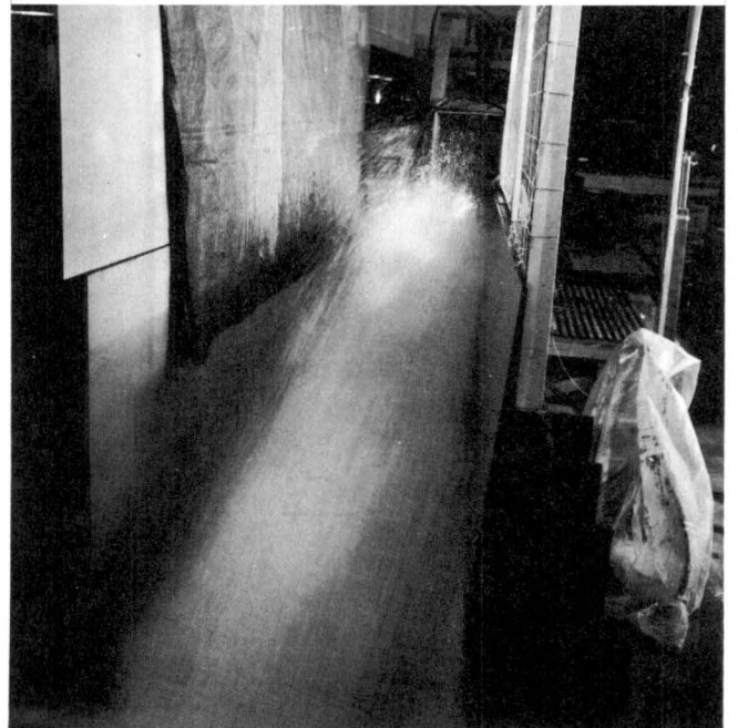
Figure 102. Gate is open 8 ft and H_a is 400 ft. Note the trajectories of the droplet spray.
