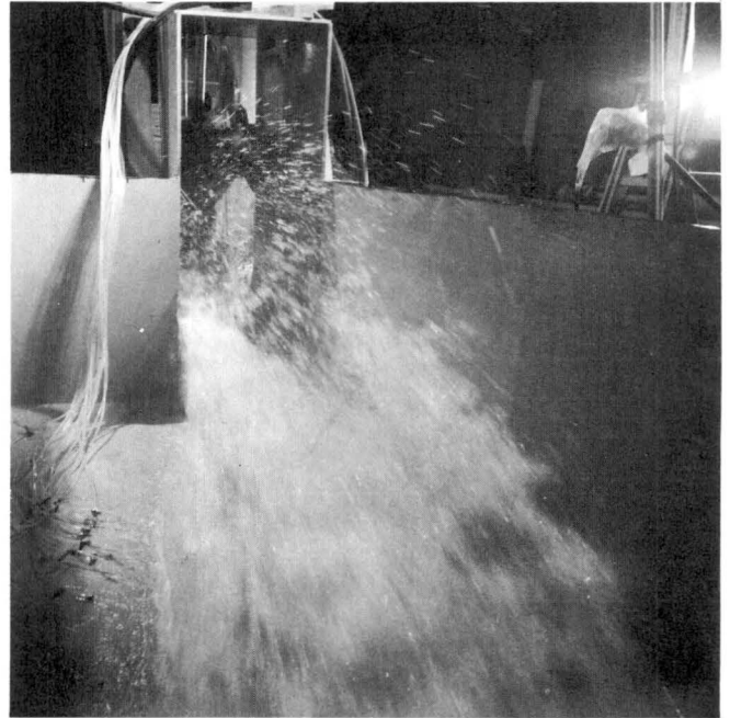
Figure 101. The spray resulting from the rooster tails extends above the chute walls.
