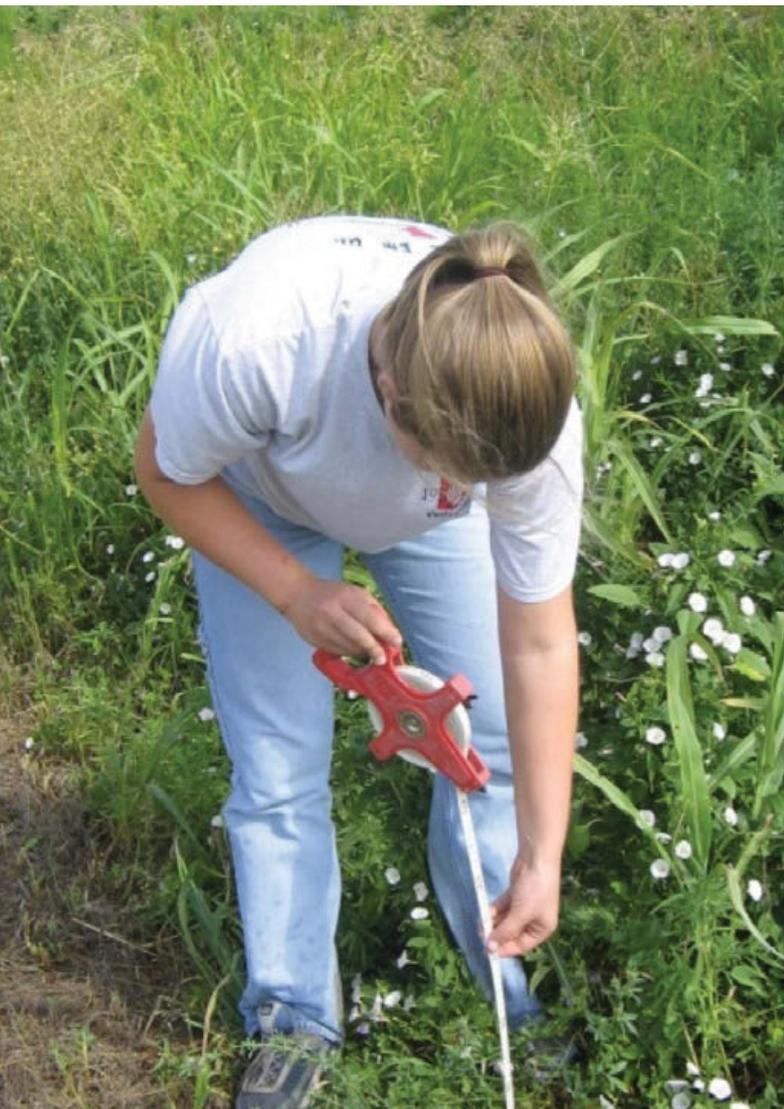
**Figure 32.** CSU field technician measuring depth to water table in well on Field DS12 using an open-spool tape, 2005
