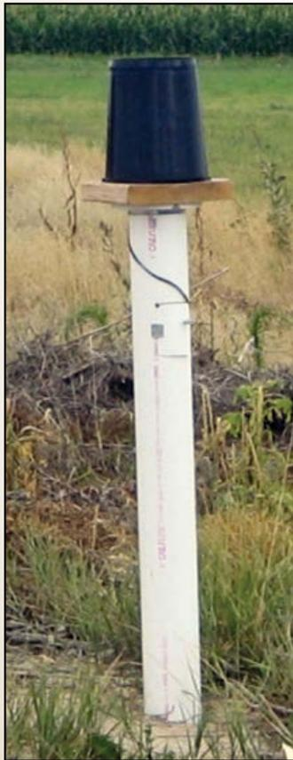
**Figure 20.** HOBO® rain gauge in Field US17E in 2008
