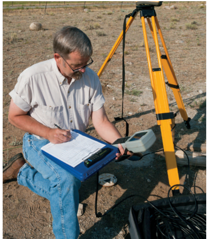
CSU Civil and Environmental Engineering Professor Timothy Gates collects data with a multi-probe at a well on a ranch near Chalk Creek.
