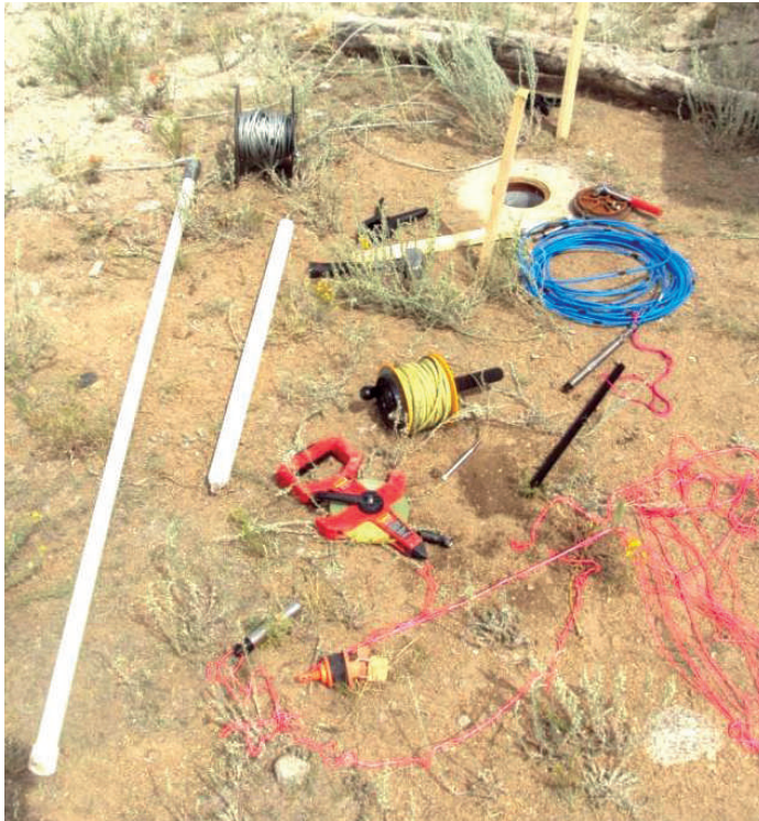
Figure 2.17. Slug test equipment and well monitoring accessories (from left, clockwise to center): 6 ft solid slug and suspension cable reel, 3 ft bailer, hammer, clamp, stakes, well cover, socket wrench, vented data logger cable (blue), Level Troll® 700 data logger (silver w/ black tip), black iron weight, transducer suspension string (pink), transducer, j-plug cap, steel tape, and electric water-level indicator.
