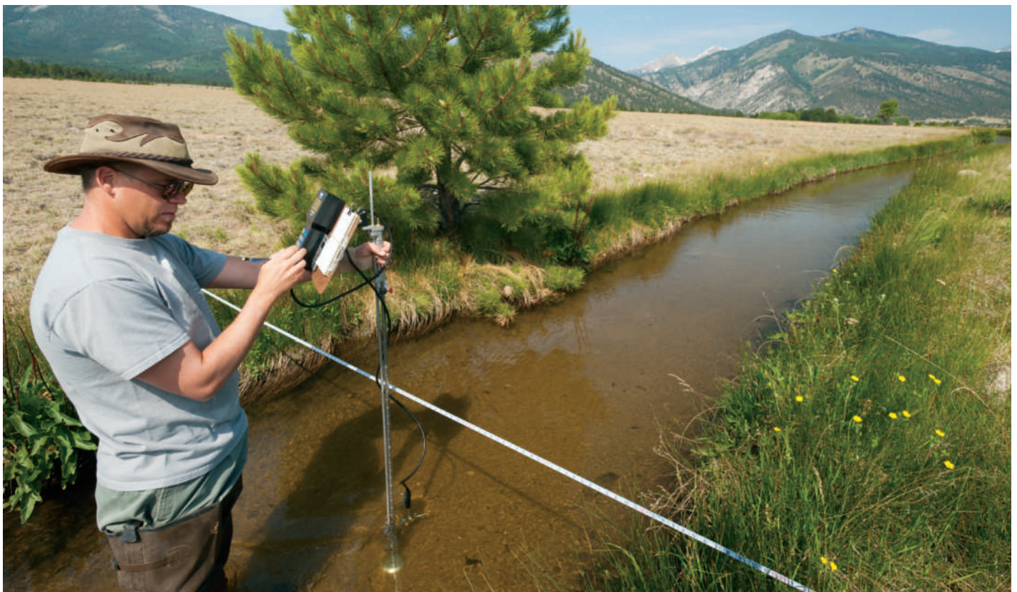
CSU Civil and Environmental Engineering graduate student Greg Steed uses an acoustic Doppler current profiler to survey Cottonwood Canal in the upper Arkansas River Basin, Buena Vista.
