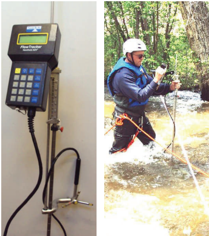
Figure 2.11. (Left) ADV device consisting of the control interface unit and the three-pronged flow measuring transceiver, mounted on a standard USGS wading rod with offset bracket. (Right) Surface water flow measurements with the ADV on the South Arkansas River in June 2011.
