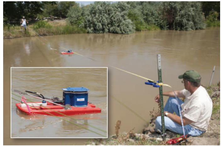
Figure 3.12. Using an ADCP to measure flow rate through a cross section on the Fort Lyon Canal in July 2011, with a close-up of the ADCP shown.
