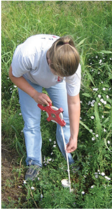
Figure 3.13. Measuring depth to water table in a groundwater monitoring well in the DSR using an open-spool tape.
