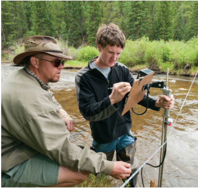
CSU Civil and Environmental Engineering graduate student Greg Steed and undergraduate student Justin Kattnig use an acoustic Doppler current profiler.
