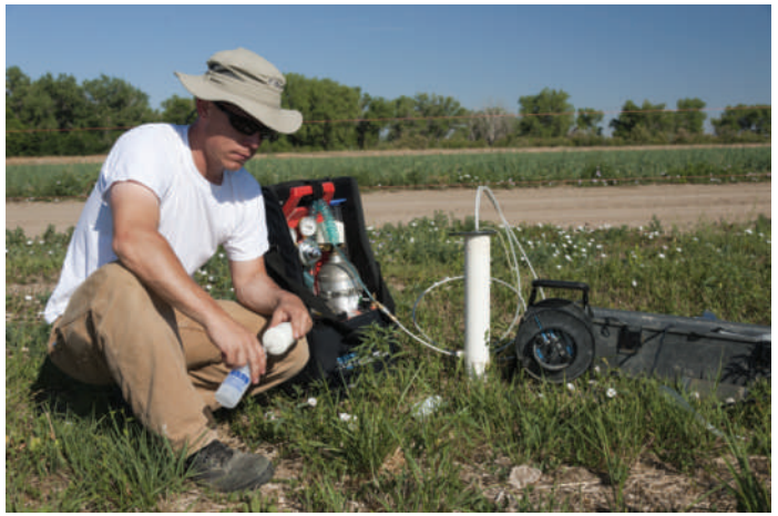
Figure 3.14. Collecting a filtered water quality sample from a groundwater monitoring well in the USR using a low-flow bladder pump.
