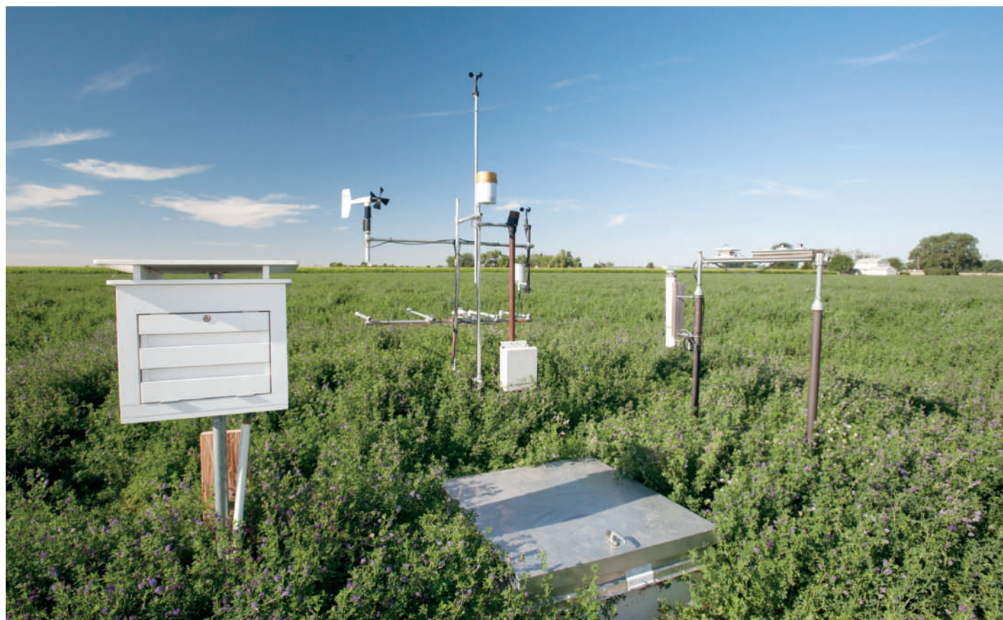
Crop lysimeter at the Colorado Agricultural Experiment Station Arkansas Valley Research Center, Rocky Ford.
