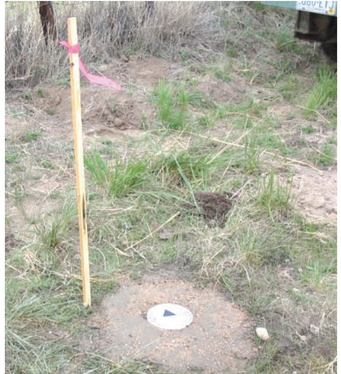
Figure 2.9. Completed monitoring well in the UARB study region.
