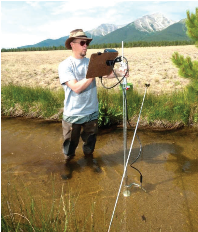
Figure 2.12. Discharge measurements in the Cottonwood Maxwell Ditch in August 2010.
