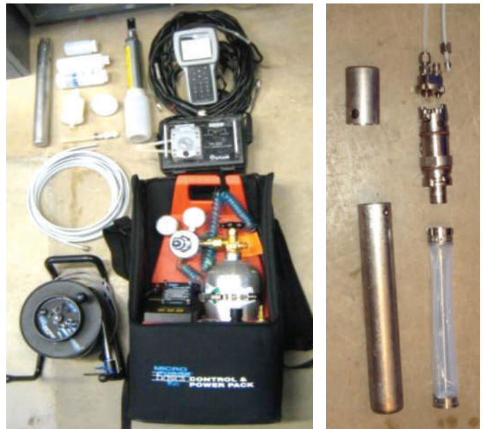
Figure 2.13. (Left) Groundwater sampling equipment (clockwise, beginning lower left): electric tape and drawdown meter; pump tubing; bladder pump, sample bottles, large and small water filters, and filter attachment tube; YSI multiprobe, YSI handpad, and cable; peristaltic surface water pump; and groundwater power pack for bladder pump operation. (Right) Close-up of disassembled bladder pump with Teflon bladder.
