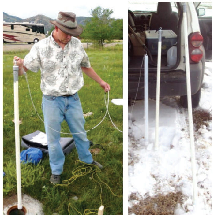
Figure 2.16. (Left) Ready for a solid slug injection test at well 127927-01 in July 2010. (Right) Various slug test devices used (from left to right). 3 ft bailer, 4 ft solid slug, and 6 ft solid slug.
