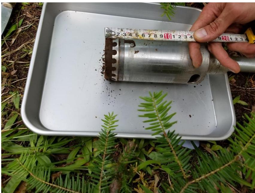
**Figure 4: Soil core collection and partition into 1-cm intervals. The ICT International 0192K1 Root Auger.**
