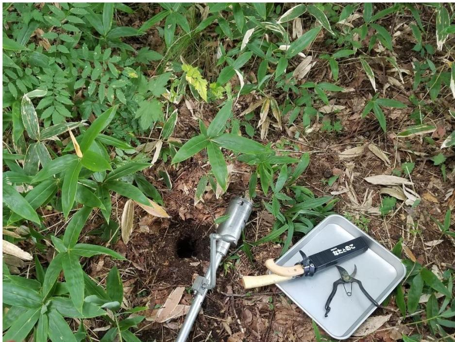
**Figure 3: Root auger, collection pan, steel clippers, and garden knife.**
