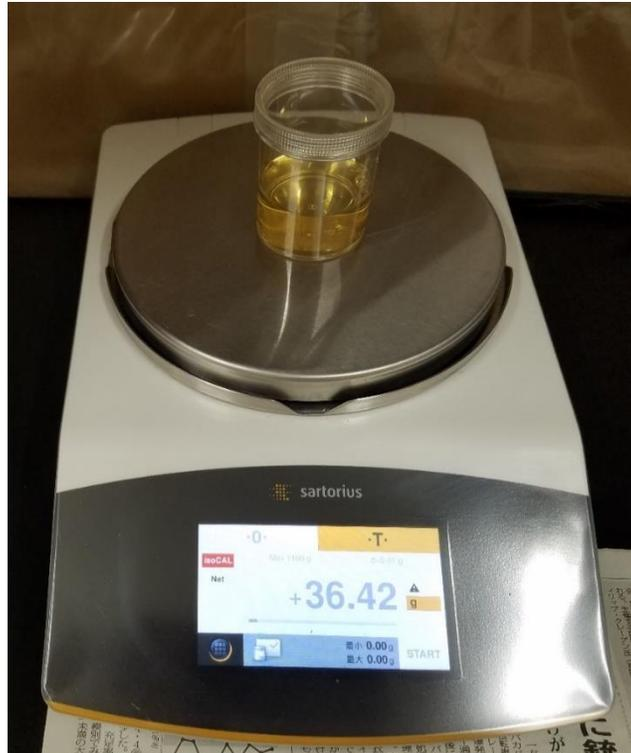
**Figure 5: Typical 100 mL U-8 Sample Container for gamma spectroscopy using a High Purity Germanium detector. Soil, vegetation and aqueous extractions were counted in these containers.**
