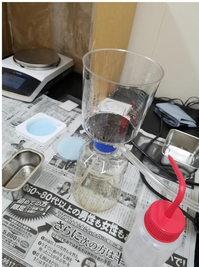
**Figure 6: Thermo Scientific™ Nalgene™ Rapid-Flow™ Sterile Disposable Filter Unit with 0.45 um PES filter + 0.45 um Omnipore Membrane Filter.**
