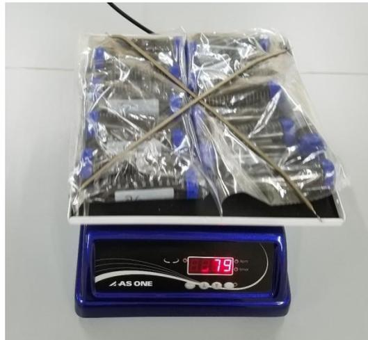
**Figure 7: An orbital shaker with timer function used for mixing soil and extraction solutions.**
