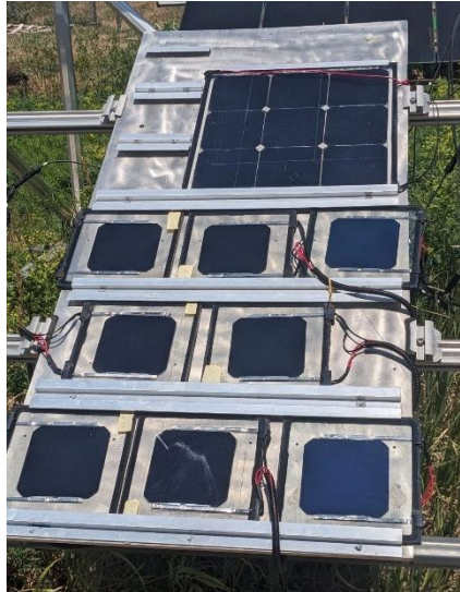
Figure 15: In-Situ data logger test plate shown with 8 single cell test samples at the CSU test field. A 3 x 3 cell module powers the measuring circuitry.
