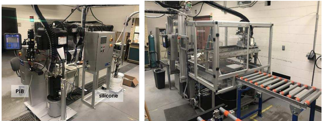
Figure 12: Graco supplied heated PIB pumping system (left) and polymer application tooling shown with 30cm x 30cm adapter plate installed (right).
