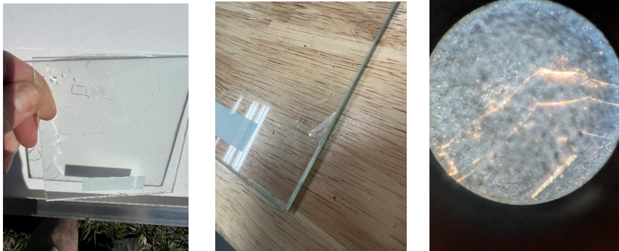
Figure 23: Right: markings observed on un-encapsulated samples exposed outdoors 124 days. Center: additional films remain under peeled regions. Right: cracks observed through 60x magnification
