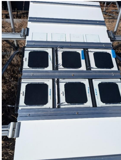
Figure 17: Static Weathering Station shown with 6 encapsulated samples and 4 un-encapsulated samples
