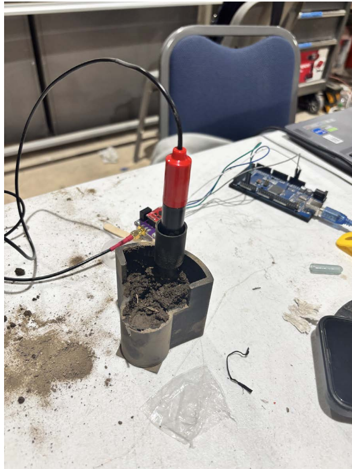
Figure 5.3: Soil collection and pH sensor testing. Soil moisture content was characterized to identify the minimum water-to-soil mass ratio required for reliable pH readings. Readings below approximately 2% moisture content were unstable; consistent and repeatable readings required a minimum of 5% moisture content. Testing was conducted using representative soil types sourced from the CSU Soil Lab.
