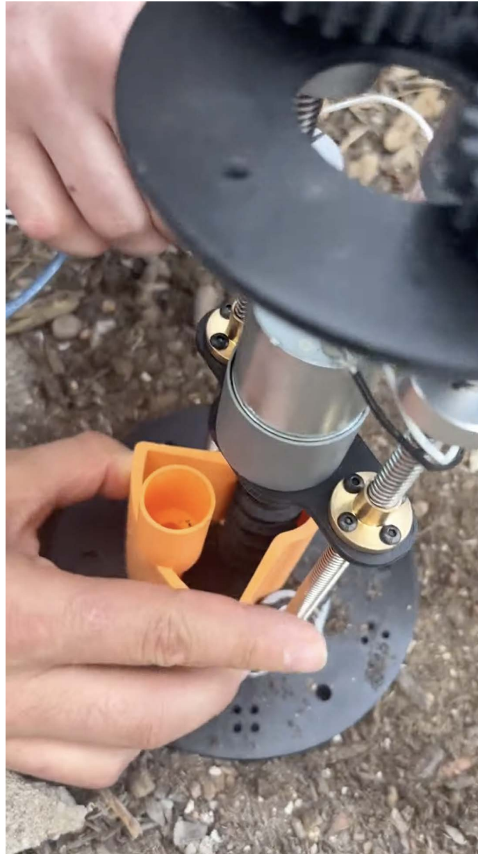
Figure 5.1: Auger mechanism during torque validation testing. The auger was driven into representative soil samples to validate that the 150:1 gearbox provided sufficient torque for penetration and sample collection without stalling the motor beyond its rated current limit.
