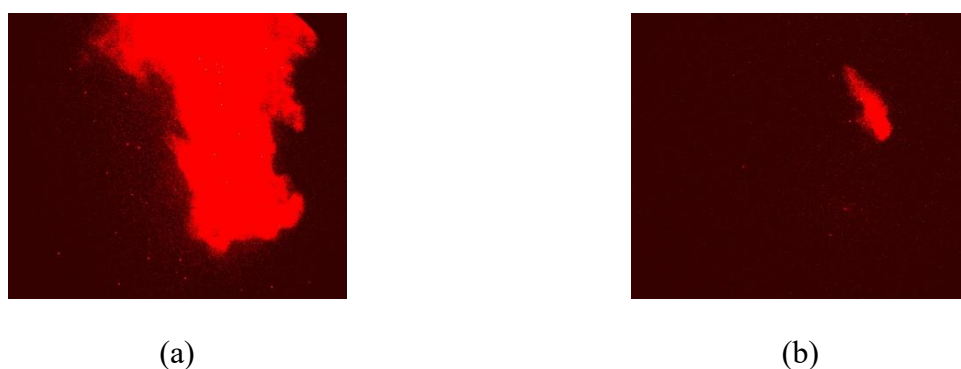
Fig. 4.7 Representative images of OH chemiluminescence 5 ms after the laser deposition (a) Ignition at Laser energy – 250 mJ (b) Long mode failure at Laser Energy – 80mJ. Camera gate – 1 ms.
