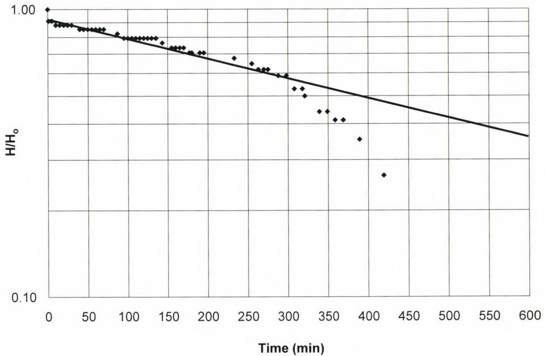
Fig. E.4. Plot of head ratio ( $H/H_0$ ) versus time for well B8.
