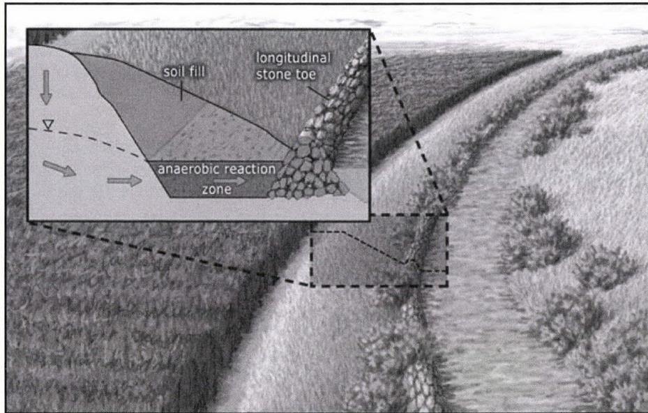
Fig. 1.1. Reactive stream stabilization (RS2) structure. The anaerobic reaction zone represents the permeable reactive barrier composed of sawdust. The blue arrows indicate the direction of groundwater flow.
