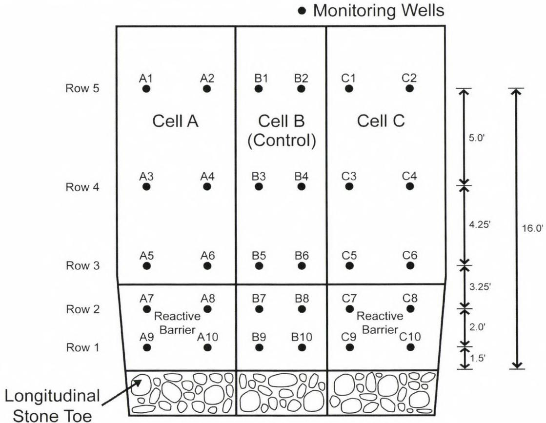
Fig. 3.13. Monitoring well network.
