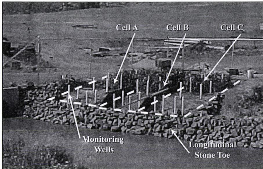
Fig. 3.1. Experimental field structure.
