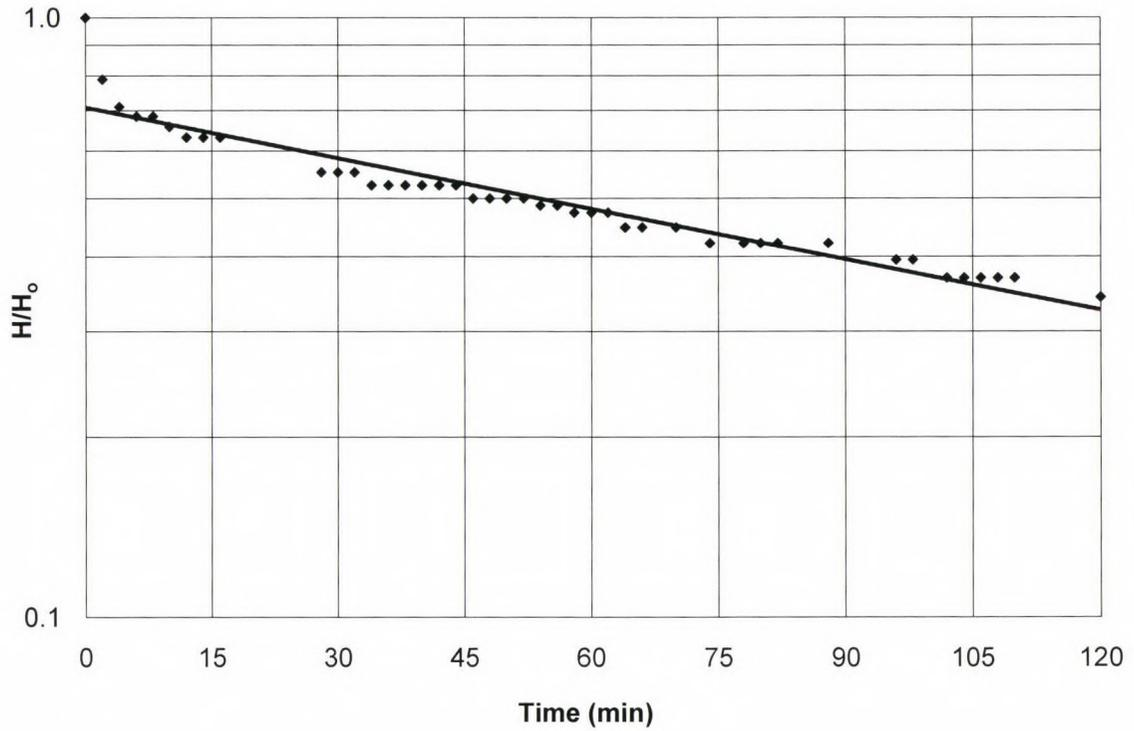
Fig. E.1. Plot of head ratio ( $H/H_0$ ) versus time for well A3.
