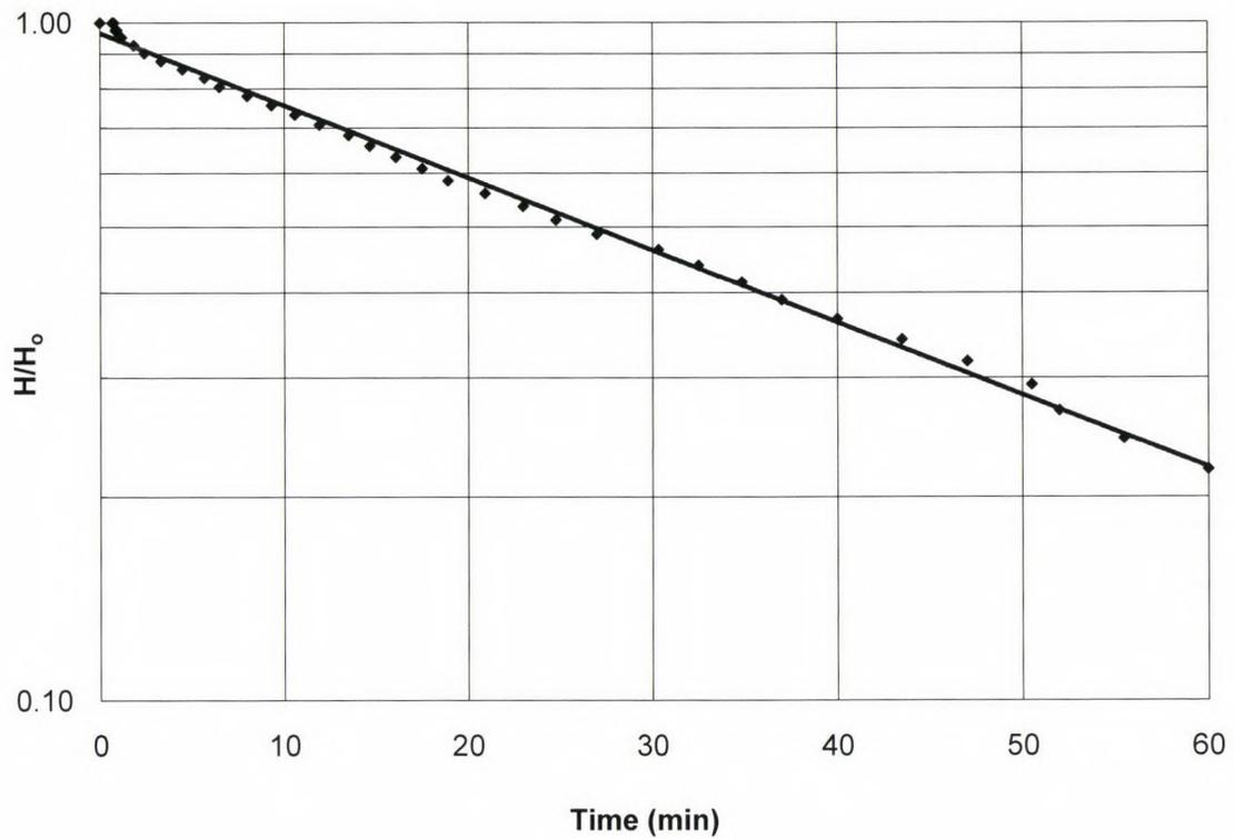
Fig. E.2. Plot of head ratio ( $H/H_0$ ) versus time for well A10.
