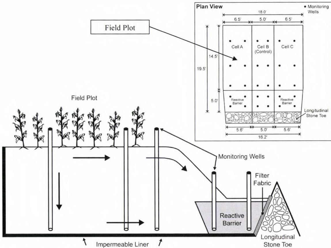
Fig. 3.2. Cross section of research cell and plan view of field structure.
