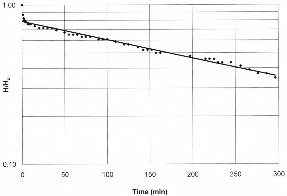
Fig. E.3. Plot of head ratio ( $H/H_0$ ) versus time for well B4.
