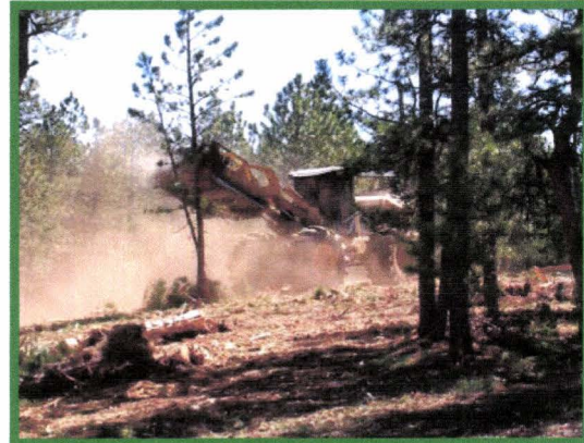
The Hydro-Ax is hard at work masticating trees on the first 67 acres in Lory State Park.
