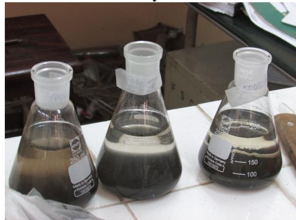
**Water-ashes mixture after 24 hours of settling**
