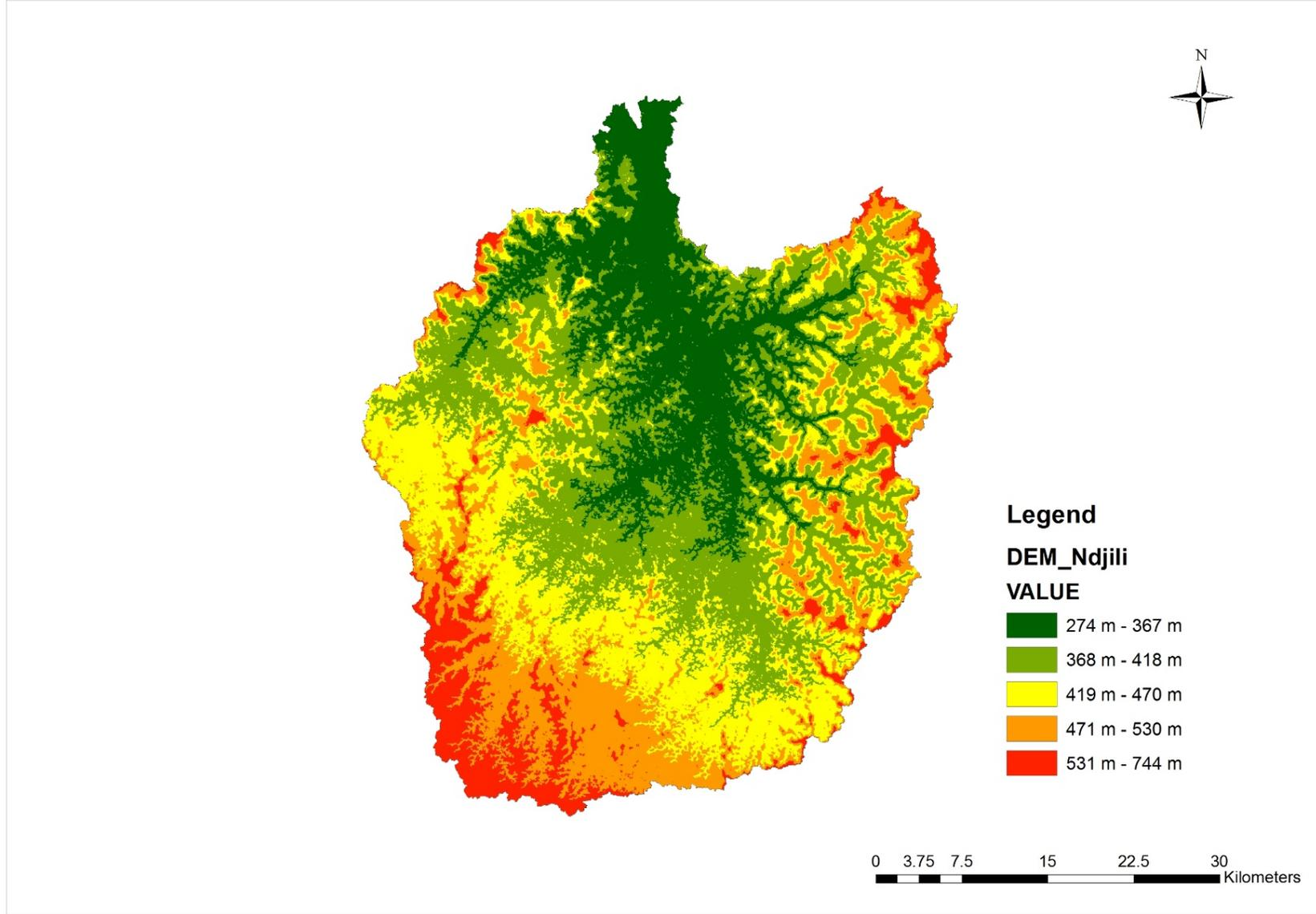
**Figure 3.3 – Digital elevation model (DEM) of the N'djili River Basin**
