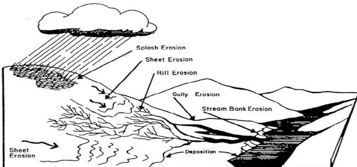
Figure 2.1 – The mechanisms of soil erosion (USACE 1985)
