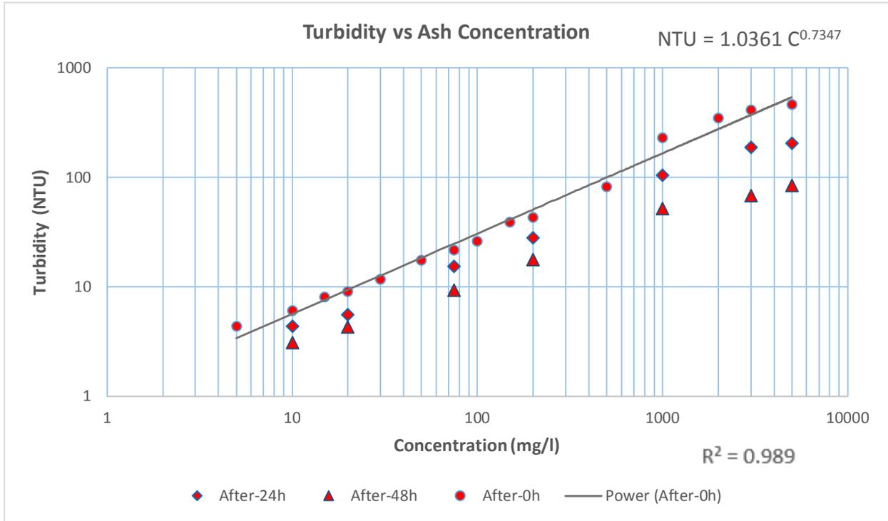
**Figure 4.27 - Effect of ash concentration on water turbidity.**
