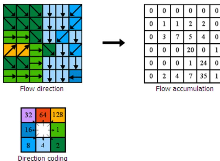
**Figure 4.7 - Determining the accumulation of flow**
