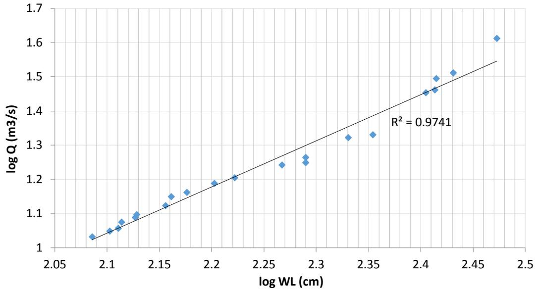
**Figure 3.12 - Flow rating curve at the N'djili Station 2**
