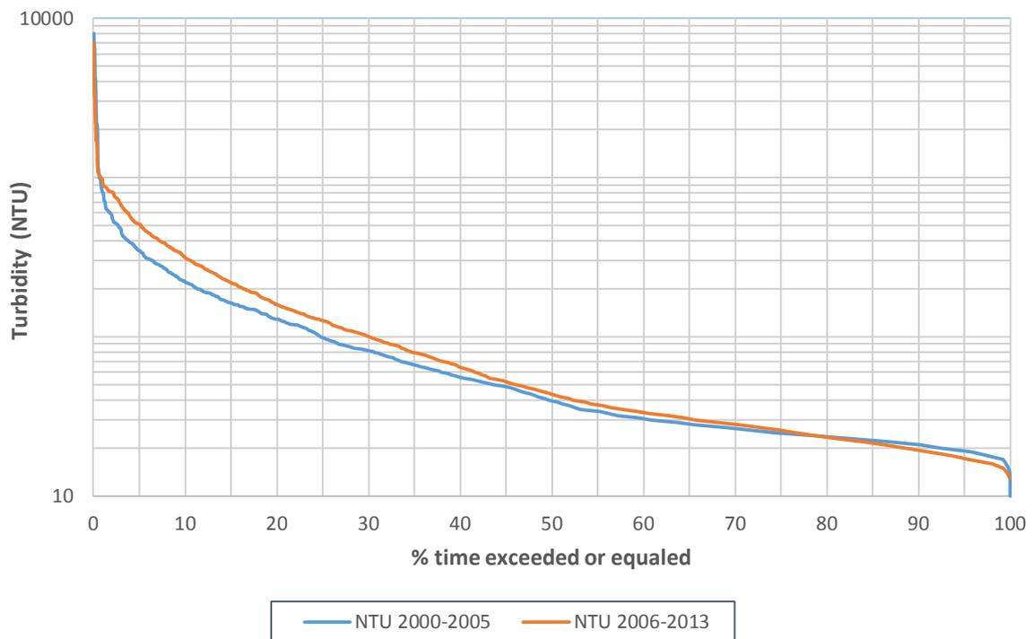
**Figure 1.6 – Exceedance probability curves of turbidity at the intake of the N’djili water plant for the periods 2000-2005 and 2006-2013**
