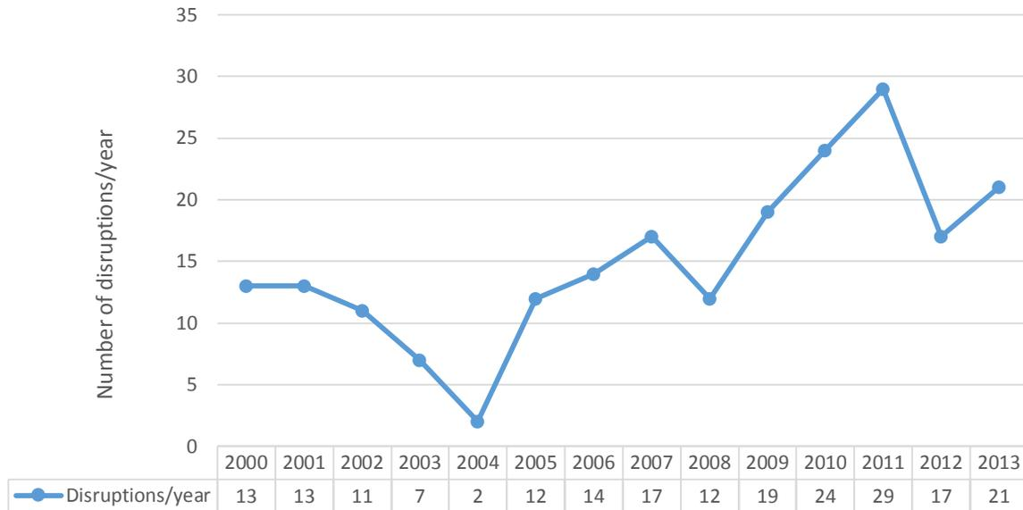
**Figure 1.5 – Number of water pumping disruptions per year at the N’djili water treatment plant due to high turbidity**
