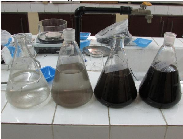
**Water-ashes mixture after 0 hour of settling**
