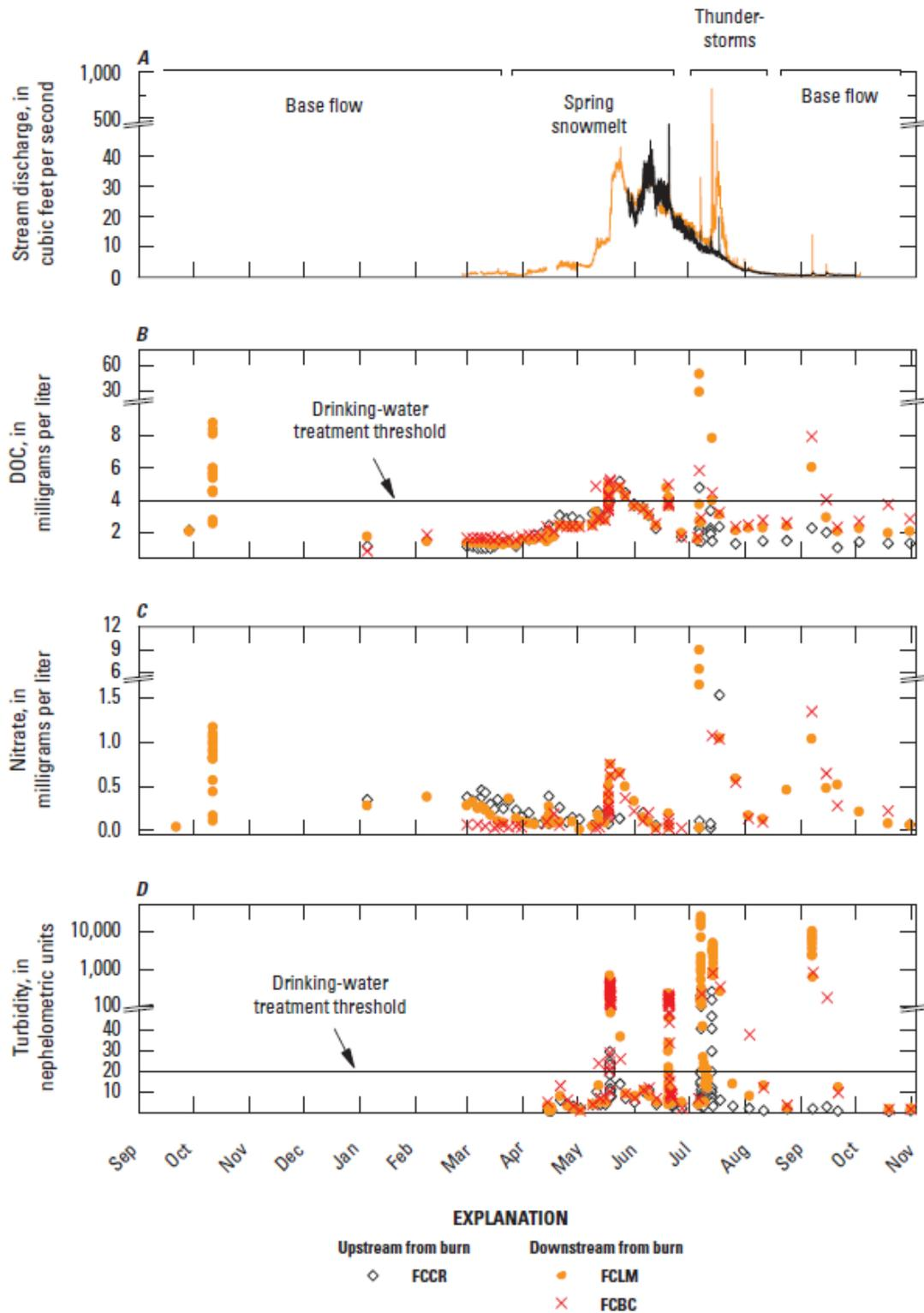
**Figure 2.5 - Stream discharge at 5-minute intervals and selected water quality characteristics in 2010-2011 measured in Fourmile Creek, Colorado, at monitoring stations FCCR, FCLM, and FCBC (Writer et al., 2012).**
