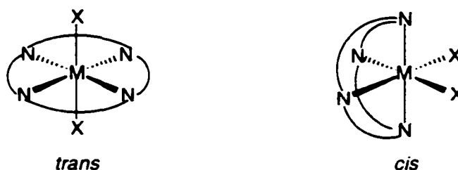
Figure 2.9 Possible coordination geometries of cyclams
