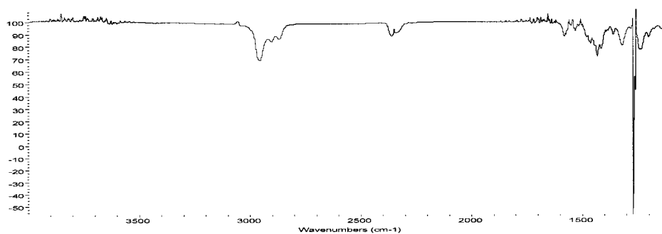
Figure S3.8 IR spectrum of \text{Na}_2(3,5\text{-DTBC}) (ca. 0.1 M in \text{CH}_2\text{Cl}_2 , \text{CaF}_2 cell, under \text{N}_2 ).
