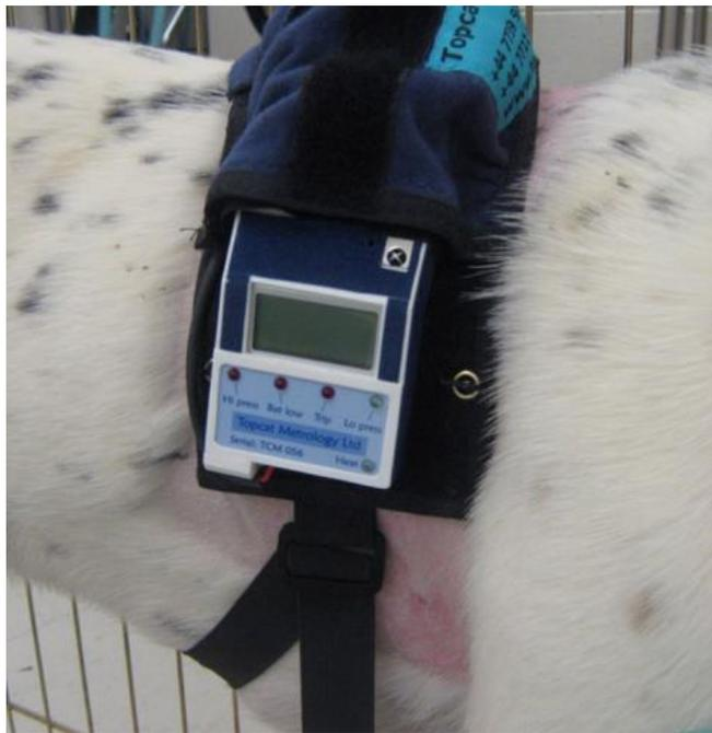
**Figure 4.1:** Thermal nociceptive threshold testing device (Topcat Metrology Ltd.) was applied on the latero-dorsal aspect of a dog's thorax. The thorax was clipped of hair allowing better contact between the thermal probe and skin of the dog.
