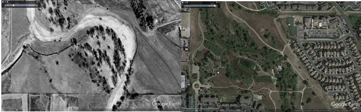
Figure 1: Comparison of a section of Cherry Creek showing channel planform and geometry evolution between 1955 and 2019.
