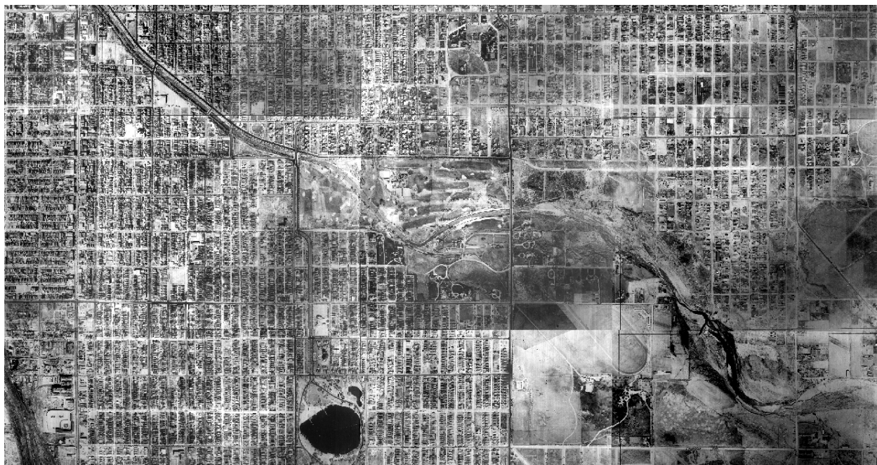
Figure 4.21: 1933 aerial photograph (King 1933) of Cherry Creek in the lower sub-watershed through the City and County of Denver. The anthropogenic-confined trapezoidal straight channel is visible near the confluence with the South Platte River (upper left). Prior to urban development the creek was an unconfined meandering sand bed channel (lower right).
