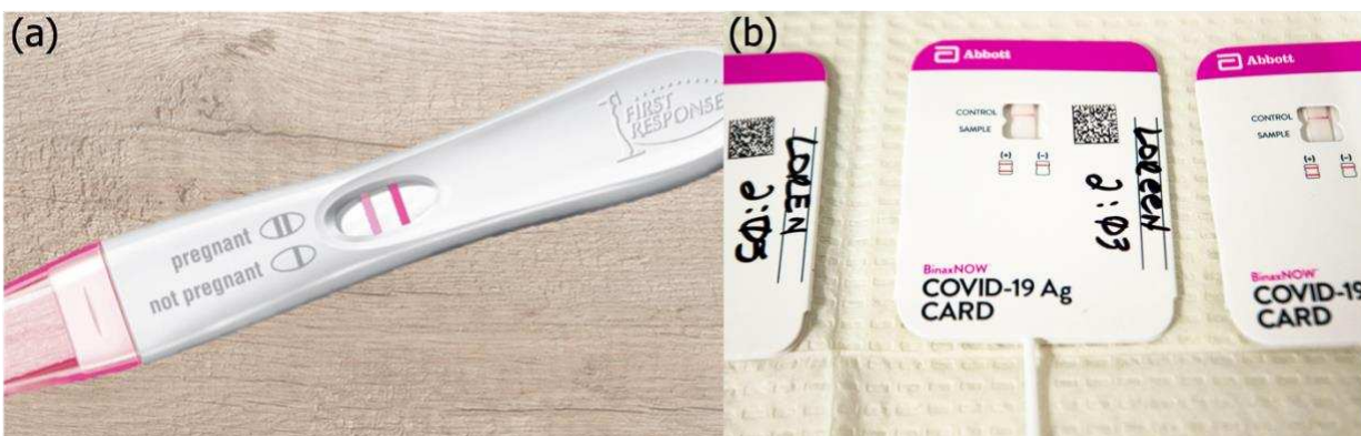
Figure A5.10. (a) Image of a home pregnancy test with housing. (b) Photograph Binax COVID-19 home test kit with integrated nasal swap.
