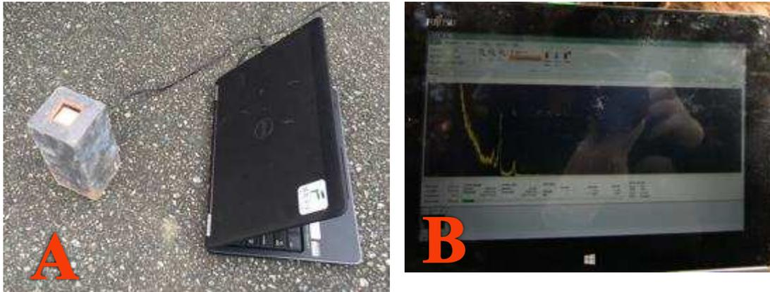
Figure 6: (A) 1-cm<sup>3</sup> Kromek CZT detector (B) The whole-body measurement of the boar using the instrument
