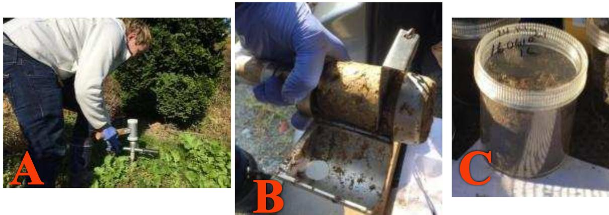
Figure 10: (A) Soil samples were collected in the boar home range. (B) Samples were sliced into three 3-cm pieces. (C) Example of a prepared sample.
