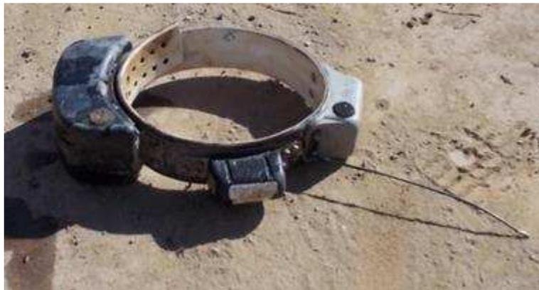
Figure 7: Radiocollar used on the boar to determine home range and external dose
