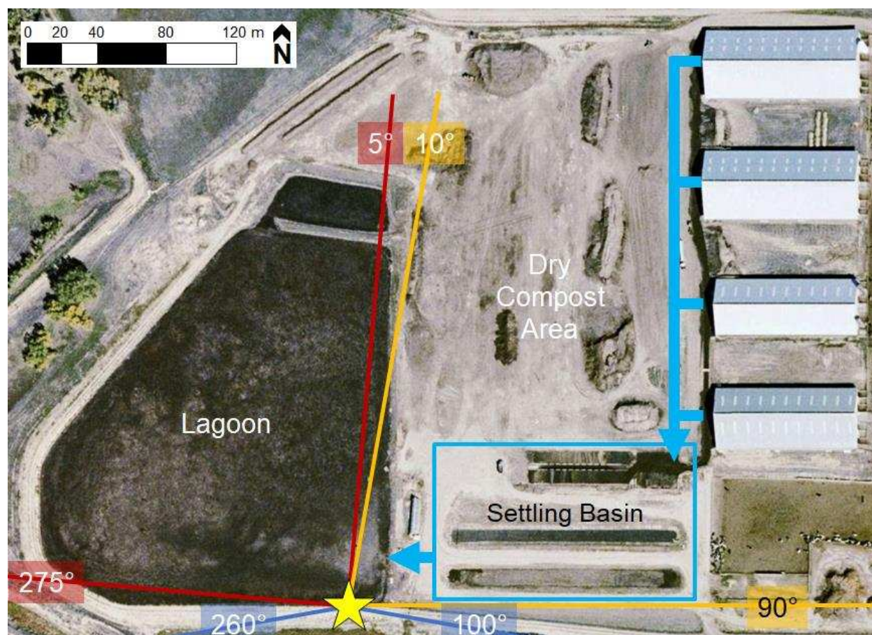
Figure 3.1. Satellite image of manure management and the free-stall barns on the dairy. The eddy covariance station is indicated by a yellow star, while light blue arrows show the flow of waste from the lactating cow barns. Before being pumped into the lagoon via an underground pipe, washed waste flows through a sedimentation basin (lower right) to reduce total solids. Lagoon (left), dry compost area (right), sedimentation basin (lower right), and lactating cow barns (far right) are methane sources. Colored lines and associated labeled wind direction ( \theta ) angles are to indicate how \theta filtering was done based on source area (red for lagoon source of 275^\circ < \theta < 5^\circ , yellow for NE sectors of the EC footprint with 10^\circ < \theta < 90^\circ , and blue for the field source designated for 100^\circ < \theta < 260^\circ ; excluded \theta 's are 5^\circ - 10^\circ , 90^\circ - 100^\circ and 260^\circ - 275^\circ ).
