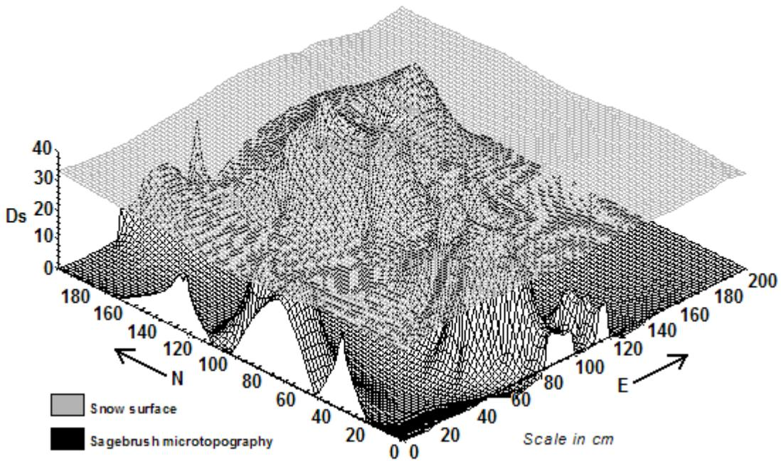
Figure 2-1: 3-D sagebrush plant and snowdrift microtopographic contour maps
