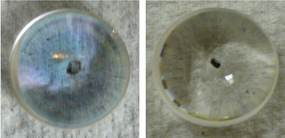
Figure 40 – Damage to focusing lenses in optical spark plug. Left: AR coated Gadium lens, sustained noticeable damage within 45 minutes. Incident beam was 9.2 mJ, 25 ns,  $\approx$  4.7 mm in diameter. Right: Uncoated SF11 lens, sustained noticeable damage within 2.5 hours. Incident beam was 9.2 mJ, 25 ns,  $\approx$  7.0 mm in diameter.
