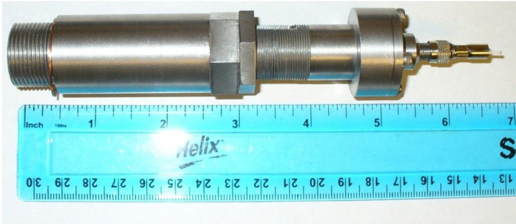
Figure 21 – Assembled optical spark plug.
