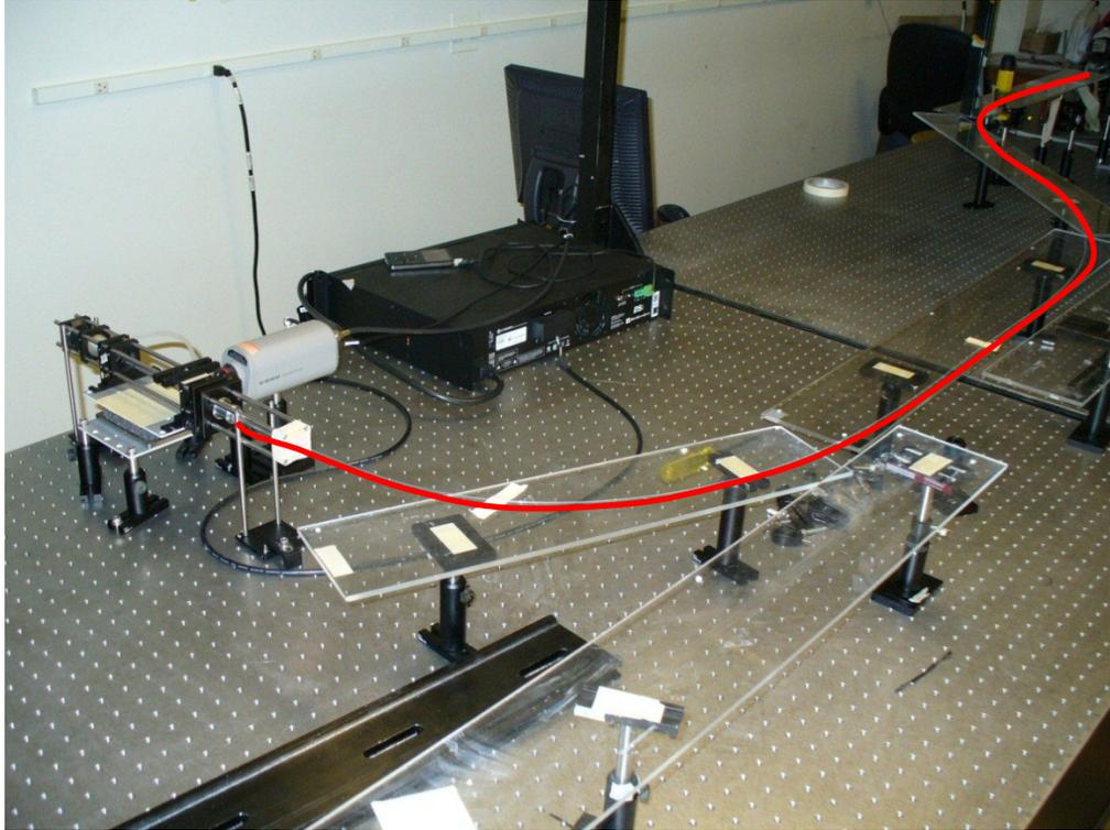
Figure 17 – Configuration (c), “3” shape. Fiber highlighted in red. Final bend  $\approx 40$  cm radius of curvature.
