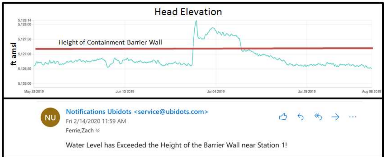
Figure 3.20: Example of a real-time alert using the Ubidots Events functionality. The uppermost box shows a hydrograph at a real-time data acquisition location at Site B. The red line in the hydrograph shows a hypothetical height of the contaminant barrier wall at Site B used to prevent the groundwater contaminants at Site B from reaching the public water supply. The bottom graph shows an example of an email that was sent in real-time as a result of the groundwater head elevation exceeding the hypothetical height of the containment barrier wall at Site B.
