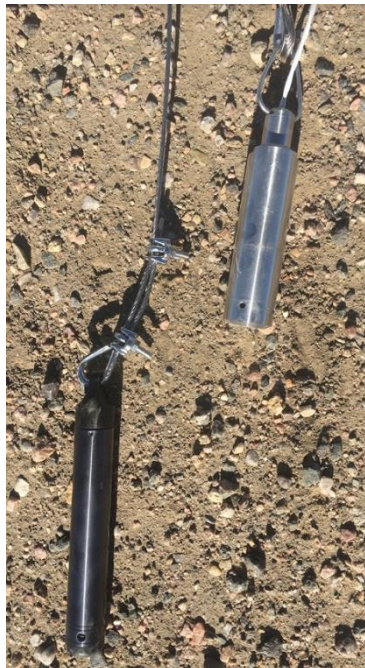
Figure 3.12: Deployment of modified/sealed FYD-101 (top) and Levelogger (bottom).
