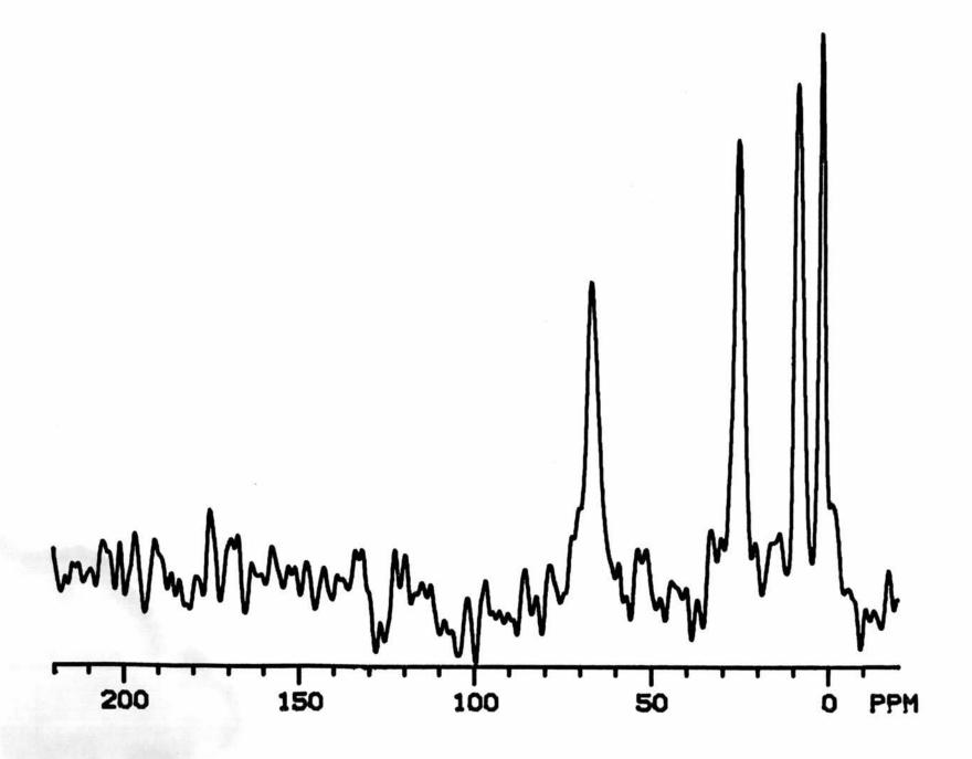
Fig. 39.  $^{13}\text{C CPMAS}$  spectrum of 8% (by weight) isobuty1 alcohol on HY(400).
