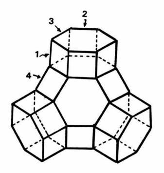
Fig. 2. Beta cages linked through the 6-rings to form the faujasite structure.
