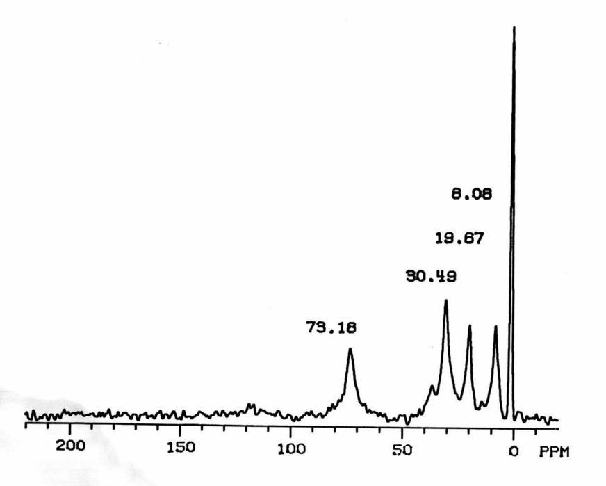
Fig. 41.  $^{13}$ C CPMAS of 12% (by weight) n-butyl alcohol on HY(400).
