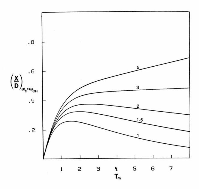
Fig. 12. Plot of (X/D) at  $\omega_2 = \omega_{CH_2}$  vs  $\tau_m$  for several values of  $T_{1CH_2}$  using W<sub>o</sub> and  $T_{1CH}$  values given in the text.
