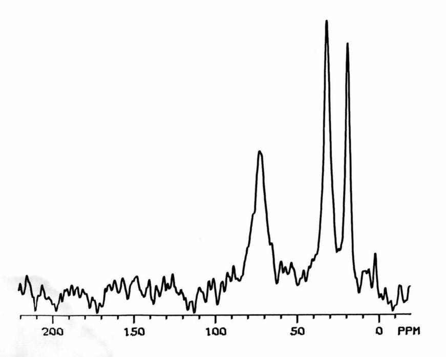
Fig. 40.  $^{13}\text{C CPMAS}$  spectrum of 11.9% (by weight) sec-butyl alcohol on HY(400).
