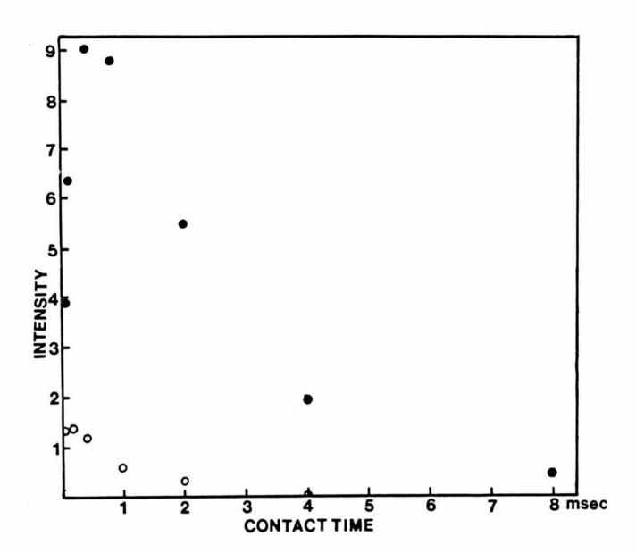
Fig. 21. Results of a rotating-frame  $^{13}\text{C}$  relaxation experiment on the methyl carbons of 15% 2-propanol on HY(400).
