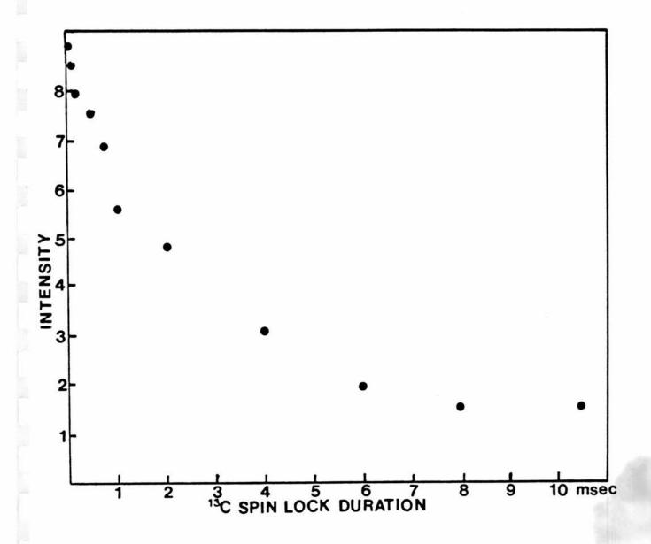
Fig. 22. Results of a rotating-frame  $^{13}\text{C}$  relaxation experiment on the carbinol carbon of 15% 2-propanol on HY(400).
