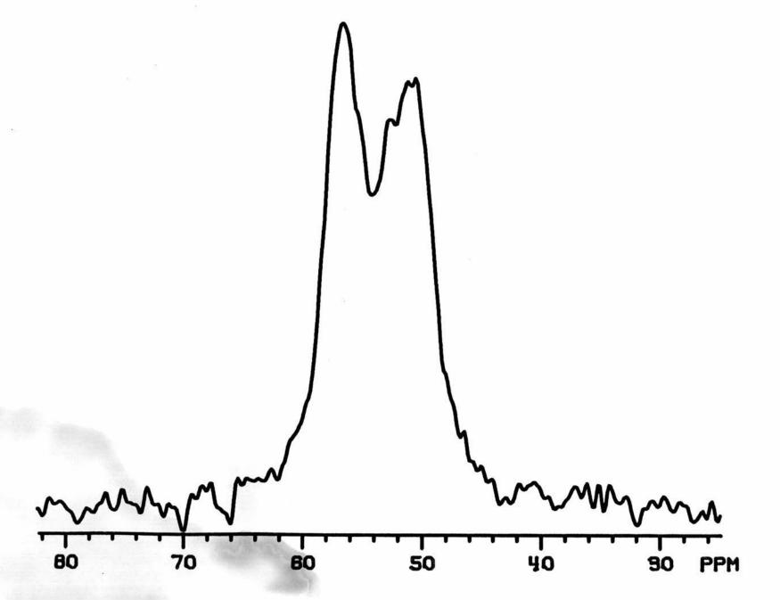
Fig. 49. Results of a rotationally-synchronized interrupted-decoupling experiment on a sample of methanol on HY(400) evacuated at  $10^{-6}$  torr at 90°C for 12 hr.
