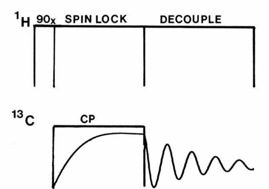
Fig. 6. Pulse sequence for measuring  $T_{1\rho}$ . After preparation by cross-polarization,  $^{13}\text{C}$  magnetization is lest to evolve in the  $^{13}\text{C}$  spin-locking field for a variable time, t.
