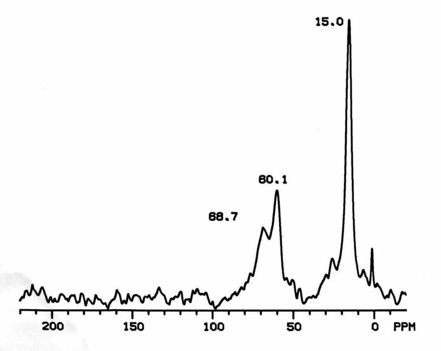
Fig. 38.  $^{13}$ C CPMAS spectrum of 5.7% (by weight) n-propanol on HY(400).
