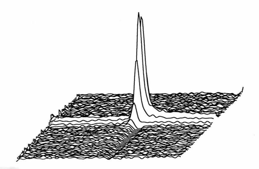
Fig. 45.  $^{13}\text{C}$  CPMAS spectrum of 22% methyl alcohol (by weight) on HY(400).
