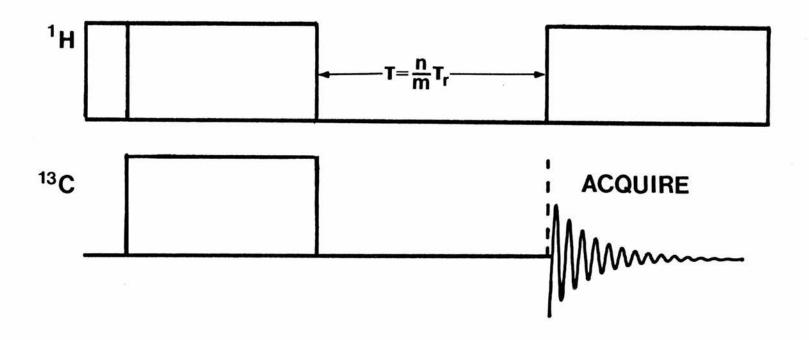
Fig. 36. Evolution of the  $^{13}\text{C}$  resonances of HY(400)/10%MeOH during the rotationally-synchronized interrupted-decoupling experiment.
