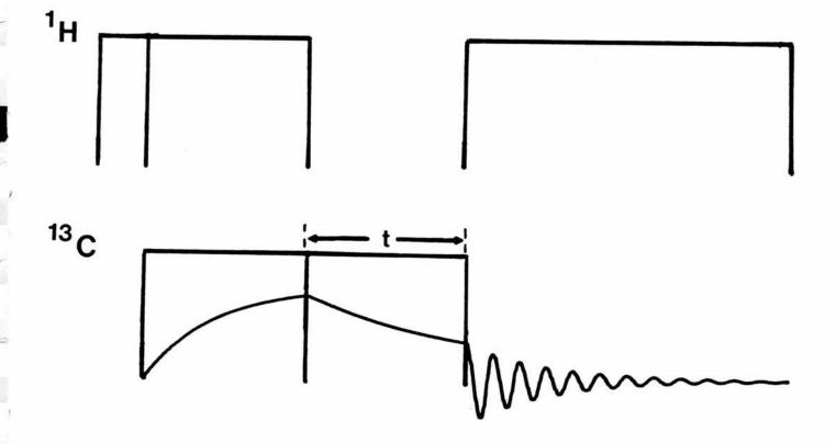
Fig. 7. Pulse sequence to measure the 90° pulse length of the  $^{13}\mathrm{C}$  r.f. field.  $^{13}\mathrm{C}$  magnetization is rotated back toward  $\mathrm{H}_{o}$  immediately after preparation by cross-polarization.
