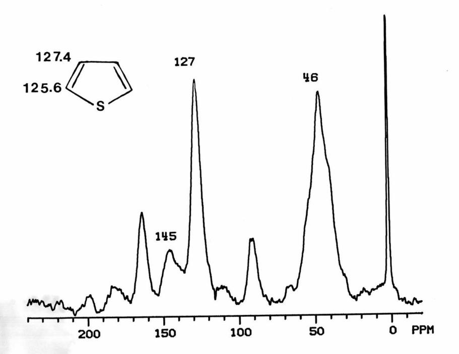
Fig. 15.  $^{13}\text{C}$  CPMAS spectrum of 15% acetaldehyde by weight on HY(400).
