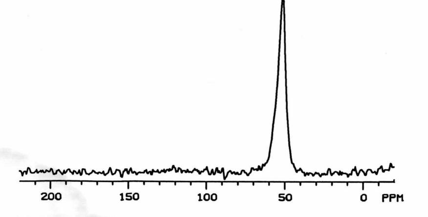
Fig. 53. Non-spinning  $^{13}\text{C}$  CP spectrum of HY(500)/8% MeOH. A chemical shift anisotropy powder pattern is displayed as well as a motionally narrowed resonance.
