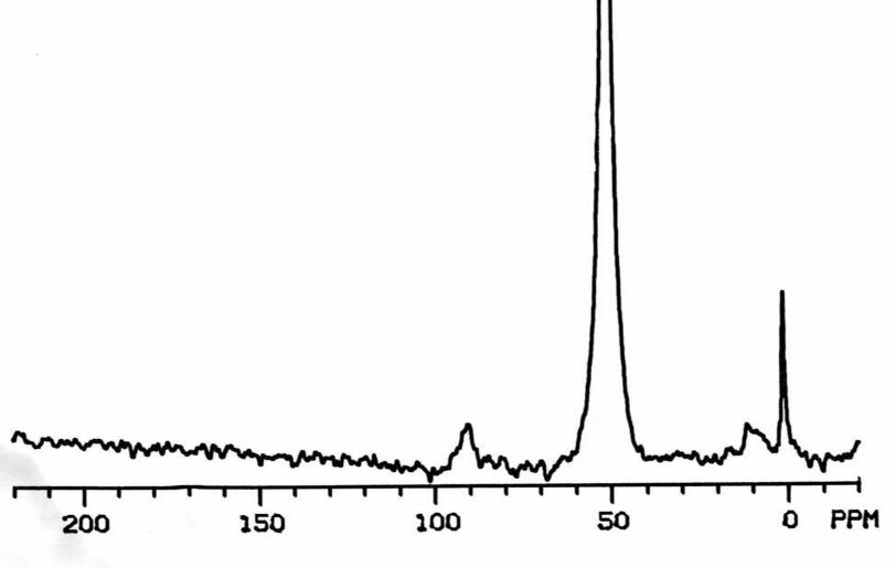
Fig. 46.  $^{1}\text{H-coupled}$   $^{13}\text{C}$  CPMAS spectrum of 22% methyl alcohol (by weight) on HY(400).
