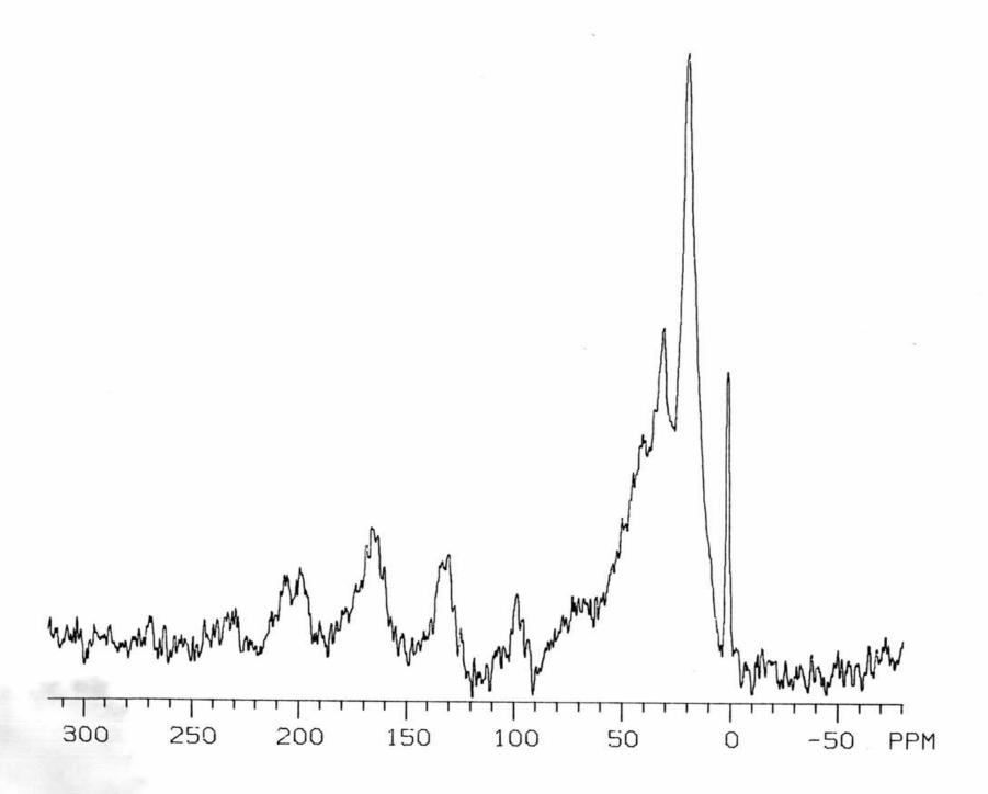
Fig. 16.  $^{13}\text{C}$  CPMAS spectrum of 30% methyl alcohol by weight adsorbed on HY(400).
