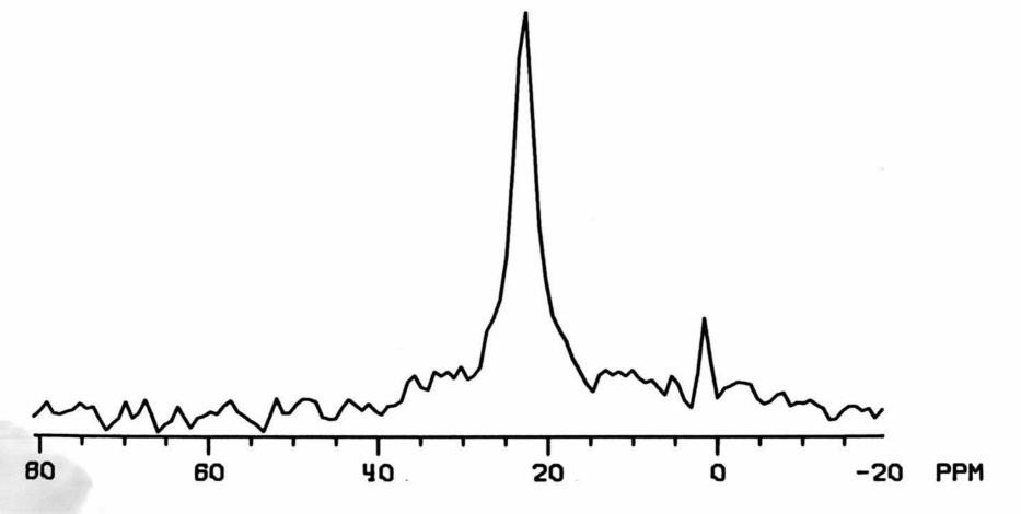
Fig. 9. <sup>13</sup>C CPMAS spectrum of 17% methylamine by weight adsorbed onto HY(150).
