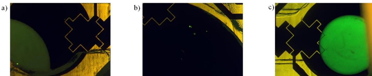
Figure 53 - a) Sample reservoir. b) Waste reservoir with unbound DNA. c) Output reservoir with eluted DNA.
