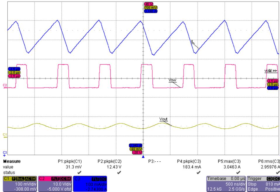
Figure 5.4 Waveforms of inductor current  $I_L$ , switch node voltage  $V_{SW}$  and output voltage  $V_{out}$  at  $V_{in}=3.5V$
