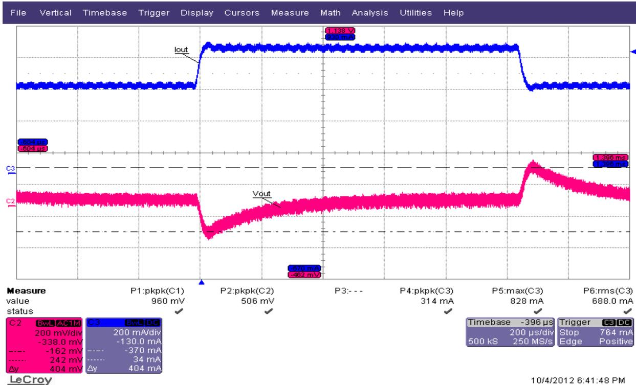
Figure 5.7 560mA to 800mA Load Transient response,  $V_{in}=5.5V$   $V_{out}=12V$
