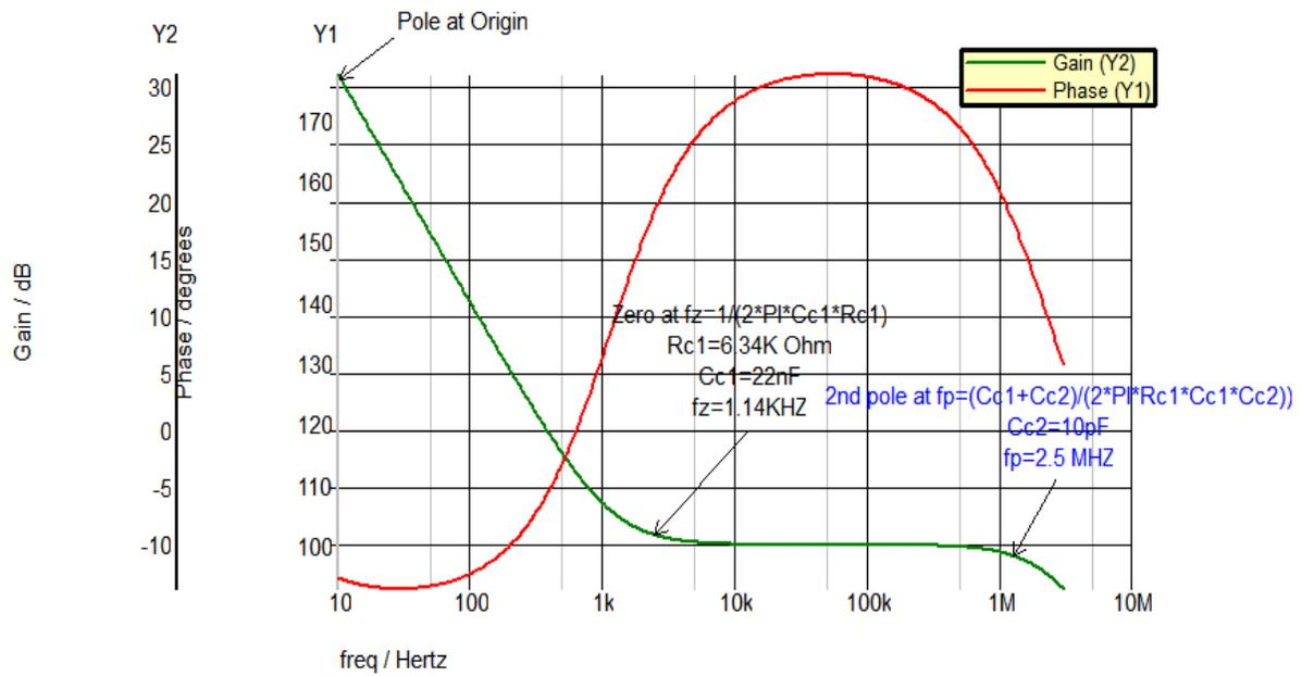
Figure 3.5 Bode Plot of type II compensation
