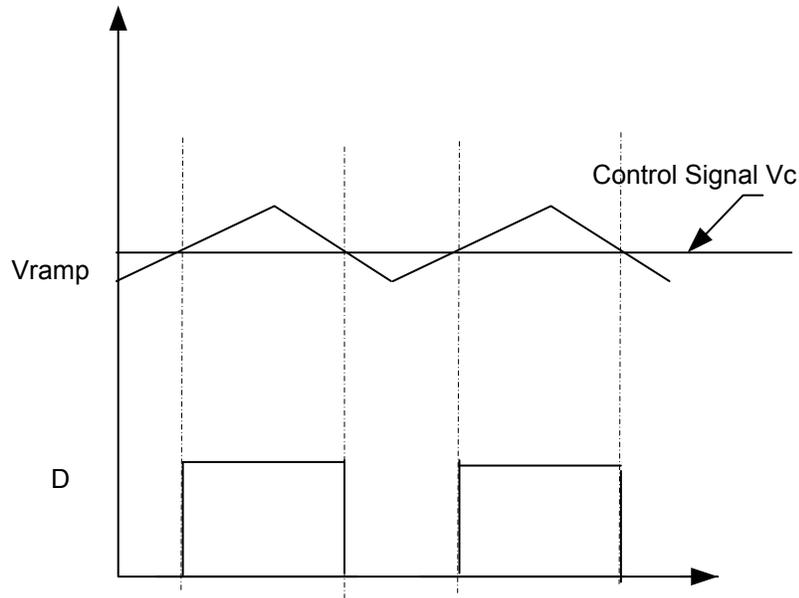
Figure 2.7 Switch current, control signal and Duty Cycle  $D$  of the VMC
