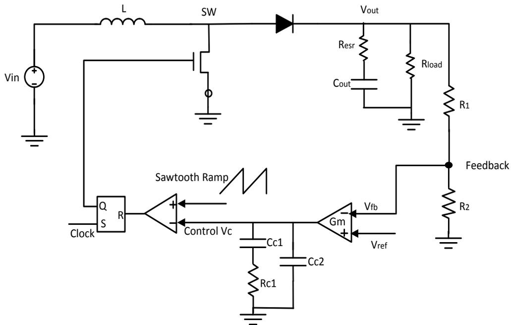
Figure 2.6 Control circuit of the boost converter with VMC
