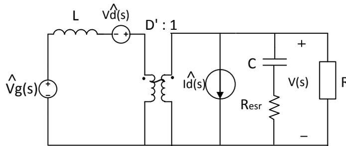
*Figure 2.1 The small-signal equivalent circuit model of boost converter*
