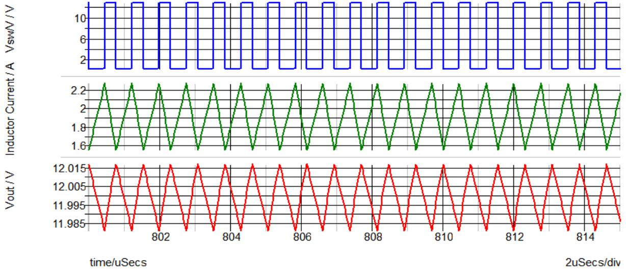
Figure 4.4 Waveform of  $V_{sw}$ ,  $I_L$  and  $V_{out}$  for  $V_{in}=5.5V$ ,  $L=3.3\mu H$
