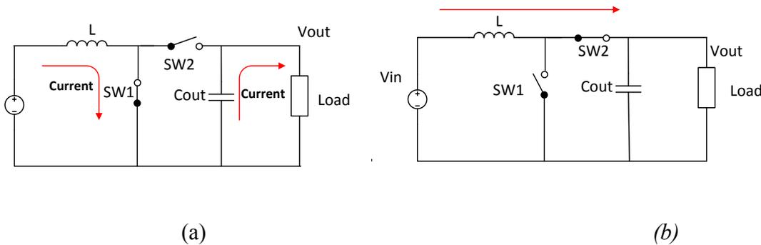
Figure 1.2 The two circuit configurations of boost converter (a) On Time (b) OFF time
