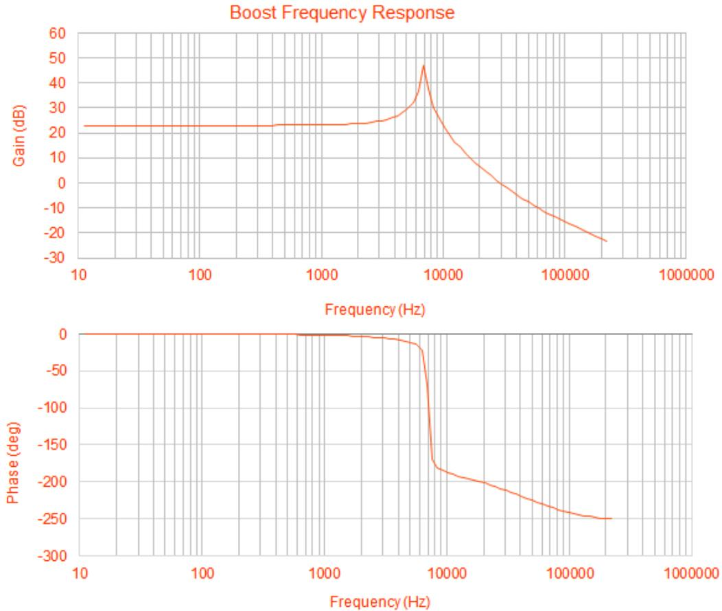
*Figure 2.8 VMC boost converter open loop bode plot*
