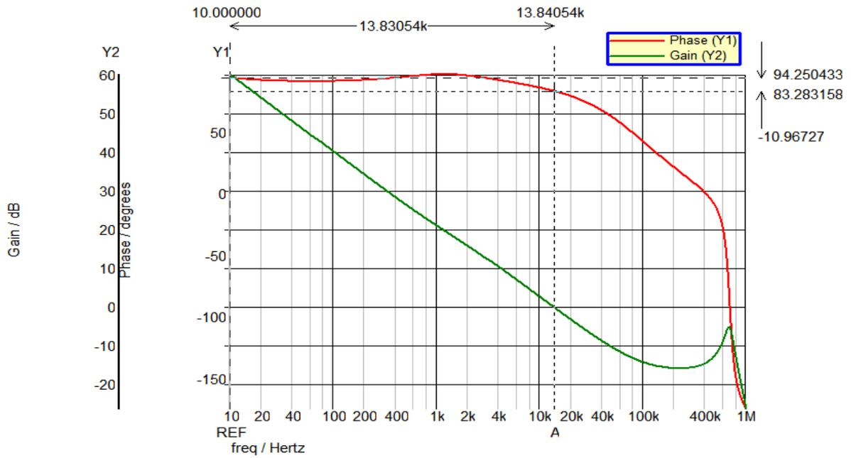
Figure 4.3 Open loop bode plot for  $V_{in}=5.5V$ ,  $L=3.3\mu H$
