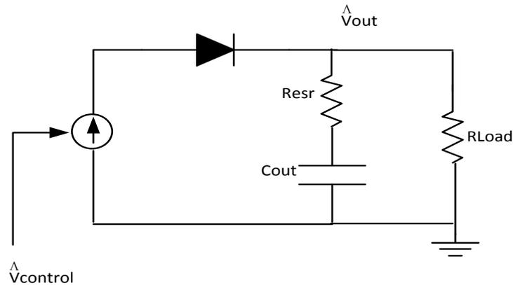
Figure 2.13 Boost converter simple average model
