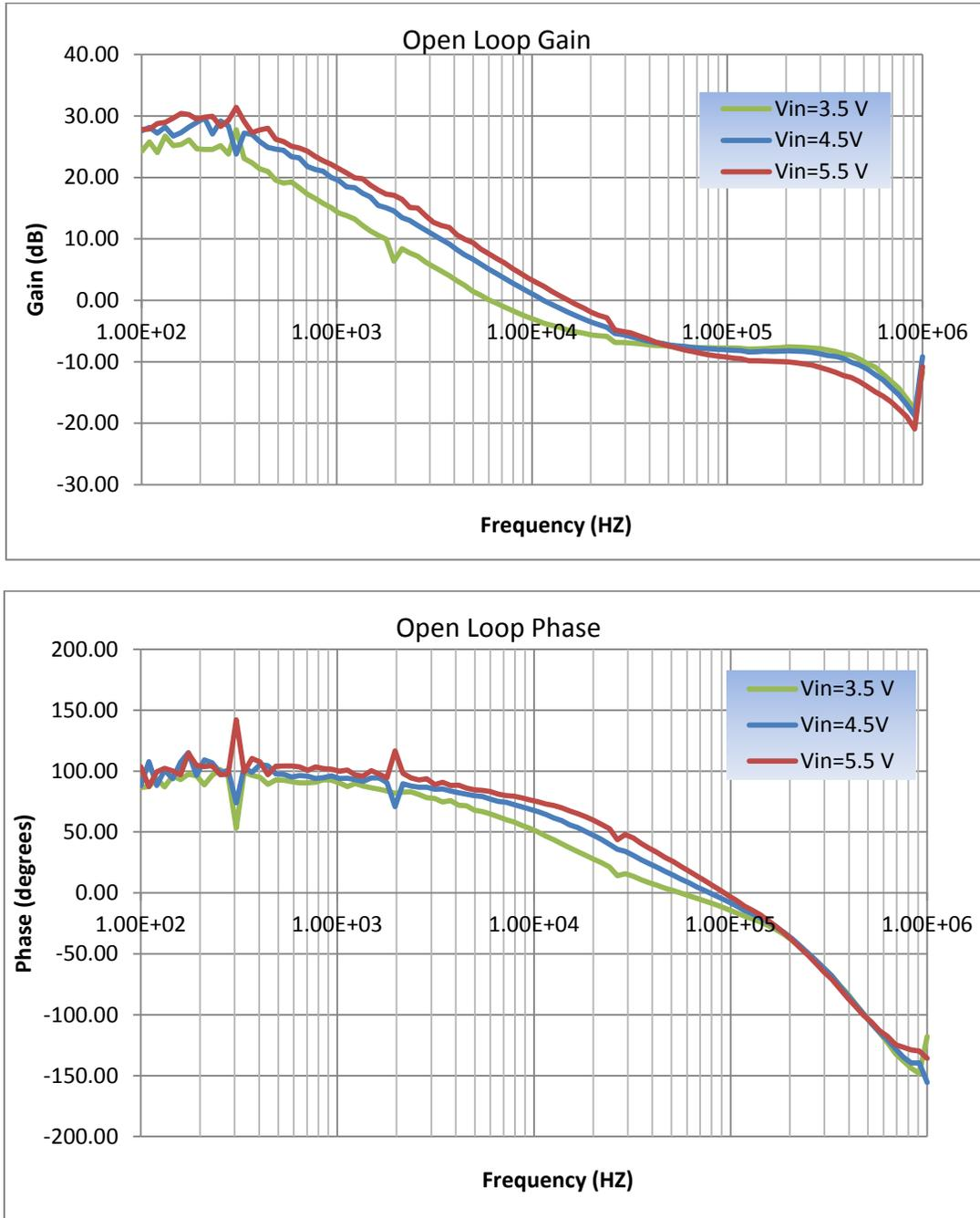
Figure 5.3 Open Loop bode plot lab test for  $V_{in}=3.5V$ ,  $4.5V$  and  $5.5V$
