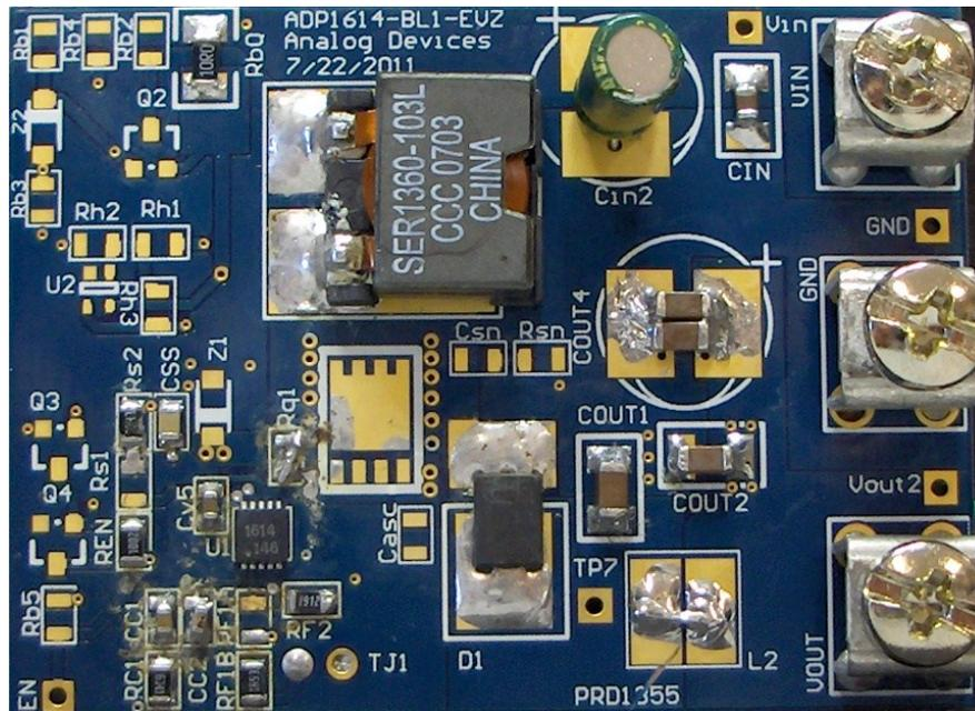
Figure 5.1 Prototype of 1.3MHz CMC Boost converter
