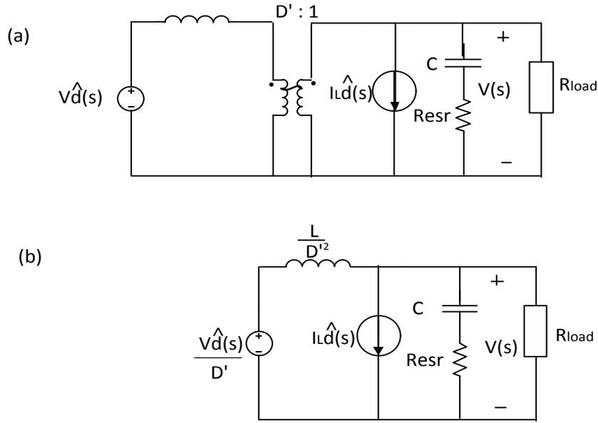
Figure 2.3 Manipulation of the boost equivalent circuit model to find  $G_{vd}(s)$ : (a) set source  $\hat{V}_g(s)$  to zero (b) moving voltage source  $\hat{d}(s)$  and the inductor through the DC transformer
