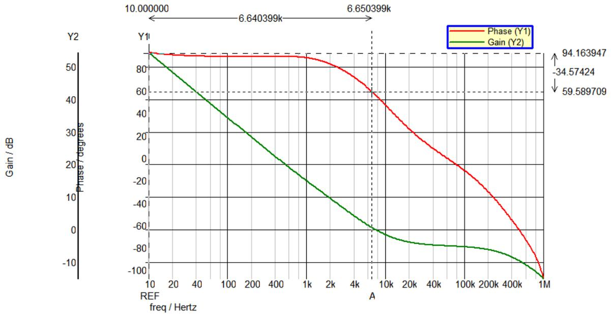
Figure 4.5 Open loop bode plot for  $V_{in}=3.5V$ ,  $L=10\mu H$
