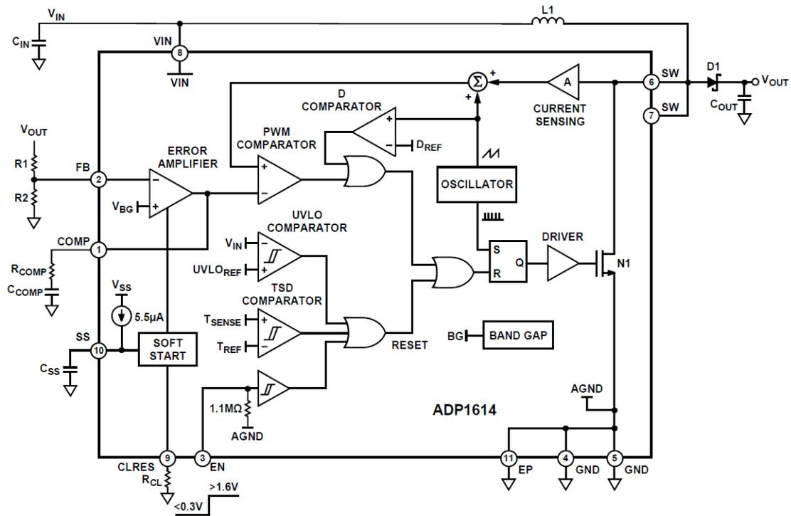
Figure 3.1 Block Diagram with Step-Up Regulator Application Circuit (courtesy of ADI)
