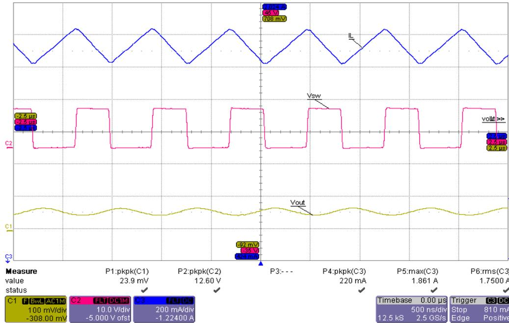
Figure 5.5 Waveforms of inductor current  $I_L$ , switch node voltage  $V_{SW}$  and output voltage  $V_{out}$  at  $V_{in}=3.5V$
