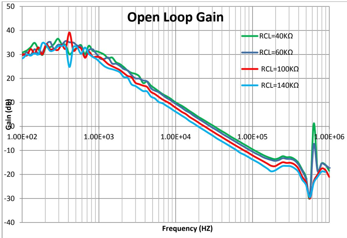
*Figure 6.1 Open Loop gain varies with current limit resistor  $R_{CL}$*
