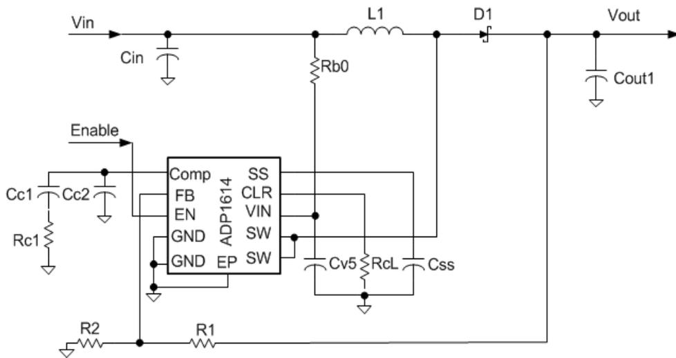
Figure 3.2 Schematic of the boost converter using ADP1614 (courtesy of ADI)
