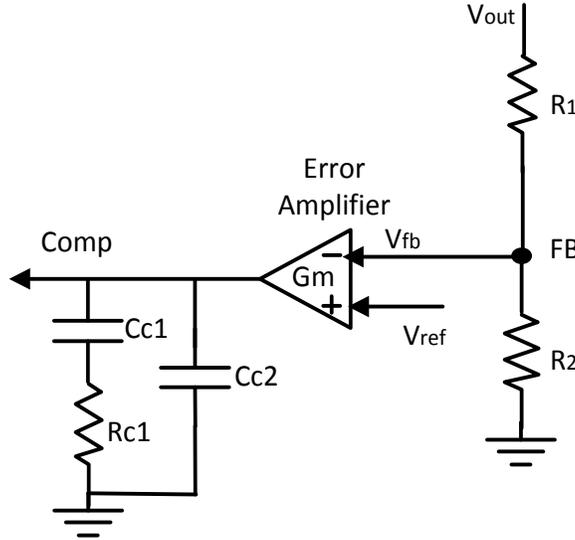
Figure 3.4 Compensation components
