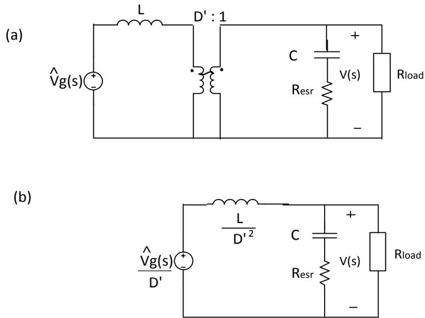
Figure 2.2 Manipulation of the boost equivalent circuit model to find  $G_{vg}(s)$ : (a) set source  $\hat{d}(s)$  to zero (b) moving voltage source  $\hat{V}_g(s)$  and the inductor through the DC transformer
