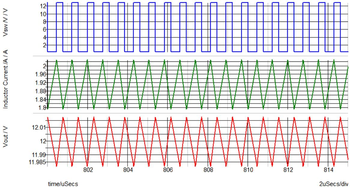
Figure 4.8 Waveforms of  $V_{sw}$ ,  $I_L$  and  $V_{out}$  for  $V_{in}=5.5 V$ ,  $L=10\mu H$
