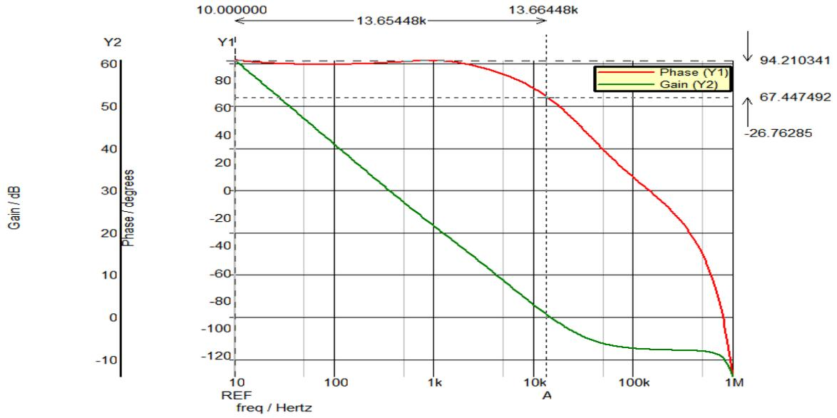
Figure 4.7 Open loop bode plot for  $V_{in}=5.5V$ ,  $L=10\mu H$
