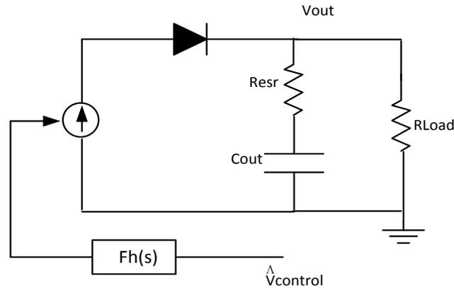
Figure 2.14 Current Mode control Boost converter enhanced model with high frequency correction
