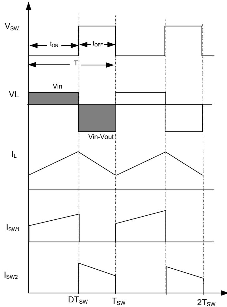
Figure 1.3 Waveforms of current and voltage in a boost converter operating in continuous conduction mode
