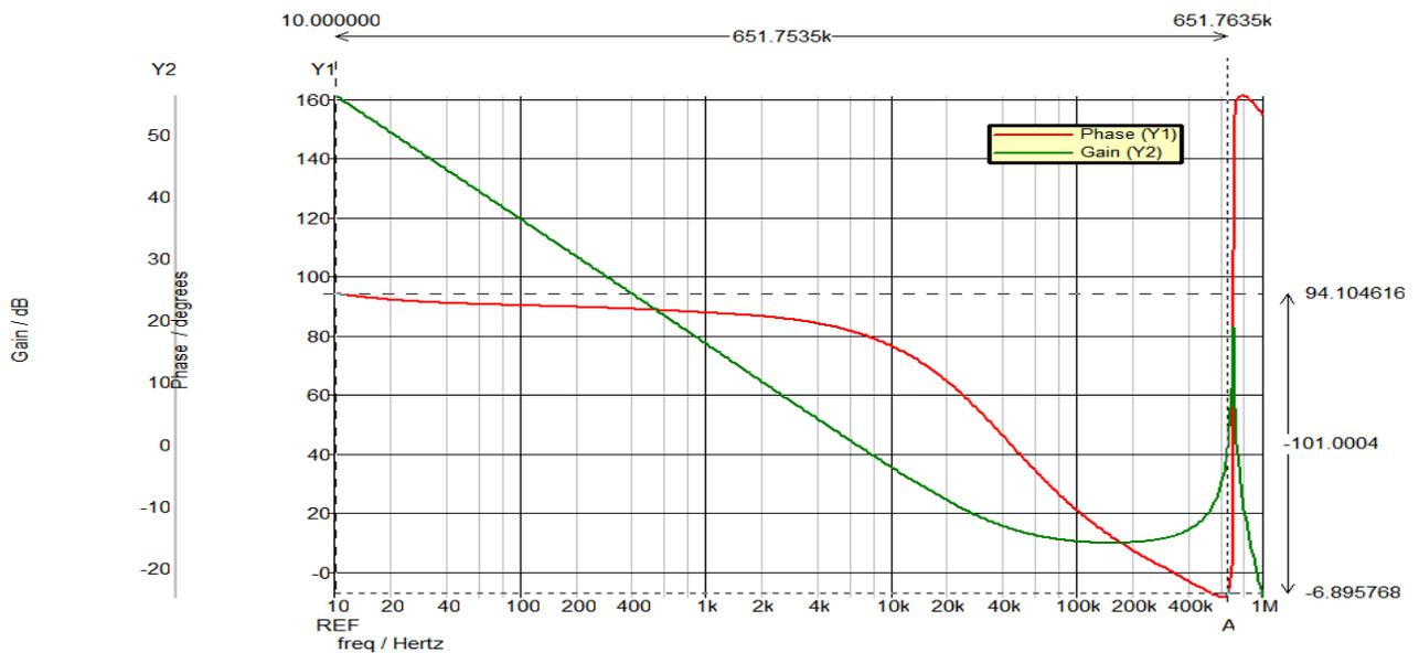
Figure 4.1 Open loop bode plot for  $V_{in}=3.5\text{V}$ ,  $L=3.3\mu\text{H}$
