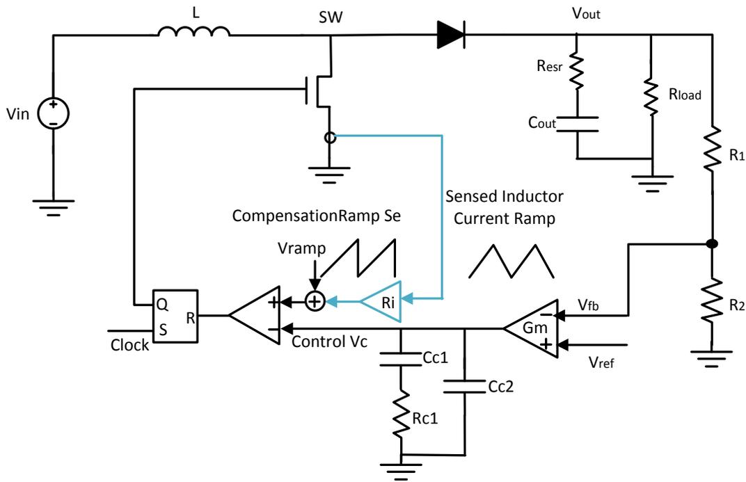
Figure 2.9 control circuit of the boost converter with CMC
