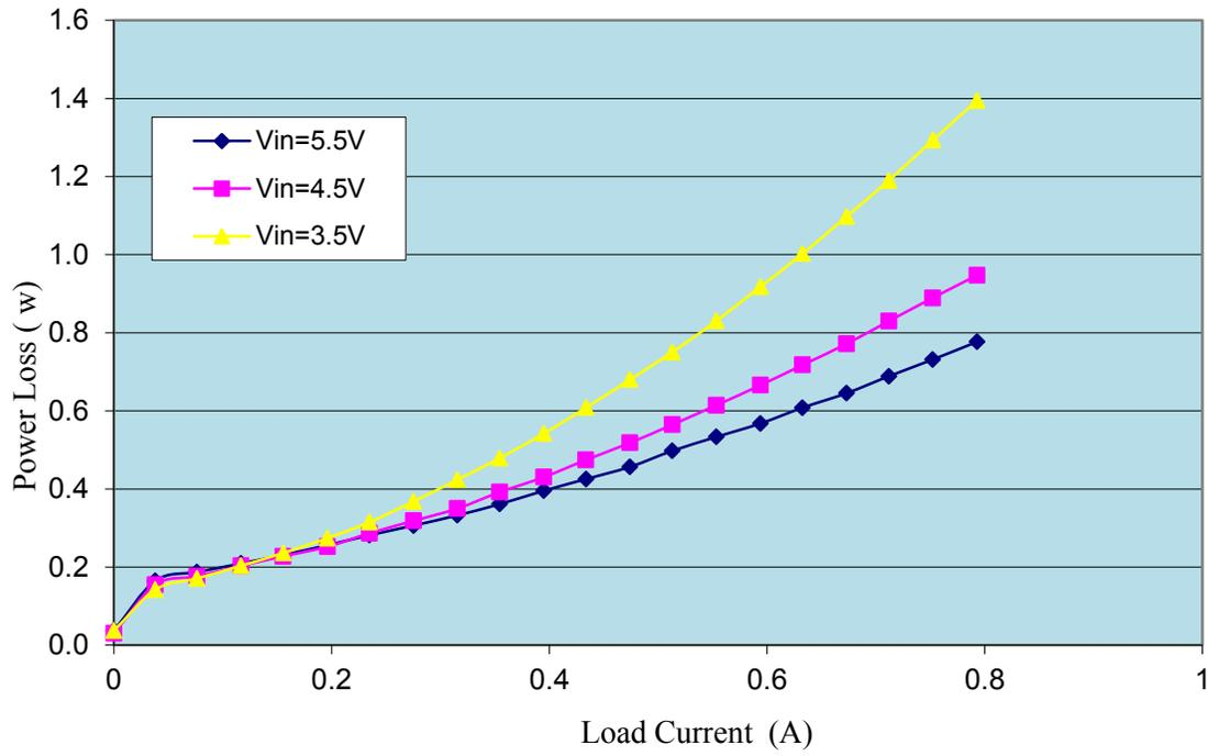
Figure 5.8 Efficiency test result for  $V_{in}=3.5V$ ,  $4.5V$  and  $5.5V$
