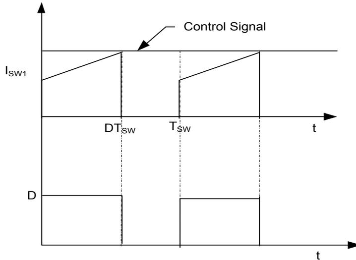
*Figure 2.10 Switch current, control signal and Duty Cycle  $D$  of the CMC*
