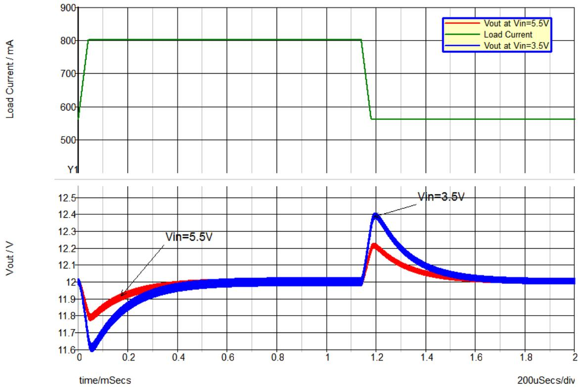
Figure 4.9 560mA to 800mA load Transient for  $L=10\mu H$
