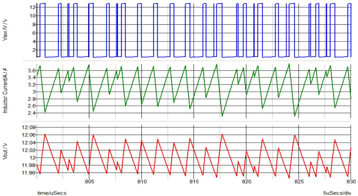
*Figure 4.2 Unstable waveform of  $V_{sw}$ ,  $I_L$  and  $V_{out}$  at  $V_{in}=3.5V$ ,  $L=3.3\mu H$*
