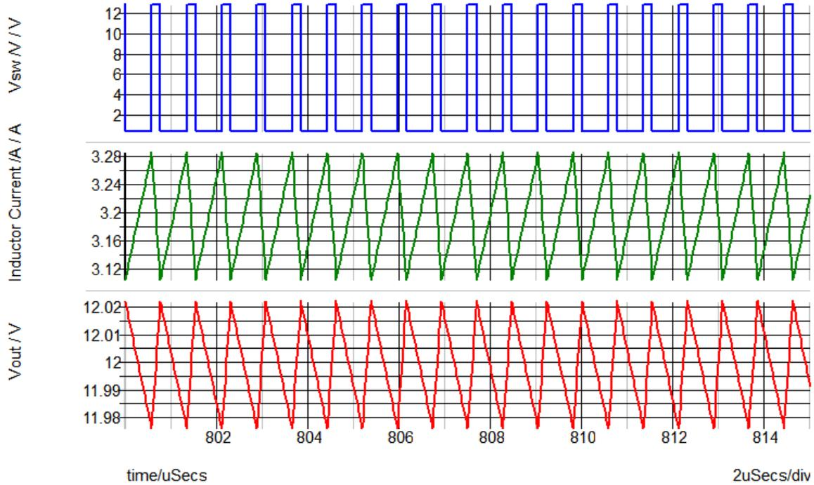
Figure 4.6 Waveform of  $V_{sw}$ ,  $I_L$  and  $V_{out}$  for  $V_{in}=3.5V$ ,  $L=10\mu H$
