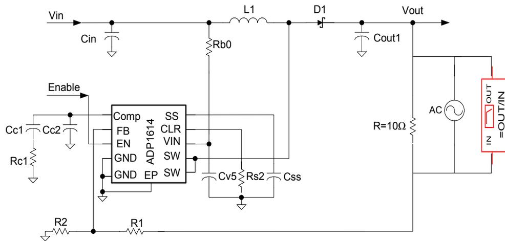
Figure 5.2 Boost converter connected with Frequency Response Analyzer
