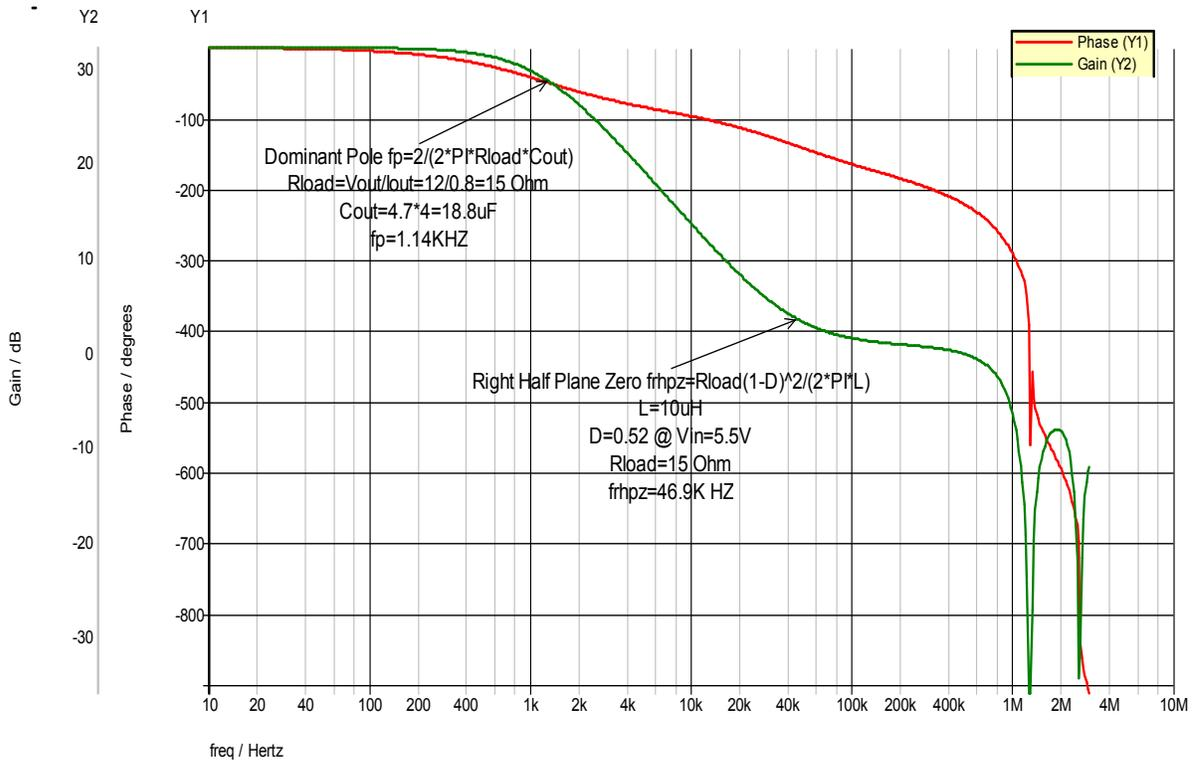
Figure 3.3 Bode Plot of Inner Current loop for CMC Boost Converter
