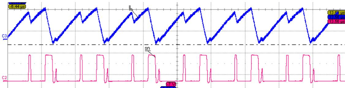
*Figure 2.11 Sub harmonic oscillation waveform in Current Mode Control*
