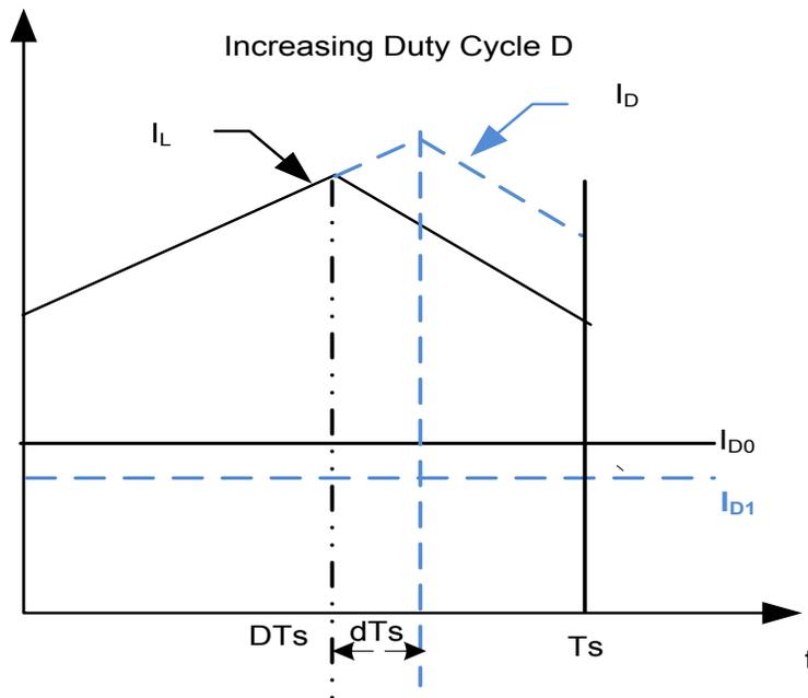
Figure 2.4 The current decreases in the output diode with increasing duty cycle  $D$  [9]
