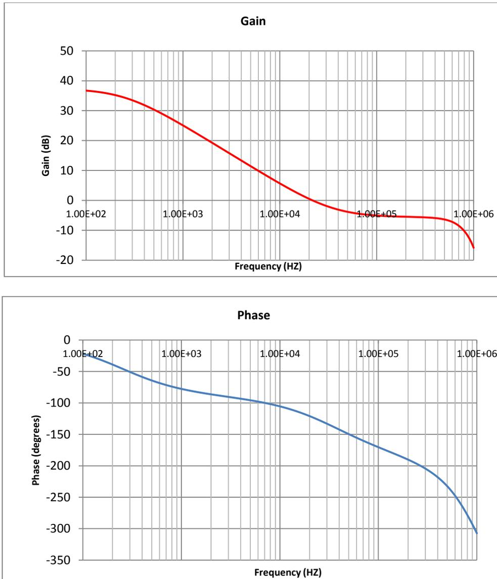
*Figure 2.5 RHPZ observed in the power stage from the output of the error amplifier (COMP pin) to the output*
