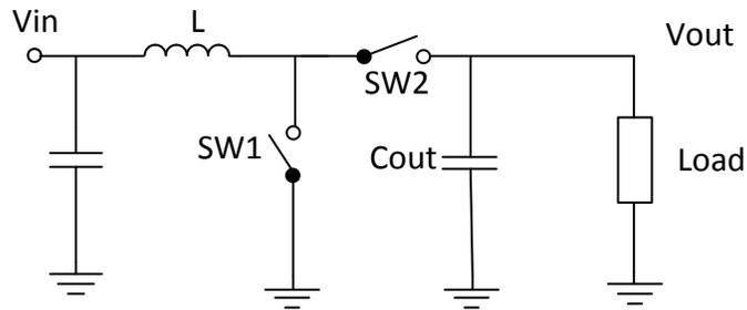
*Figure 1.1 Basic boost converter topology*
