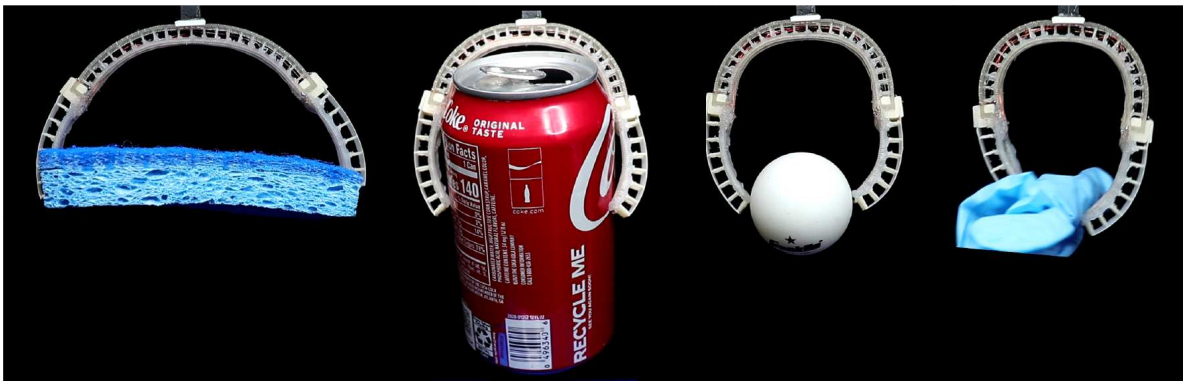
Figure 6.12: The objects that the adaptive gripper can pinch by morphing the base, i.e., a sponge, a Coke can, a pingpong ball, and a glove.
