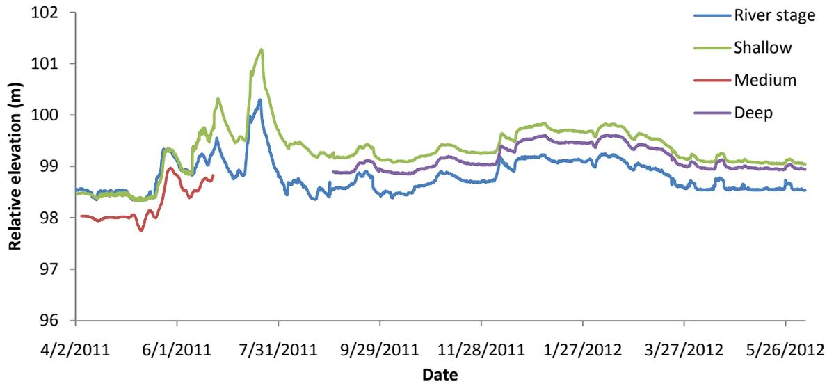
**Figure 11:** Pressure transducer data from shallow, medium, and deep piezometers for cross section 3. Water table elevations were compared to the surface elevation values of the South Platte River. Measurements from the medium piezometer were taken on an hourly basis from May 3<sup>rd</sup> to June 22<sup>nd</sup>, 2011, and from April 2<sup>nd</sup>, 2011 to June 6<sup>th</sup>, 2012 for the shallow and deep piezometers.
