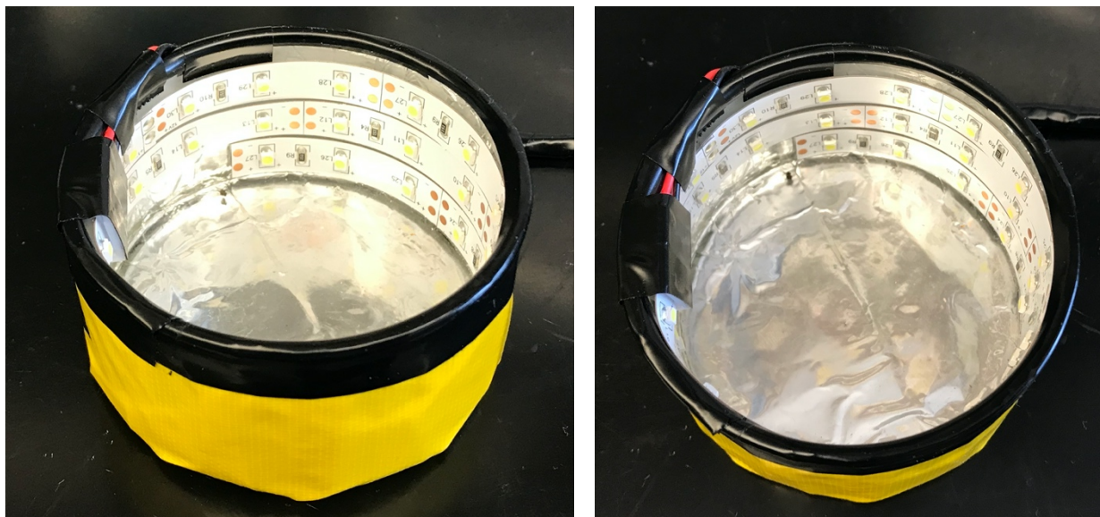
Figure 4.10. Photographs of the LED wells constructed with more light strips. These reactors were built by wrapping an 80 mm x 40 mm recrystallization dish with aluminum foil and wrapping uncoated white LED strips (15 LED segments) around the inside of the disk. The photographs provide a side view (left) and top view (right).
