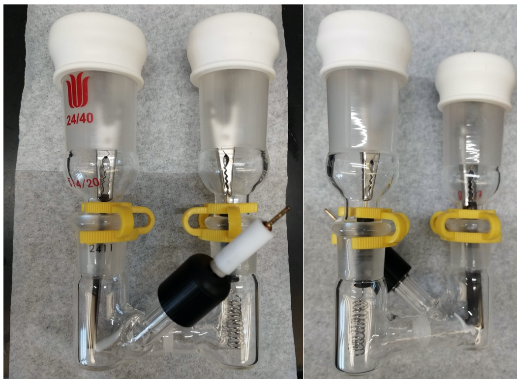
Figure 4.6. Photographs of the U-cell used in this work. (Left) Front side of the cell, showing the working electrode compartment on the left side, with a glassy carbon working electrode and reference electrode inserted in the side-arm. In the center, an extra-fine glass frit acts as a separator to prevent reaction solution from contacting the counter electrode, which is displayed in the right-side compartment. (Right) View of the U-cell from the back-side.
