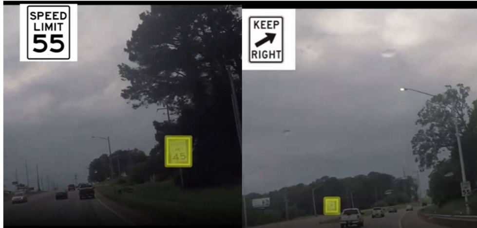
Figure 14. Sample TSR Errors Incorrect Identification (Left) and Missed Detection (Right)
