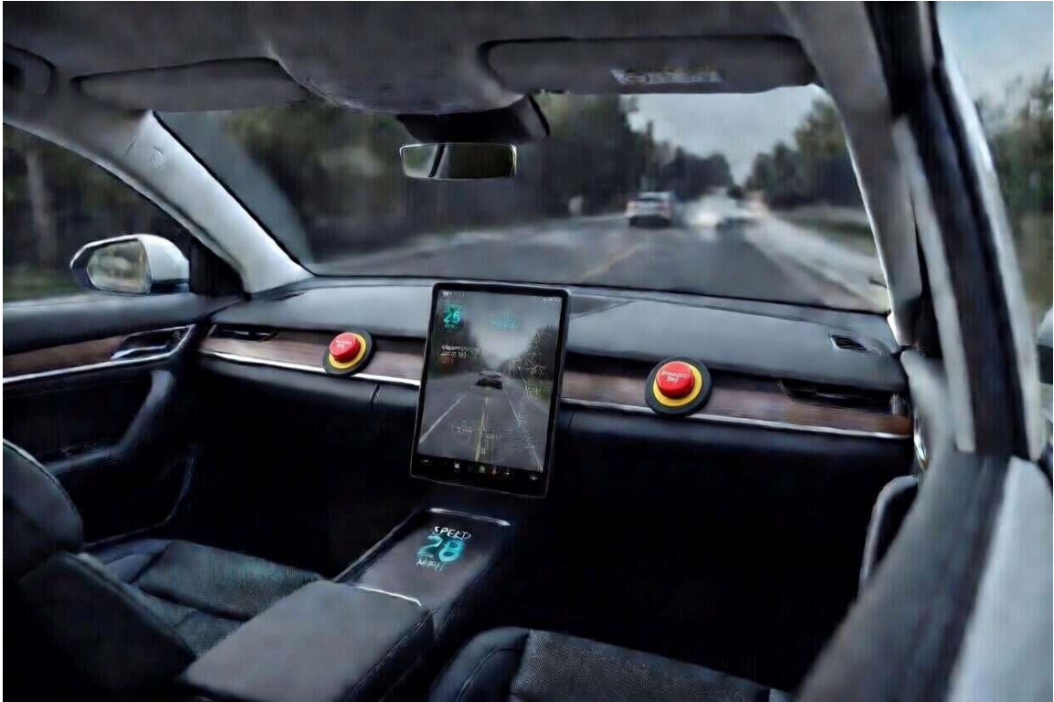
Figure 43. AI Generated SDV Center Console Display, Front Seat, Physical E-Stop Only
