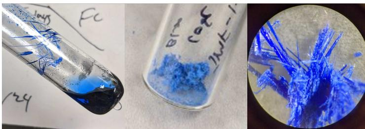
**Figure 4.1:** Picture of the completed reaction in sealed tube (left) with the blue material on the top of cobalt selenide powder. The product after solidifying and being ground (middle) and the crystals scraped from the side of the tube (right).
