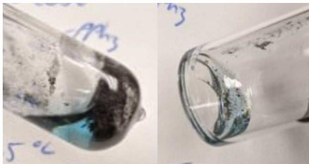
**Figure 4.11:** Sealed ampoule containing the cobalt-triphenylphosphine reactions (left) and the blue material from this reaction after being removed from the ampoule (right).
