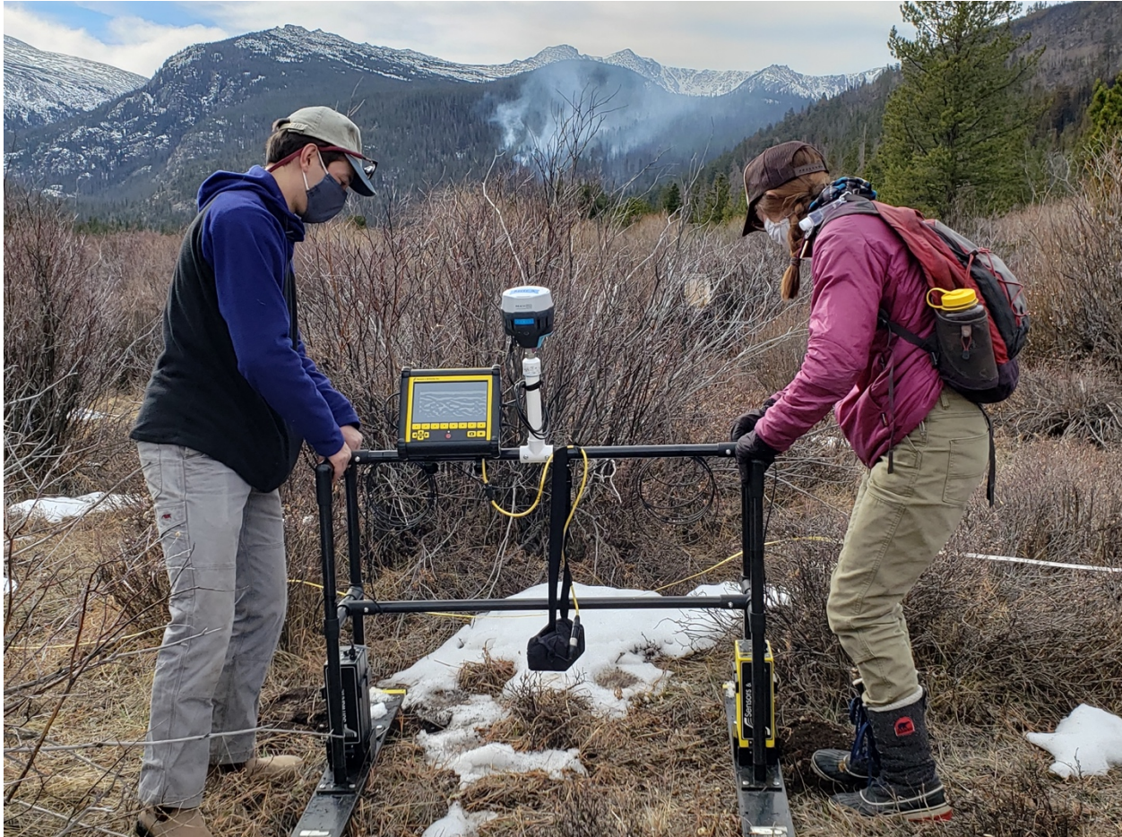
Figure 5: Sensors and Software PulseEKKO GPR system configured to collect a common offset transect (photo courtesy of M. Ronayne)
