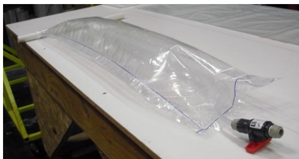
Figure 29. Photo of the CO 2 collection bag for the Equilibrium Study inflated. This photo shows the toothpaste tube design of the bag.
