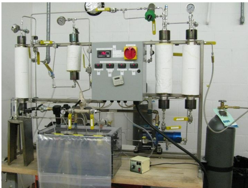
Figure 33. Photo of the apparatus for the Flow Study. The reduction of tubing between the storage tank and back pressure regulator is very present in this photo. Also the polycarbonate box had to be reversed, so a plastic curtain was added for safety.
