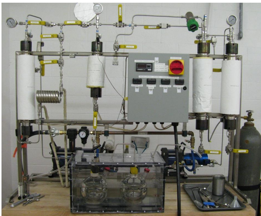
Figure 28. Photo of the apparatus for the Equilibrium Study. This configuration had some tubing removed and the addition of the needle valve and polycarbonate box assembly.
