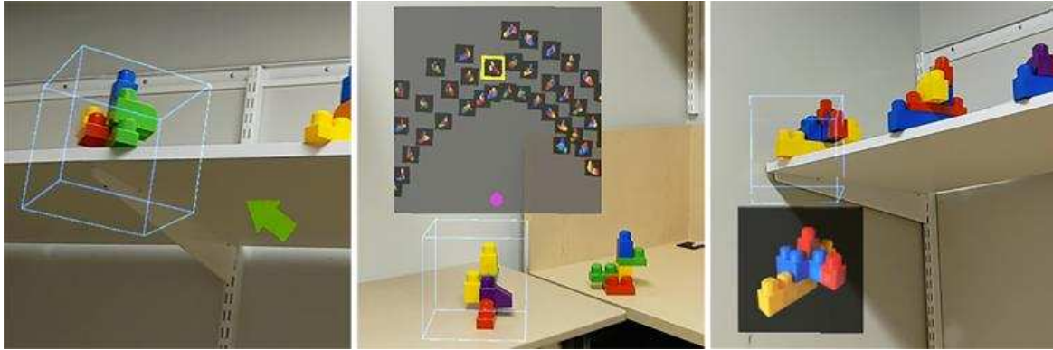
Figure 1. An illustration of an arrow cue (left) that points directly to the target independent of head movement, a minimap cue (middle) that shows a top-down perspective of the search scene and highlights the target, and an icon cue (right) that continuously displays an image of the target on the HMD display, respectively.
