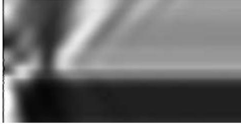
*Figure 2.12 Intensity illustration of Z axis Look Up Table (ZLUT). Horizontal pixel lines illustrate radial intensity distribution of a single bead at multiple Z positions. The focal plane is when the bead intensity changes from light to dark.*
