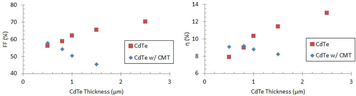
Figure 48: FF and Efficiency ( $\eta$ ) of CdS/CdTe cells at various CdTe thicknesses; with (Blue Diamonds) and without (Red Squares) a 1.75 eV CMT film
