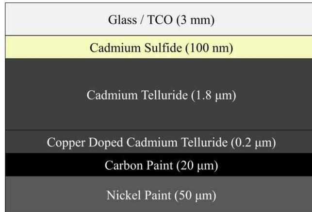
Figure 17: A diagram depicting the various layers that comprise the baseline cell structure of a typical CdS/CdTe cell manufactured in the single vacuum CSS chamber.
