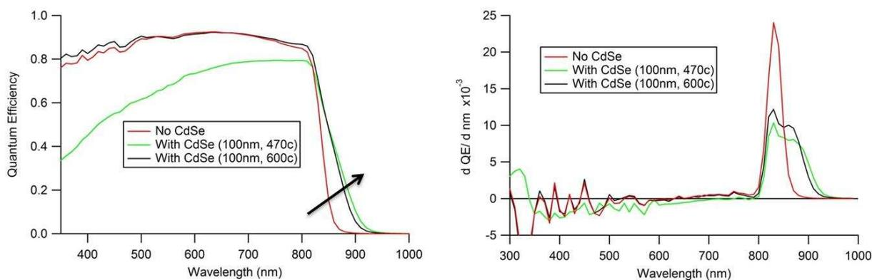
Figure 77: QE and dQE/dnm of CdSe buffered cells
