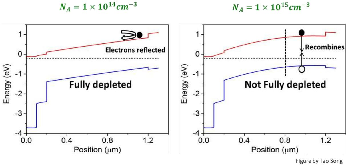
Figure 40: Depleted vs Not Depleted CdTe with Type A CMT ER
