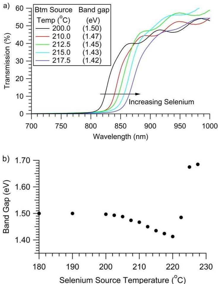
Figure 79: a) Optical transmission of CdSeTe films at various selenium bottom source temperatures b) Tauc-plot-calculated band gaps vs. selenium source temperatures. As the selenium source temperature is increased, the selenium vapor flux is increased and the CdSeTe band gap first decreases, than rises sharply.
