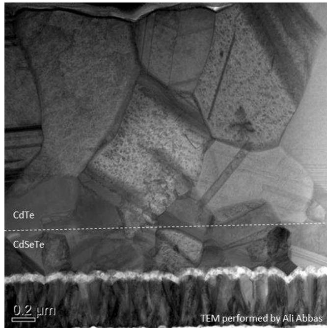
Figure 87 Cross section TEM of a 400 nm 1.45 eV CdSeTe/CdTe device using standard process conditions described in Section 2. A dashed white line represents the approximate CdSeTe/CdTe interface.
