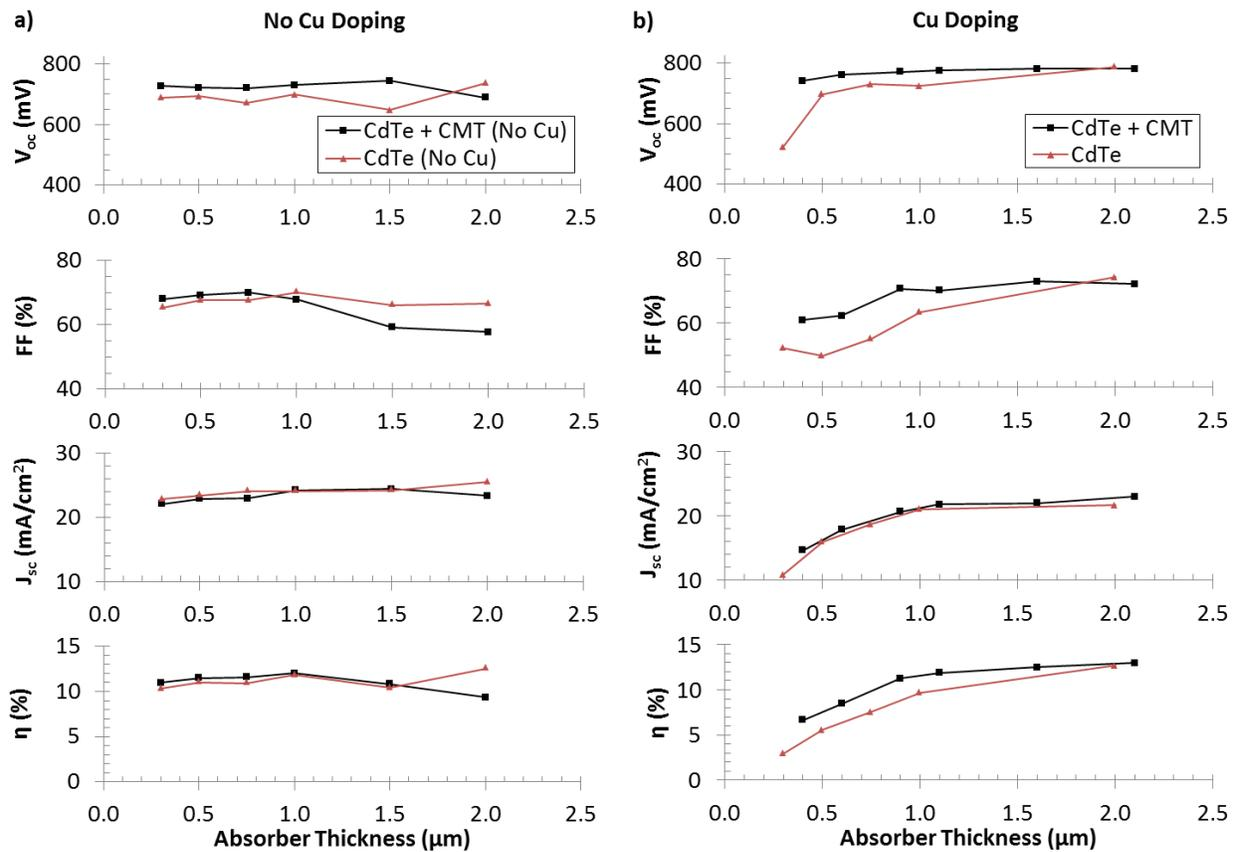
Figure 63: JV parameters of a CdTe/CMT ER structure with CdTe cap and Tellurium back contact at various CdTe thicknesses, with and without copper. Reference cells have identical structure but with CMT removed.
