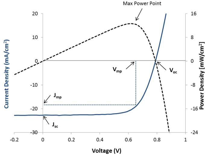
Figure 9: J-V curve of a CdTe cell with overlaid resulting power density, parameters  $V_{oc}$ ,  $J_{sc}$ ,  $V_{mp}$ ,  $J_{mp}$  are identified
