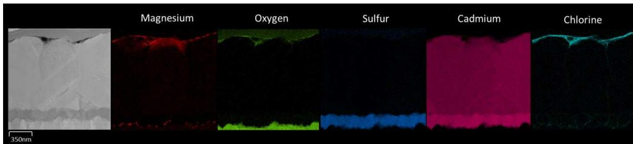
Figure 56: Cross Section TEM and EDX of CdS/CdTe/CMT stack passivated with CdCl<sub>2</sub>
