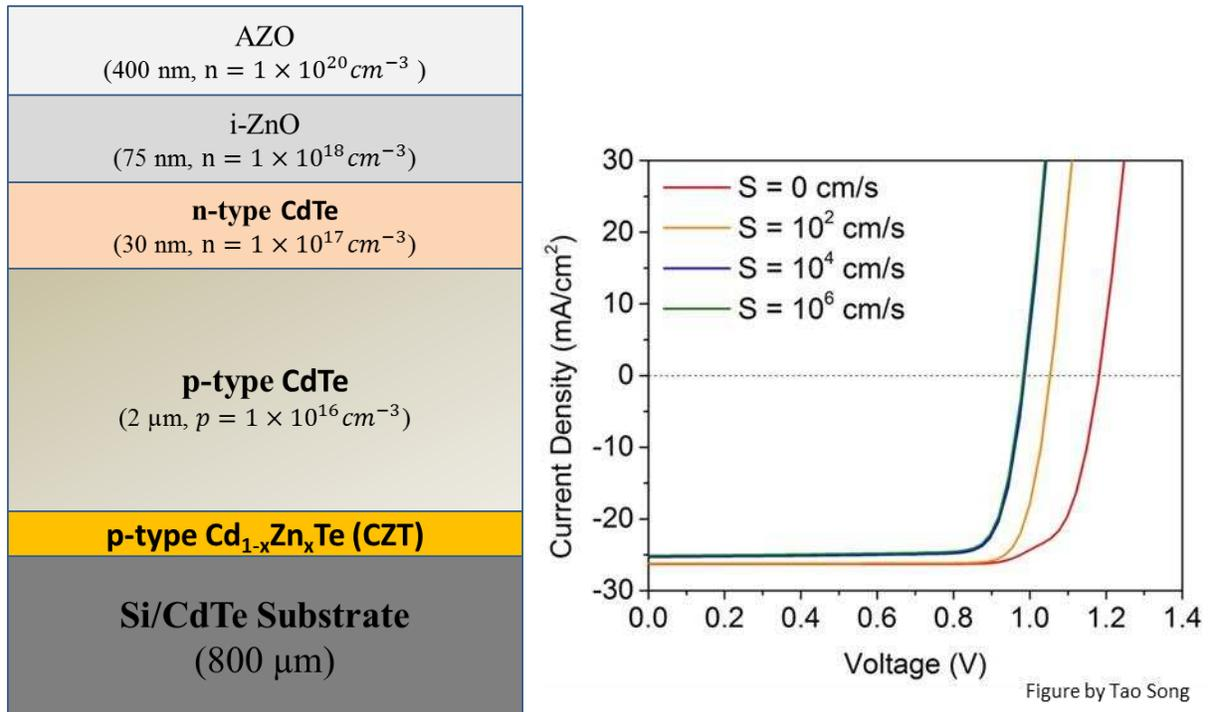
Figure 68: a) Structural diagram of ER Cell b) Modeled JV performance as a function of varying ER/CdTe IRV.
