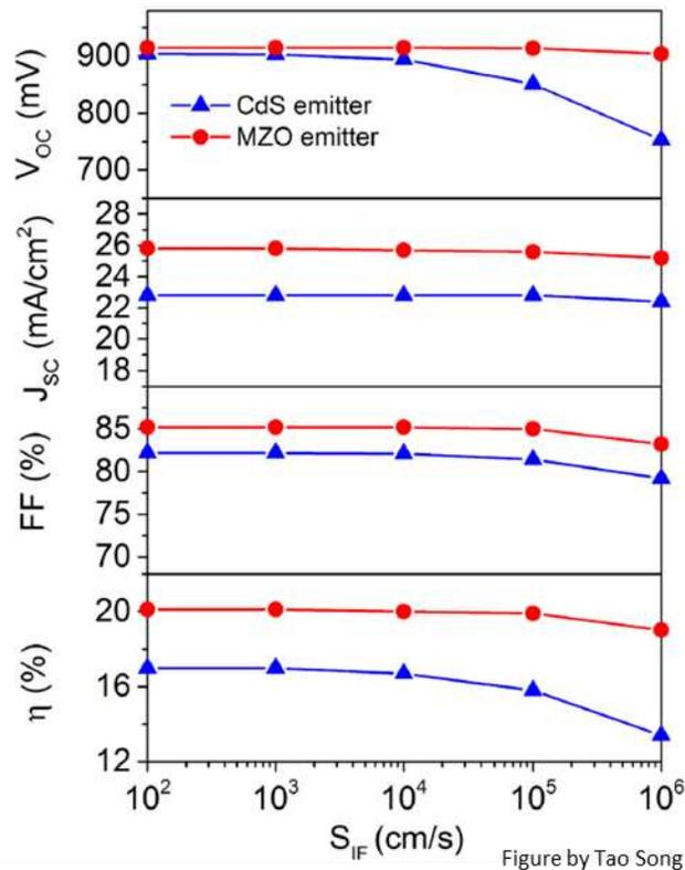
Figure 69: Calculated performance parameters as a function of interface recombination velocity with two practical emitters: CdS ( $E_g=2.4 \text{ eV}$ ,  $\Delta E_c = -0.1 \text{ eV}$ ) and MZO ( $E_g=3.7 \text{ eV}$ ,  $\Delta E_c = +0.2 \text{ eV}$ ). Figure 69 is Figure 10 from reference (103).
