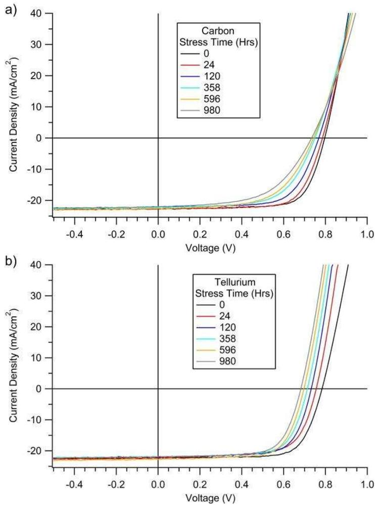
Figure 35: Accelerated Life Testing of CdS/CdTe cell with a) carbon and b) tellurium back contacts (with copper doping).
