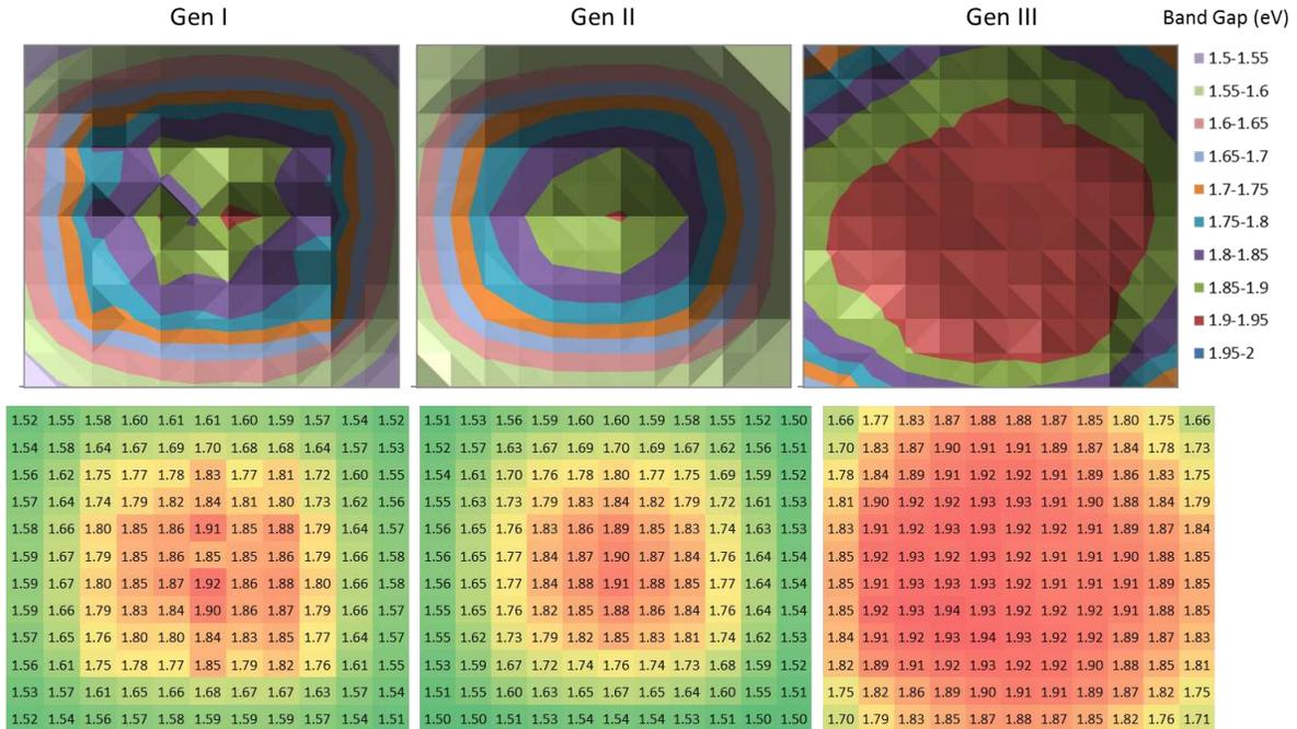
Figure 42: Co-Sublimation Source Generation I, II, and III showing band gap uniformity
