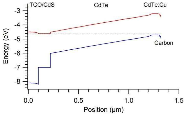
Figure 32: Band diagram of a CdS/CdTe cell with a carbon back contact, showing the formation of a VBO with the low work function back contact.
