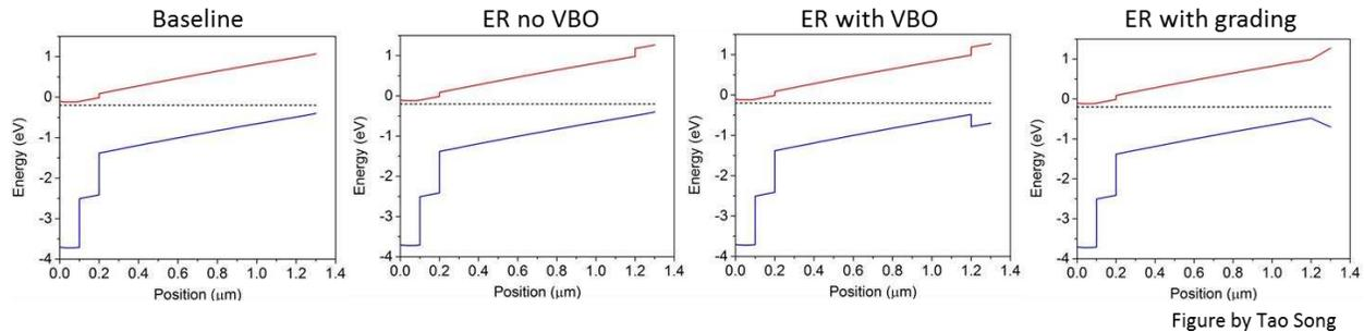
Figure 38: CMT Band diagrams a) Baseline, b) ER no VBO, c) ER with 0.3eV VBO, ER with graded 0.3eV VBO (82)
