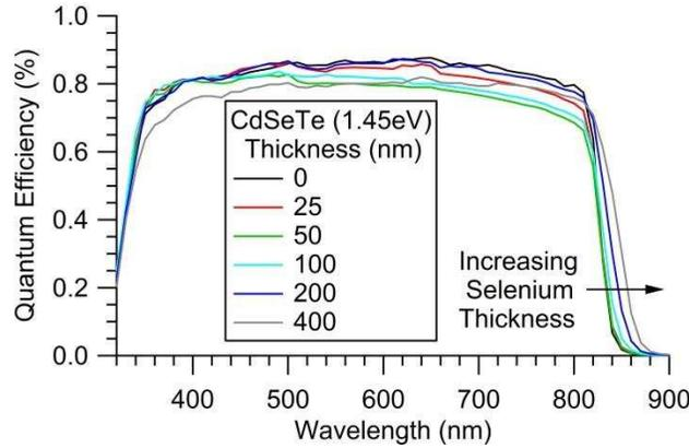
Figure 91: QE of 1.45eV CdSeTe/CdTe cells at various CdSeTe thicknesses. Greater photon collection above 840 nm is seen with increasing CdSeTe thickness.
