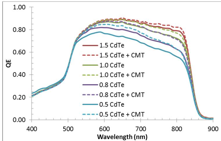
Figure 46: Quantum efficiency at various CdTe thicknesses with and without a 1.75 eV CMT layer
