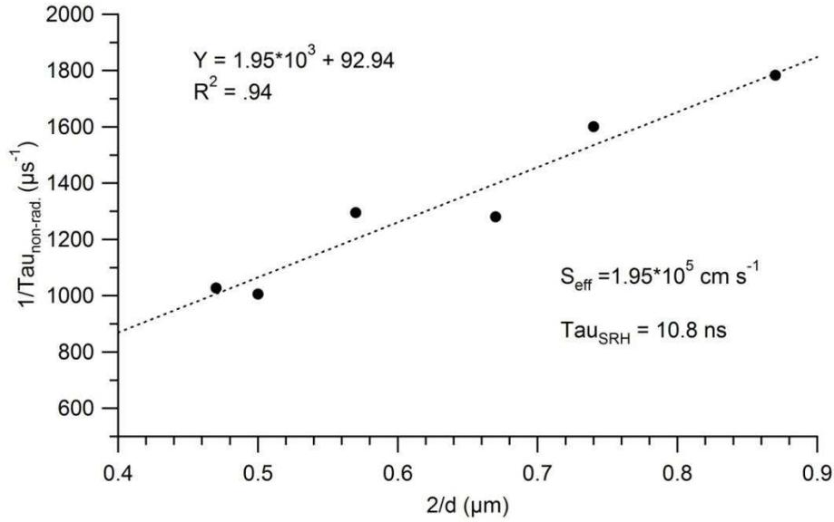
Figure 67: Inverse of the non-radiative lifetime vs  $2/d$  (Bulk CdTe absorber thickness). A linear fit is used to approximate the interface recombination and bulk SRH lifetime.
