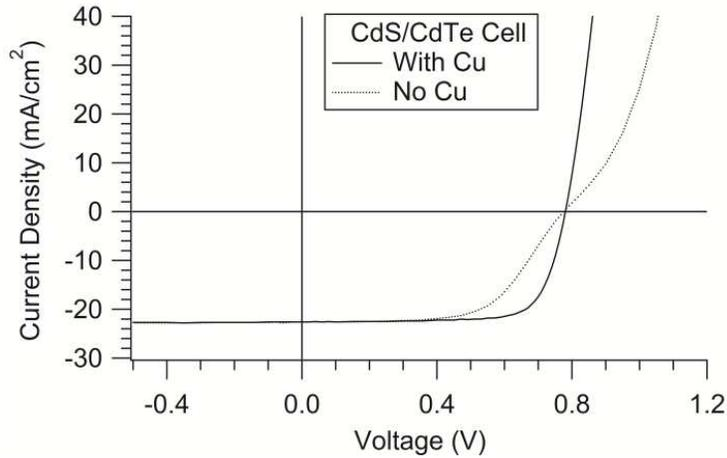
Figure 22: Current density versus voltage curves of a baseline CdS/CdTe cells.
