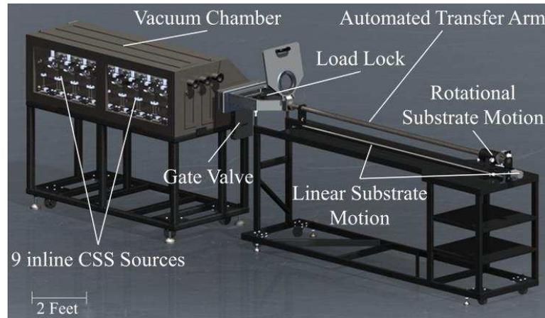
Figure 18: A diagram of the Single Vacuum Closed Space Sublimation Chamber with various key components being identified.
