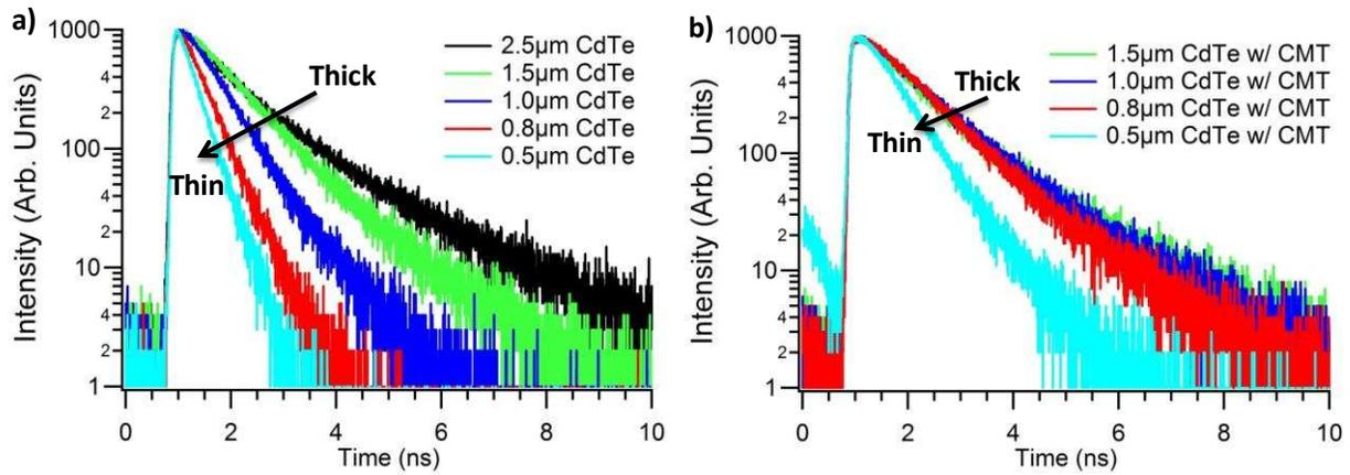
Figure 49: TRPL from a) CdS/CdTe and b) CdS/CdTe/CMT cells as a function of the CdTe absorber thickness
