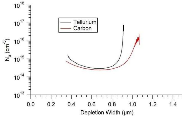
Figure 29: C-V of a CdS/CdTe cells with tellurium vs carbon back contacts
