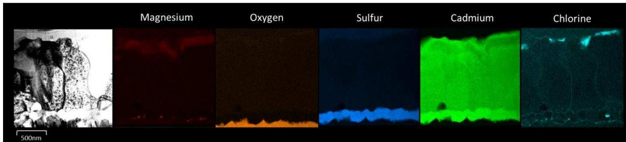
Figure 58: TEM and EDX of CdS/CdTe/CMTe/CdTe Cap stack passivated with CdCl<sub>2</sub>
