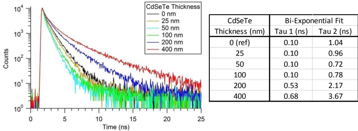
Figure 92: TRPL of 1.45eV CdSeTe/CdTe cells at various CdSeTe thicknesses. Improvements in lifetime can be seen as the CdSeTe thickness is increased.
