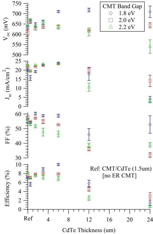
Figure 65: JV of CMT Double-Hetero-Structures at 1.8, 2.0, 2.2 eV band gaps and various thicknesses.
