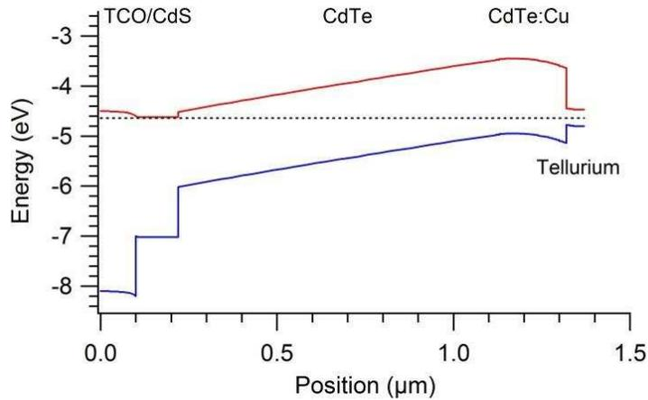
Figure 34: Band diagram of a CdS/CdTe cells with a tellurium back contact with copper doping, the increased carrier concentration at the back reduces the voltage loss.
