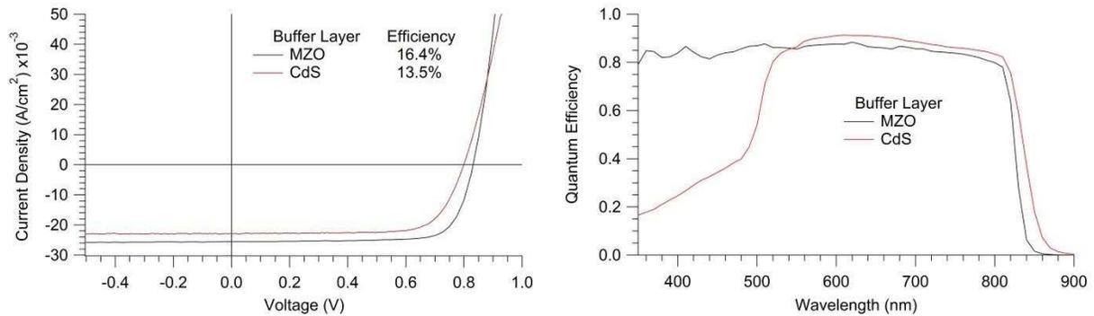
Figure 74: QE of a CdS/CdTe and MZO/CdTe cell
