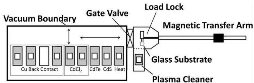
Figure 20: A diagram depicting the 2 dimensional motion of the end effector and substrate through the deposition chamber.
