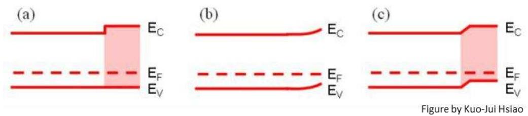
Figure 11: Band diagrams of the three proposed ER structures: a) expanded band gap layer, b) reversed back barrier, and c) heavily doped back surface (27)
