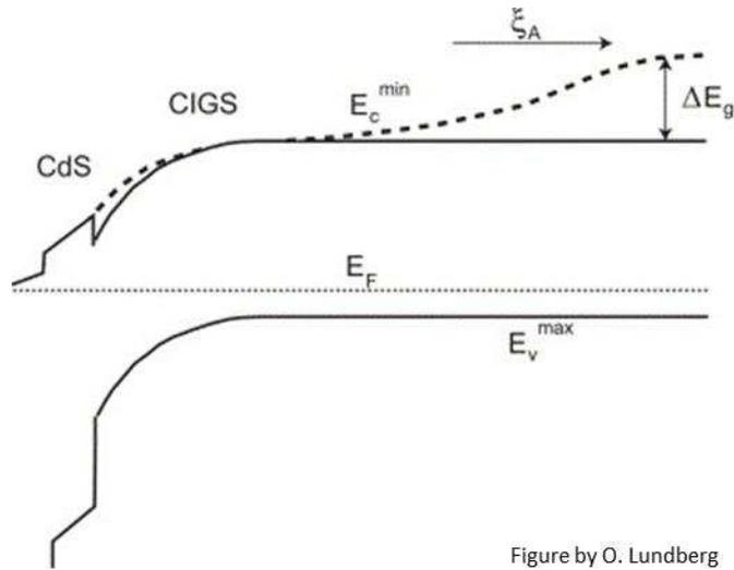
Figure 15: Band diagram of a CIGS cell, dotted line shows the change in the CBO as the Ga content is increased (35)
