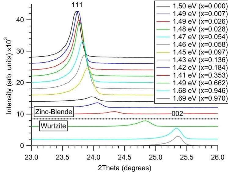
Figure 84: 111 XRD peak with varying selenium concentration. The 111 peak shifts to the right as the selenium concentration is increased, then disappears at the structural transition.
