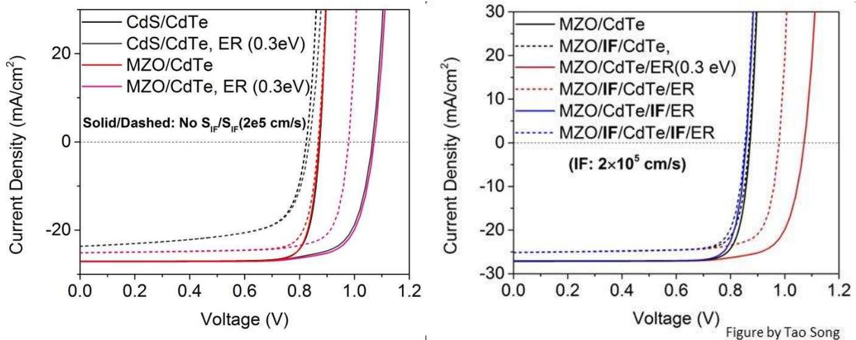
Figure 70: Modeling predicting the effects of  $10^5 \text{ cm s}^{-1}$  IRV at various key interfaces with CdS and MZO window layers. No performance improvement is predicted with  $10^5 \text{ cm s}^{-1}$  IRV at the CdTe/CMT interface.
