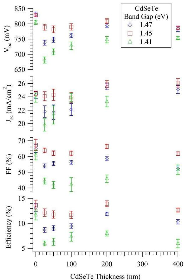
Figure 89: JV performance parameters of MZO/CdSeTe/CdTe devices with the CdSeTe layer at 1.47, 1.45, and 1.41 eV. The CdSeTe thickness is swept from 0 – 400nm. Average device values are used with a plus/minus one standard deviation error bar.  $J_{sc}$  at 1.41 eV and 400 nm is 15.4 mA/cm<sup>2</sup>.
