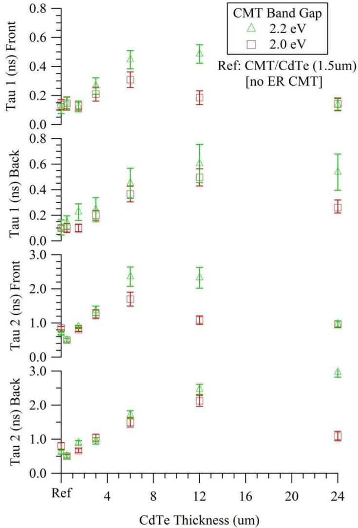
Figure 66: TRPL approximated Tau1 and Tau2 for 2.0 and 2.2 eV CMT DHT at various thicknesses.
