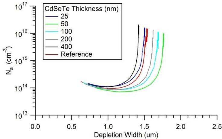
Figure 94: CV of 1.45eV CdSeTe/CdTe cells at various CdSeTe thicknesses.
