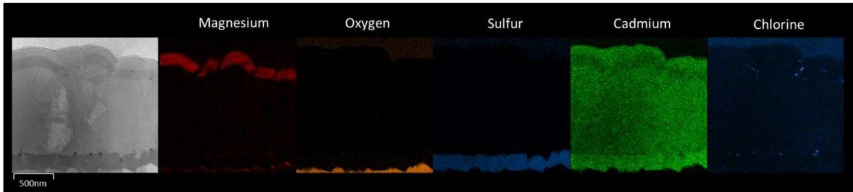
Figure 59: TEM and EDX of CdS/CdTe/CMT/CdTe Cap stack passivated with  $\text{MgCl}_2$
