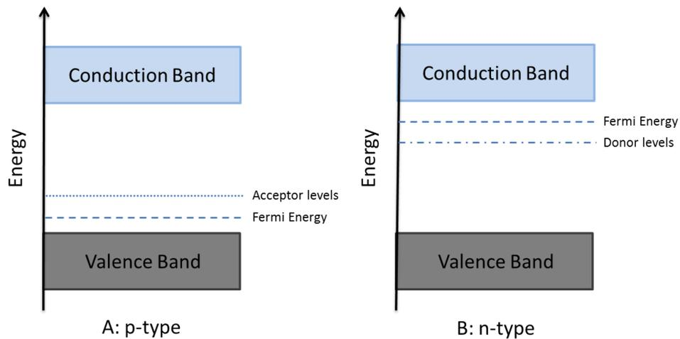
Figure 7: Position of Fermi energy a) p-type b) n-type semiconductors (25)
