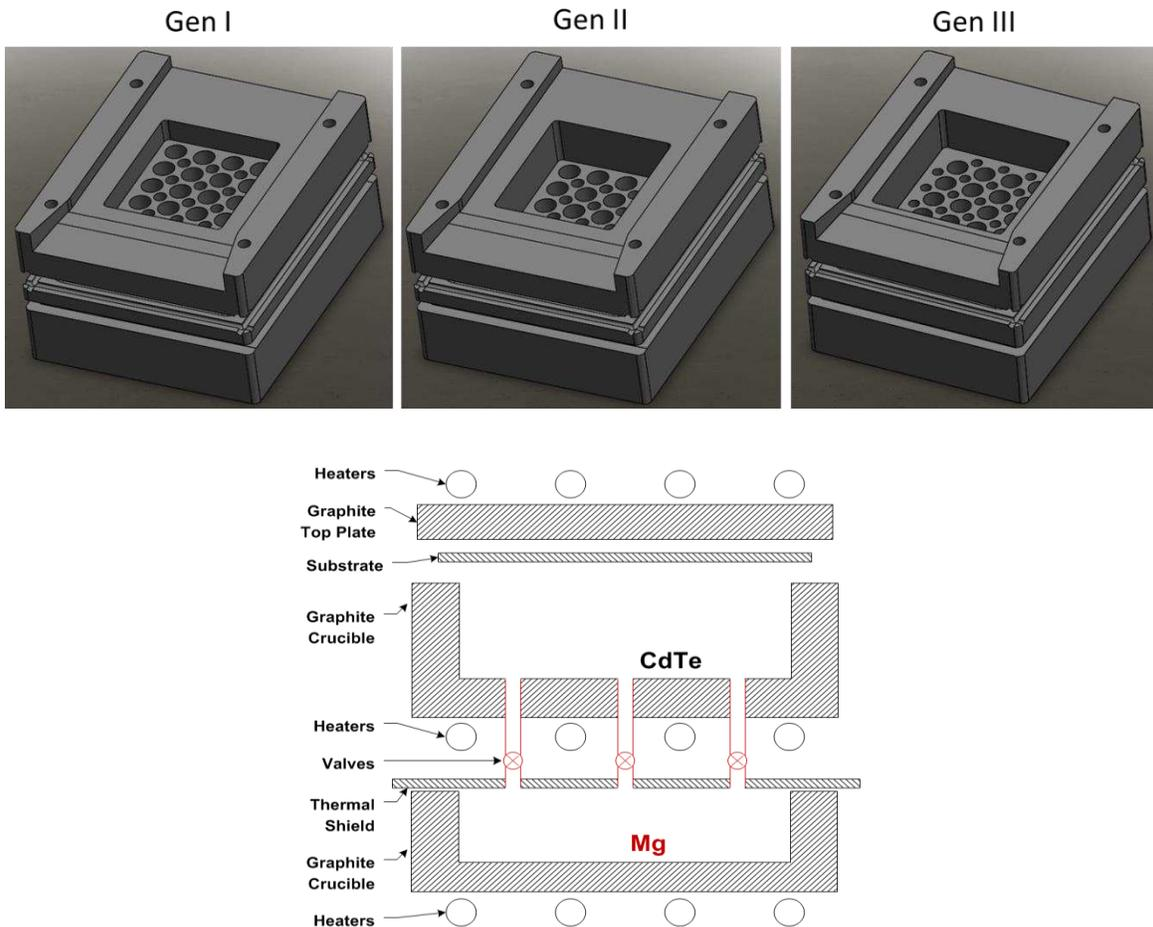
Figure 43: (top) CAD drawings of Generation I, II, and III of the CdTe Co-Sublimation Source (bottom) Schematic of Co-Sublimation Sources
