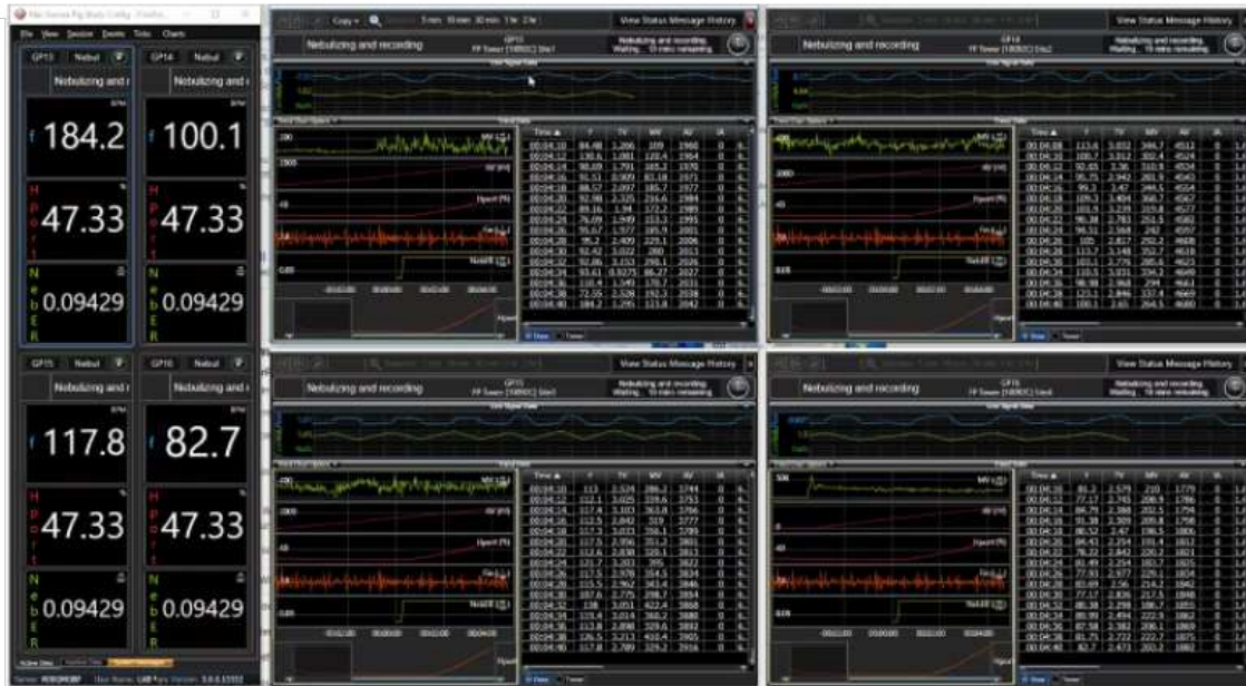
Supplemental figure S22. Particle size and parameters of Buxco inhalation tower. A) particle size distribution made by the small pore nebulizer as measured by the tower's particle size analyzer. Particles measuring an average of 1µm in diameter are the correct size for penetrating into the alveolar spaces. B) Control panel of tower during an exposure. Allows for monitoring of breaths per minute, chamber humidity, particle concentration, and accumulated inhalation volume of each animal.
