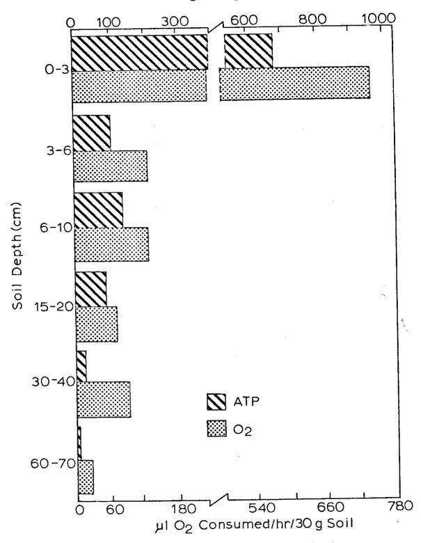
Fig. 16. Variation in ATP content and respiration rate (water + glucose amendment) with depth in irrigated soil (July sampling).
