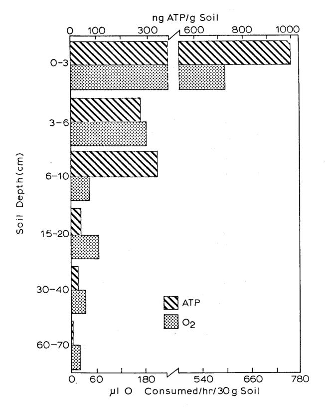
Fig. 17. Variation in ATP content and respiration rate (water + glucose amendment) with depth in non-irrigated soil (August sampling).
