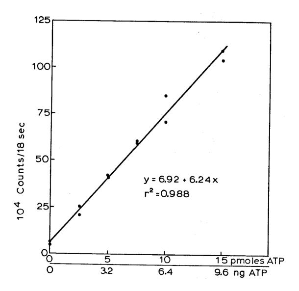
Relationship between light emission and ATP concentration with and without internal standard of bacterial extract containing ATP. Fig. 2.
