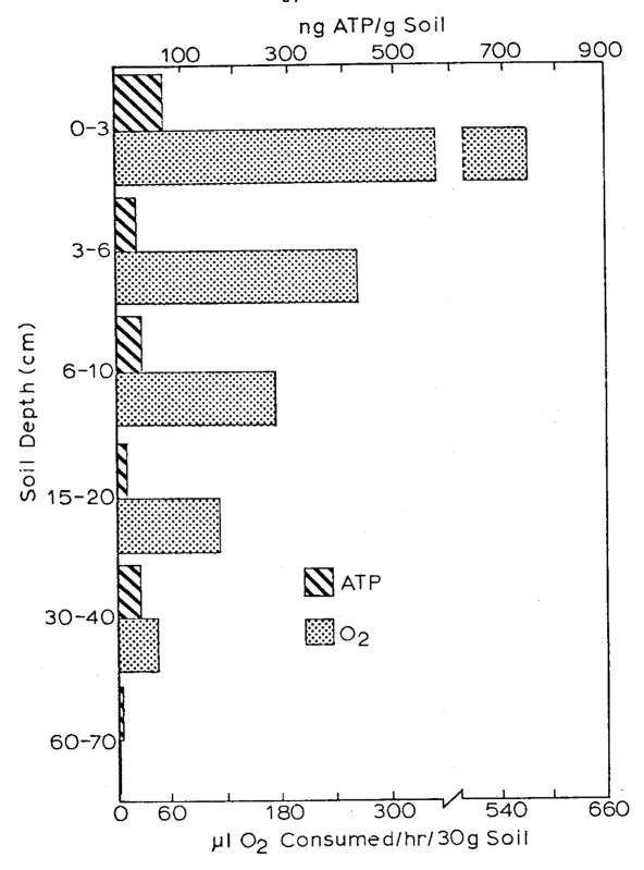
Fig. 18. Variation in ATP content and respiration rate (water + glucose amendment) with depth in non-irrigated soil (September sampling).
