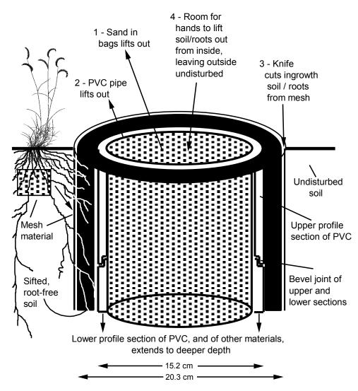
Six inch diameter PVC pipe is placed in the <u>middle</u> of larger 8 inch holes and filled with sand bags (use 1 inch doweling to space PVC in middle). This creates a one inch donut space width all around the cylinder. The donut space between the cylinder and the ingrowth cloth (the wire mesh material) is filled with root-free sifted soil from an adjacent area, and packed to a similar bulk density as outside soil using doweling. Roots are sampled the
