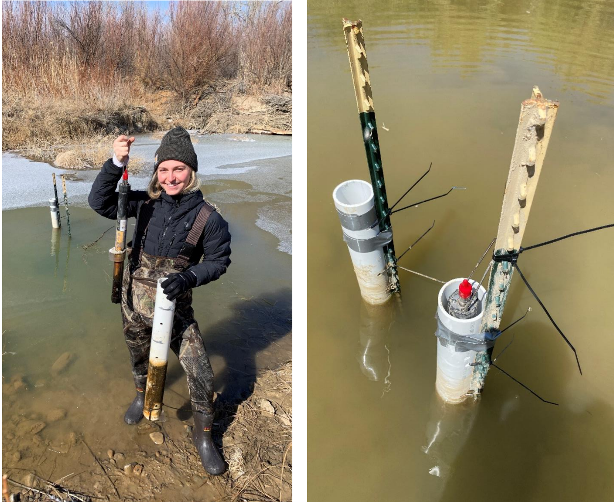
Figure 11. Images of the field site at PURLASCO. In the left image, the Aqua TROLL 600 is shown held, and in the right image, the two casings for the sensors are displayed with the Onset HOB0 logger hanging out of view in the left pipe and the Aqua TROLL 600 visible in the right pipe.
