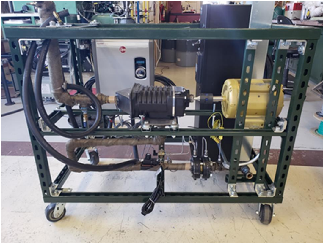
Figure C-6: Full EGR Test Cart System for CFR Engine
