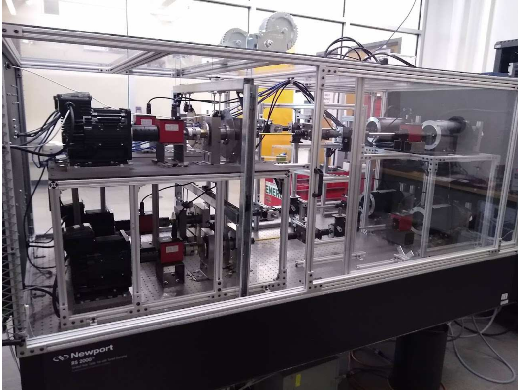
Figure 6.6: Test stand with four actuation lines.
